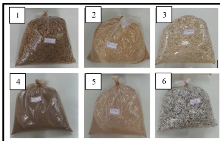
Figure 1. Samples: (1) rice husk, (2) pinus sawdust, (3) guapuruvu, (4) eucalyptus bark, (5) eucalyptus sawdust, (6) cotton linter
