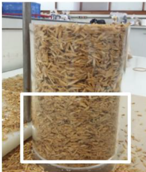
Figure 5. Container with rice husk sample (sample 1), highlighting the visually more compacted region due to the impacts suffered during the procedure
