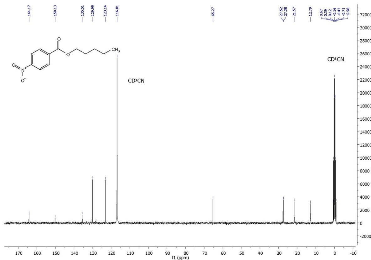
**Figure S20.**  $^{13}\text{C}$  NMR spectrum (75 MHz,  $\text{CD}_3\text{CN}$ ) of pentyl 4-nitrobenzoate.
