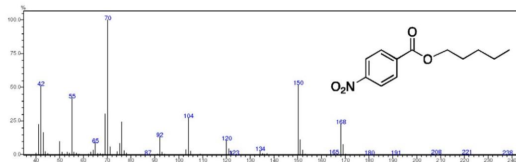
**Figure S21.** Mass spectrum (70 eV) of pentyl 4-nitrobenzoate.
