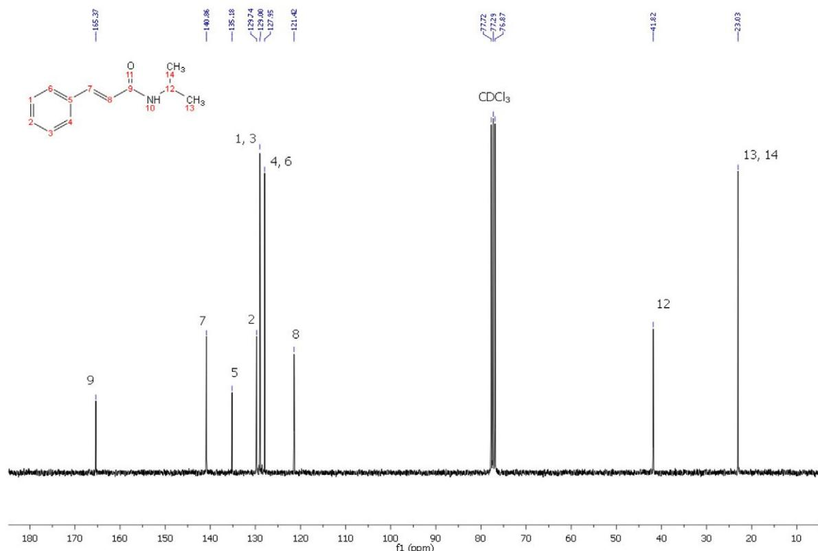
**Figure S41.** <sup>13</sup>C NMR spectrum (75 MHz, CDCl<sub>3</sub>) of *N*-isopropyl-cinnamamide.
