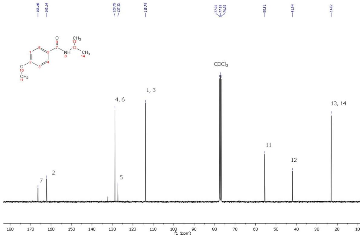
Figure S35.  $^{13}\text{C}$  NMR spectrum (75 MHz,  $\text{CDCl}_3$ ) of *N*-isopropyl-4-methoxybenzamide.
