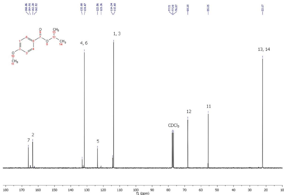
**Figure S8.**  $^{13}\text{C}$  NMR spectrum (75 MHz,  $\text{CDCl}_3$ ) of isopropyl 4-methoxybenzoate.
