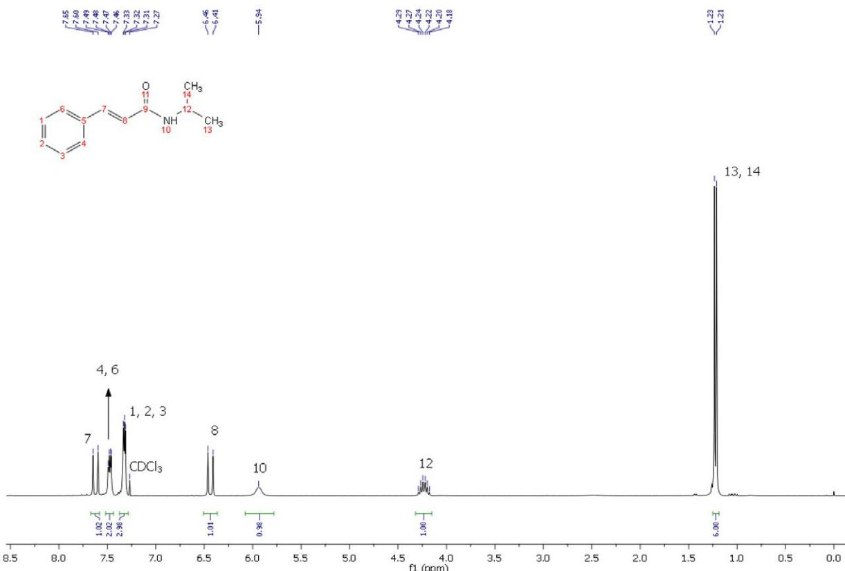
**Figure S40.** <sup>1</sup>H NMR spectrum (300 MHz, CDCl<sub>3</sub>) of *N*-isopropyl-cinnamamide.
