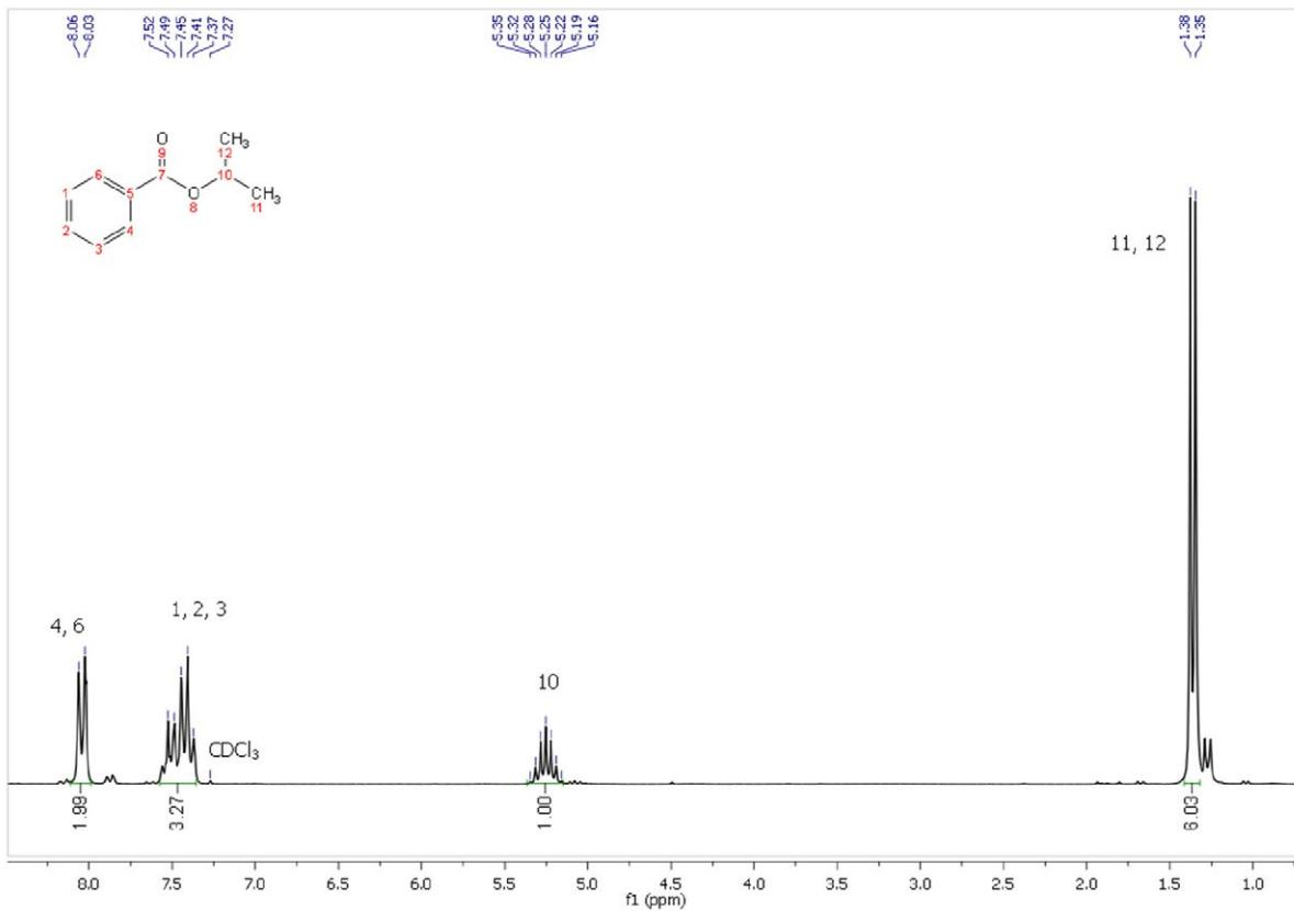
Figure S1. <sup>1</sup>H NMR spectrum (200 MHz, CDCl<sub>3</sub>) of isopropyl benzoate.
