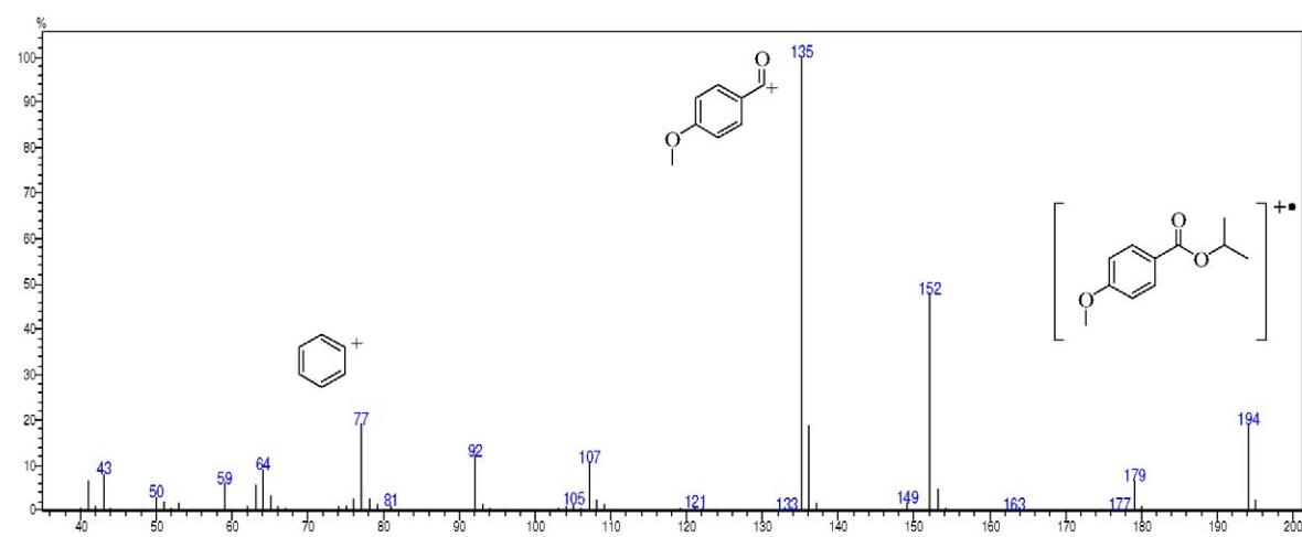
**Figure S9.** Mass spectrum (70 eV) of isopropyl 4-methoxybenzoate.
