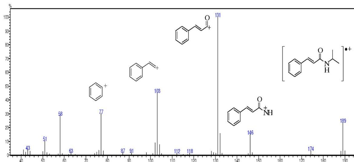
**Figure S42.** Mass spectrum (70 eV) of *N*-isopropyl-cinnamamide.
