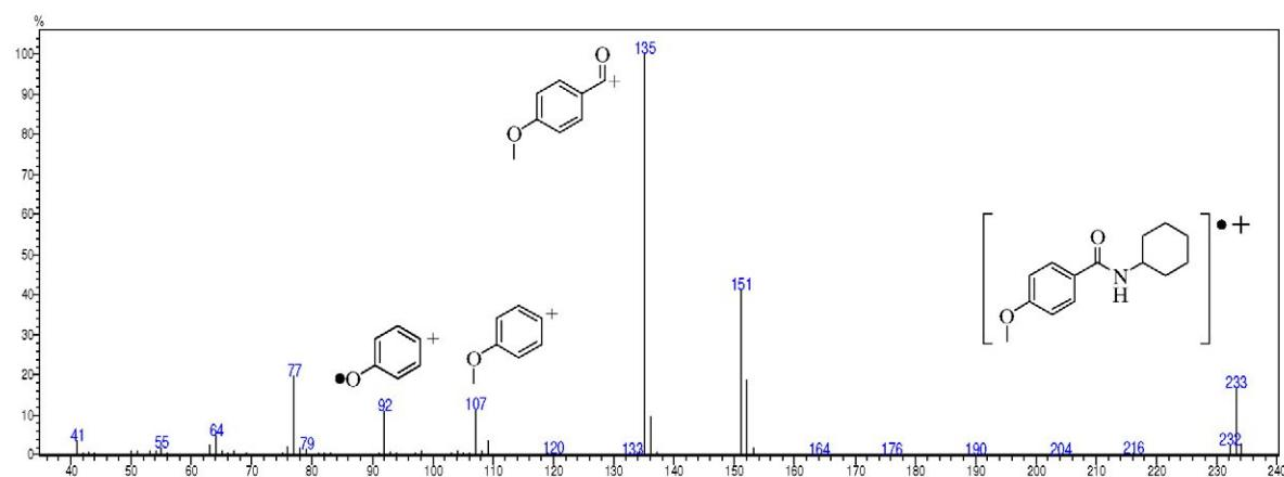
**Figure S33.** Mass spectrum (70 eV) of *N*-cyclohexyl-4-methoxybenzamide.
