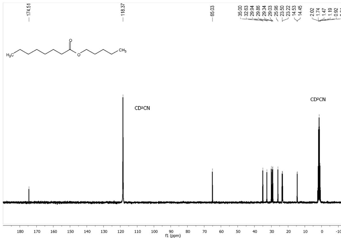
**Figure S23.**  $^{13}\text{C}$  NMR spectrum (75 MHz,  $\text{CD}_3\text{CN}$ ) of pentyl octanoate.
