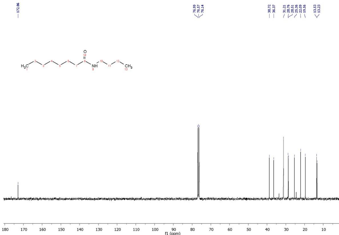
**Figure S50.**  $^{13}\text{C}$  NMR spectrum (75 MHz,  $\text{CDCl}_3$ ) of *N*-butyl-octanamide.
