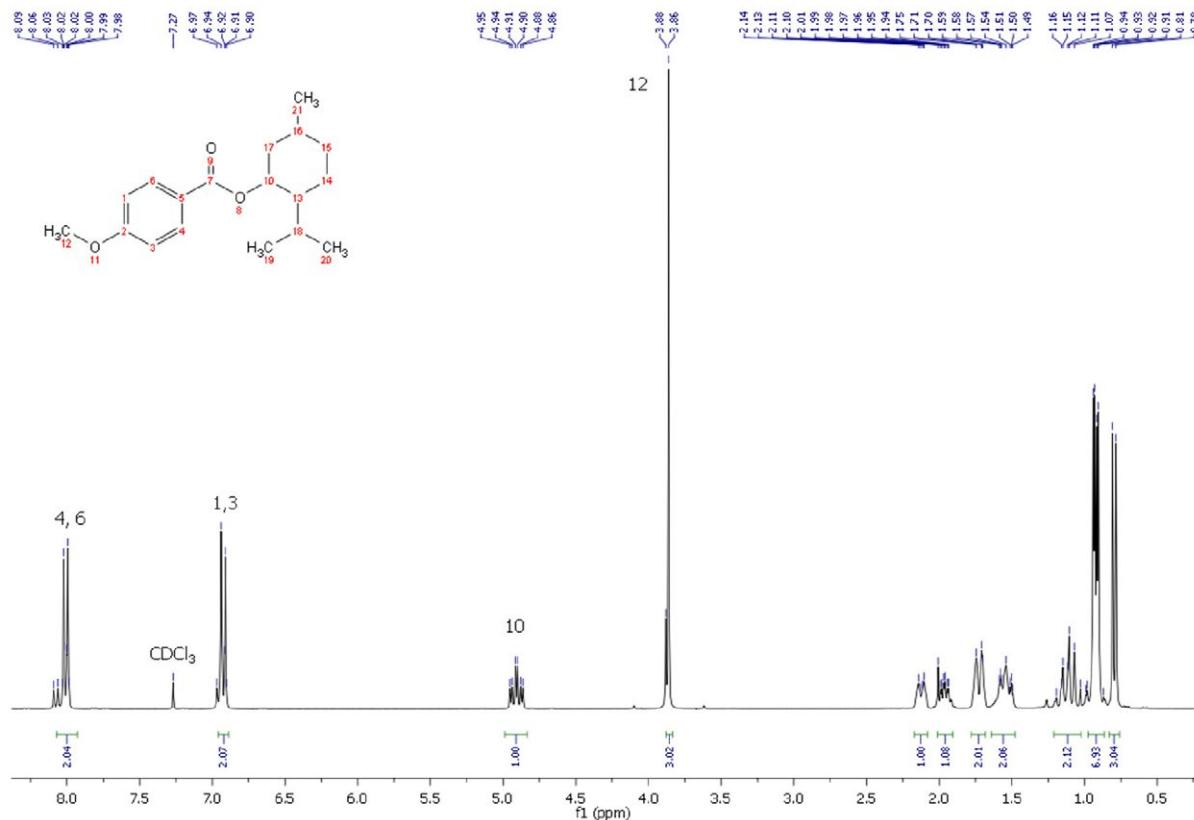
**Figure S10.** <sup>1</sup>H NMR spectrum (300 MHz, CDCl<sub>3</sub>) of methyl 4-methoxybenzoate.
