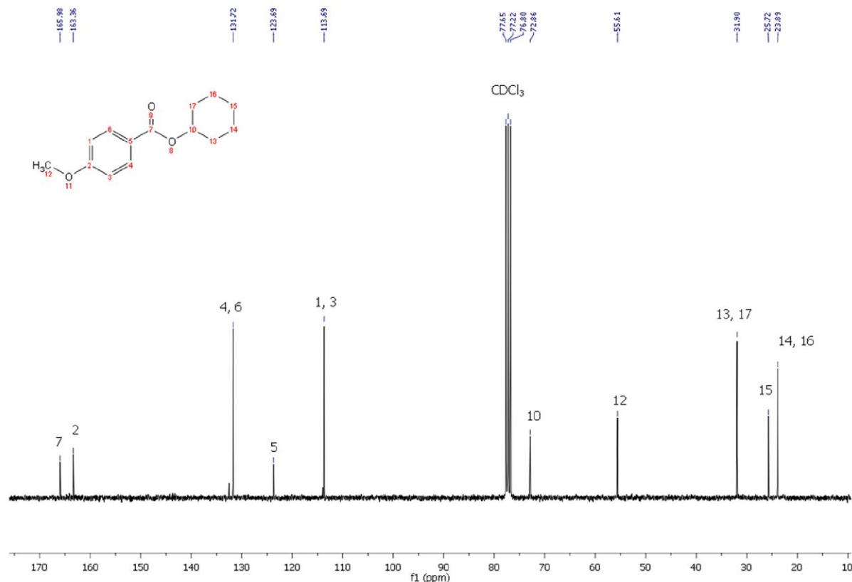
**Figure S14.**  $^{13}\text{C}$  NMR spectrum (75 MHz,  $\text{CDCl}_3$ ) of cyclohexyl 4-methoxybenzoate.
