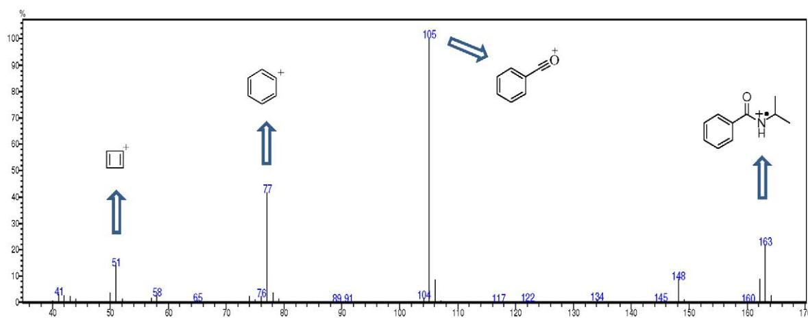
**Figure S27.** Mass spectrum (70 eV) of *N*-isopropyl-benzamide.
