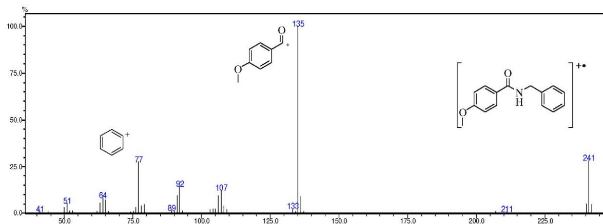
Figure S39. Mass spectrum (70 eV) of N-benzyl-4-methoxybenzamide.
