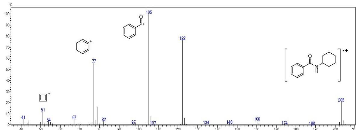
**Figure S30.** Mass spectrum (70 eV) of *N*-cyclohexyl-benzamide.
