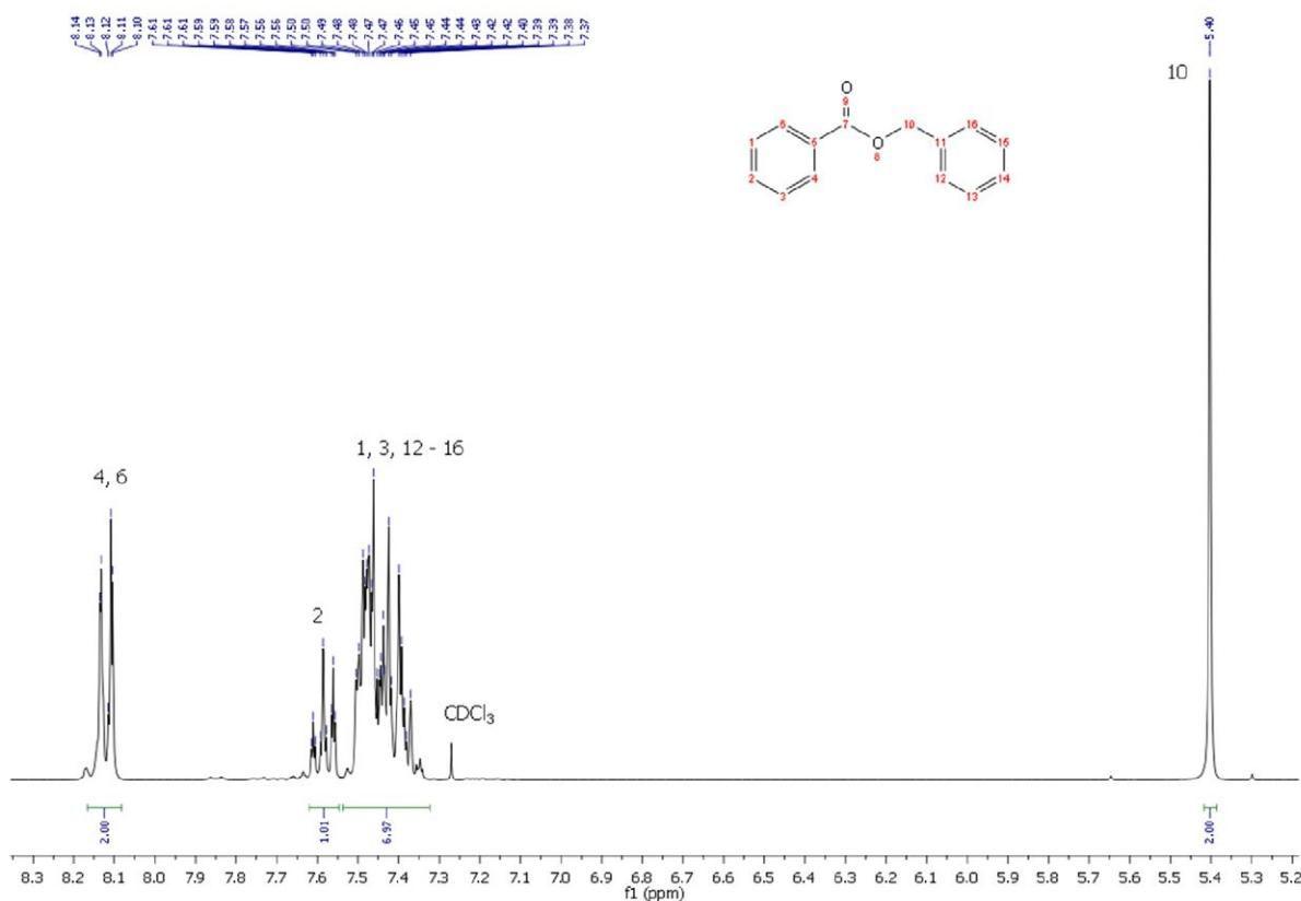
**Figure S4.** <sup>1</sup>H NMR spectrum (300 MHz, CDCl<sub>3</sub>) of benzyl benzoate.
