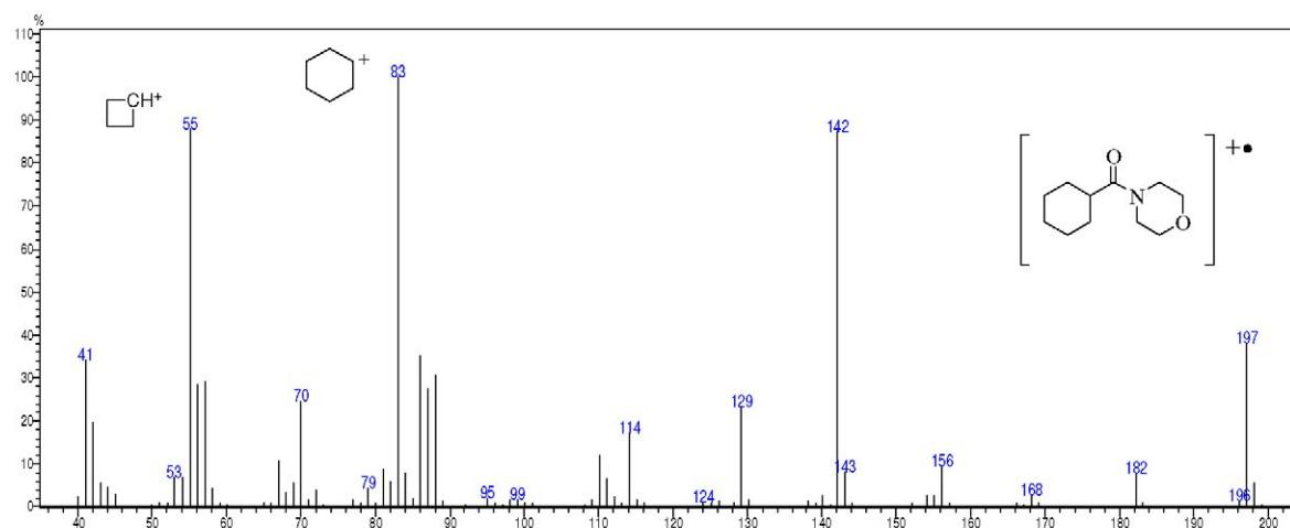
**Figure S45.** Mass spectrum (70 eV) of *N*-(cyclohexylcarbonyl)-morpholine.
