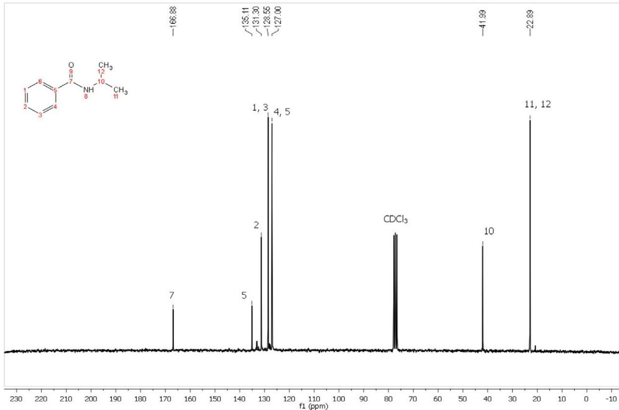
**Figure S26.** <sup>13</sup>C NMR spectrum (50 MHz, CDCl<sub>3</sub>) of *N*-isopropyl-benzamide.
