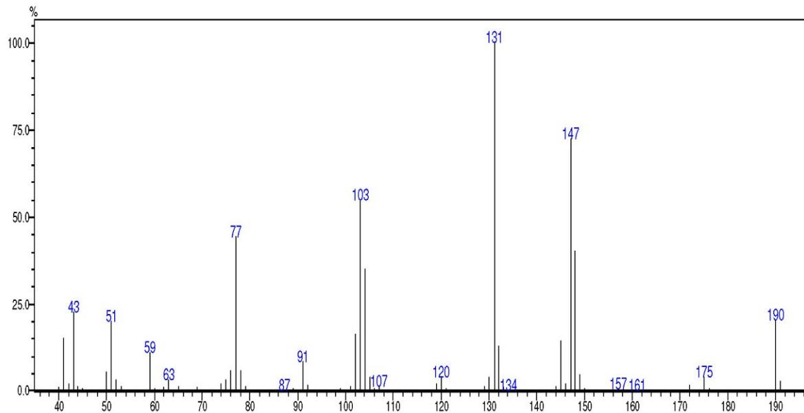
**Figure S18.** Mass spectrum (70 eV) of isopropyl cinnamate.
