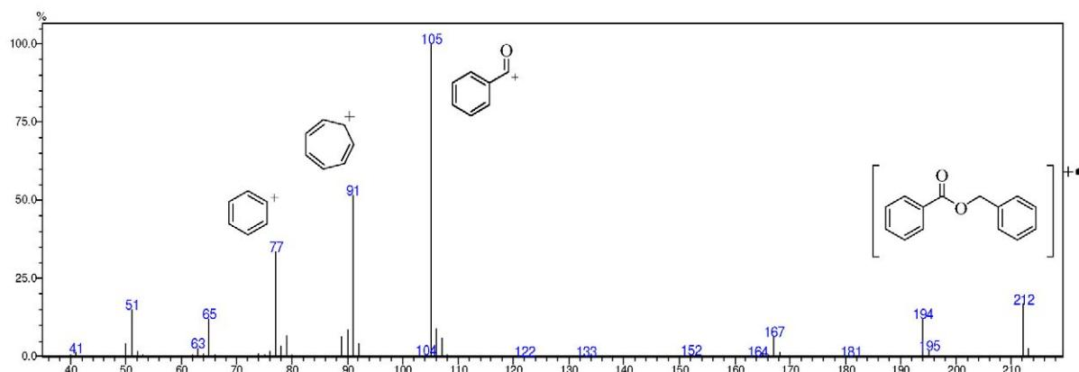
**Figure S6.** Mass spectrum (70 eV) of benzyl benzoate.
