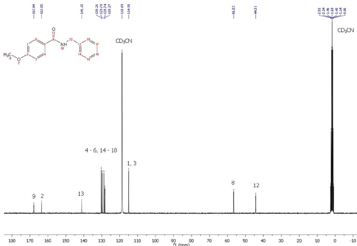
Figure S38. <sup>13</sup>C NMR spectrum (75 MHz, CD<sub>3</sub>CN) of N-benzyl-4-methoxybenzamide.
