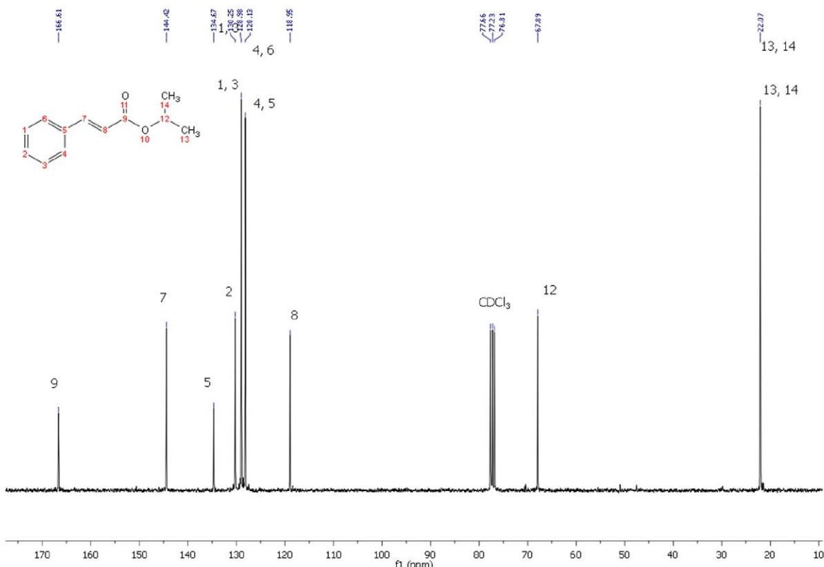
**Figure S17.** <sup>13</sup>C NMR spectrum (75 MHz, CDCl<sub>3</sub>) of isopropyl cinnamate.
