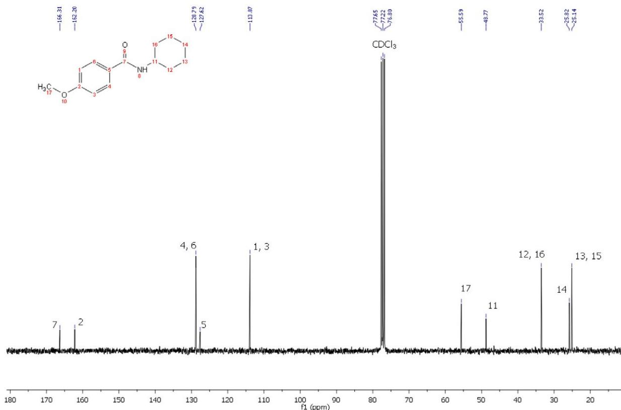
**Figure S32.**  $^{13}\text{C}$  NMR spectrum (75 MHz,  $\text{CDCl}_3$ ) of *N*-cyclohexyl-4-methoxybenzamide.
