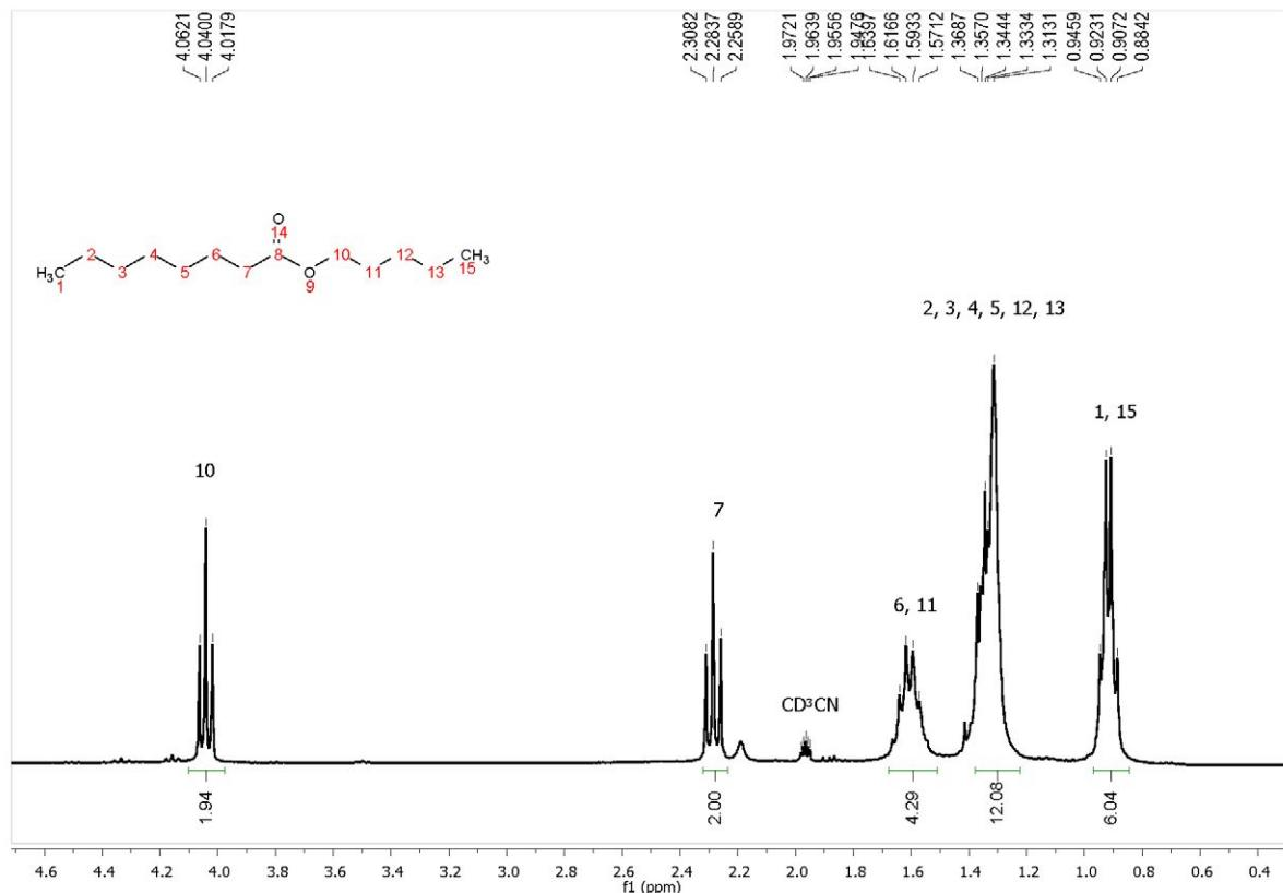
**Figure S22.**  $^1\text{H}$  NMR spectrum (300 MHz,  $\text{CD}_3\text{CN}$ ) of pentyl octanoate.
