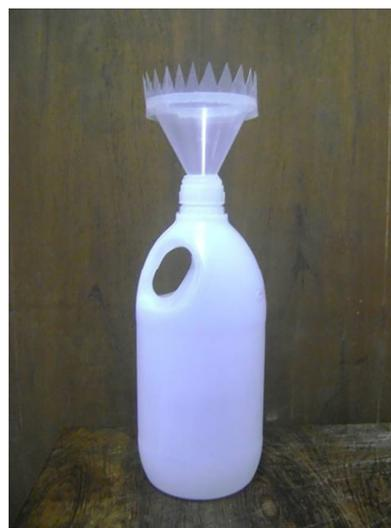
**Figure 2.** Design of the total deposition collector (adapted from reference 7).
