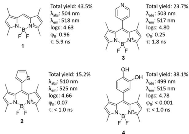
**Figure 1.** Structure and photophysical parameters of the BODIPYs synthesised, showing typical features of BODIPY dyes.
