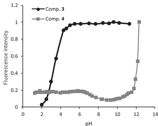
**Figure 4.** Influence of pH over intensity of fluorescence emission for compounds **3** and **4**. pH dependency was observed for both compounds.
