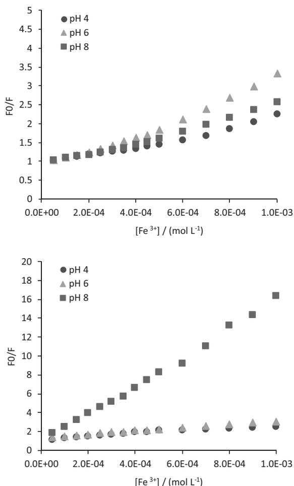
**Figure 5.** (Top) Stern-Volmer plots for the fluorescence quenching of **3** by  $FeCl_3$  in three pH values showing a relative pH-independency. (Bottom) Stern-Volmer plots for the fluorescence quenching of **4** by  $FeCl_3$  in three pH values. A significantly higher inclination at pH 6 reflects the higher sensitivity of the probe in this condition.
