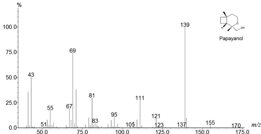
**Figure 3.** Mass spectrum and chemical structure of the natural male specific compound, papayanol.
