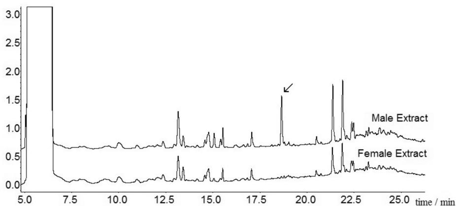
**Figure 1.** Gas chromatograms (FID) of headspace volatile extracts obtained from 24 h aeration of 10 males and females of *Conotrachelus psidii* containing host plant. The arrow indicates the male-specific compound.
