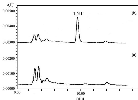
**Figure 8.** Chromatograms of extracted TNT from seawater (a) and spiked sample with 200  $\mu\text{g L}^{-1}$  of TNT by MMIP (b).
