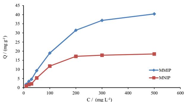
**Figure 6.** Adsorption equilibrium isotherm of MMIP and MNIP for TNT molecule (n = 3).
