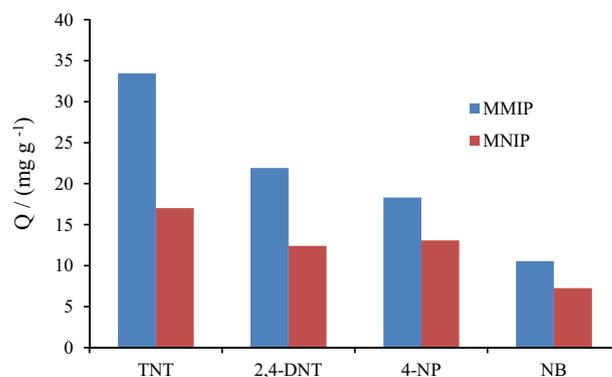
**Figure 7.** Adsorption selectivity for TNT and similar compounds by MMIP and MNIP under the optimized conditions at 200 mg L<sup>-1</sup> of concentration.
