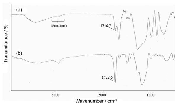
**Figure 2** FT-IR spectra of  $\text{Fe}_3\text{O}_4$ @MPTS (a) and TNT-MMIP (b).
