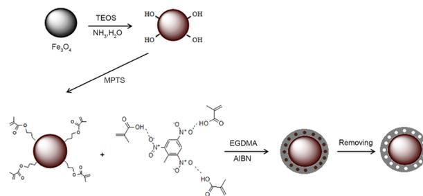
**Figure 1.** Synthesis route of TNT-MMIP by surface grafting polymerization.
