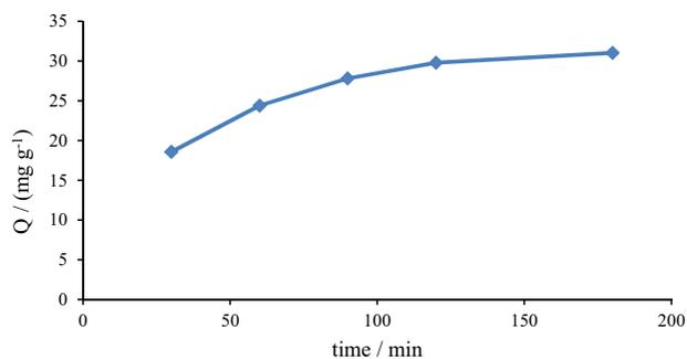
**Figure 5.** Kinetic adsorption curve for TNT adsorption at 200 mg L<sup>-1</sup> of concentration (n = 3).
