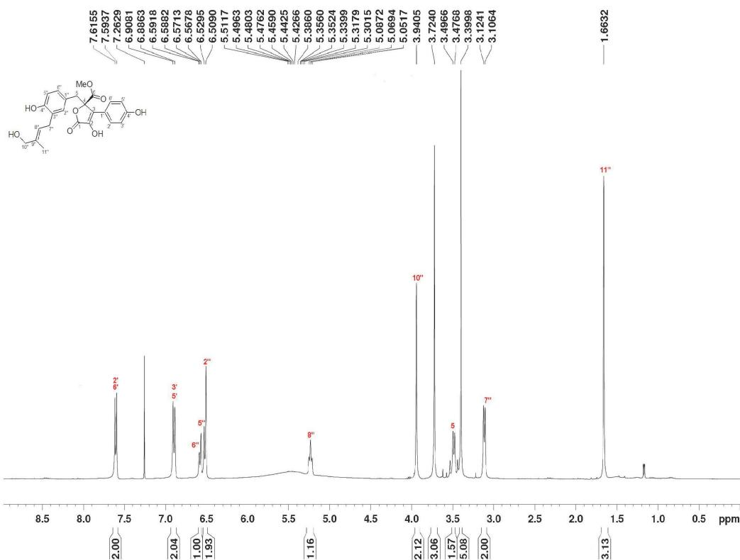
**Figure S8.**  $^1\text{H}$  NMR spectrum (400 MHz,  $\text{CDCl}_3$ ) of compound 2.
