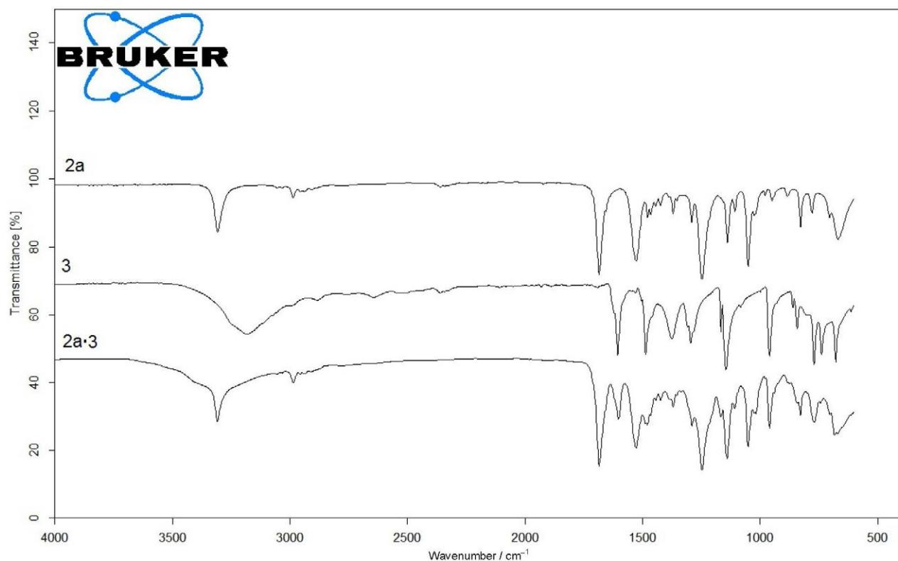
**Figure S17.** FT-IR spectra of **2a**, **3** and **2a·3** complex.
