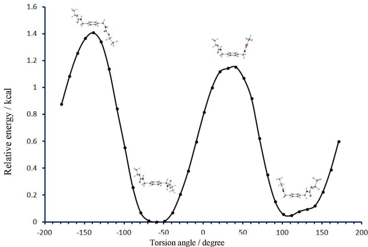
**Figure S12.** Potential energy as function of the C(2)-C(1)-C(7)-N(7) torsion angle in **2a**.
