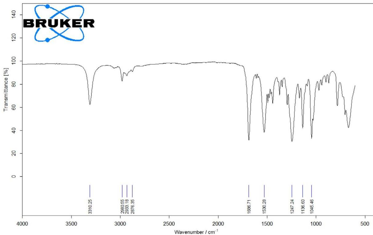
Figure S3. FT-IR spectra (neat, ATR) of 1a.
