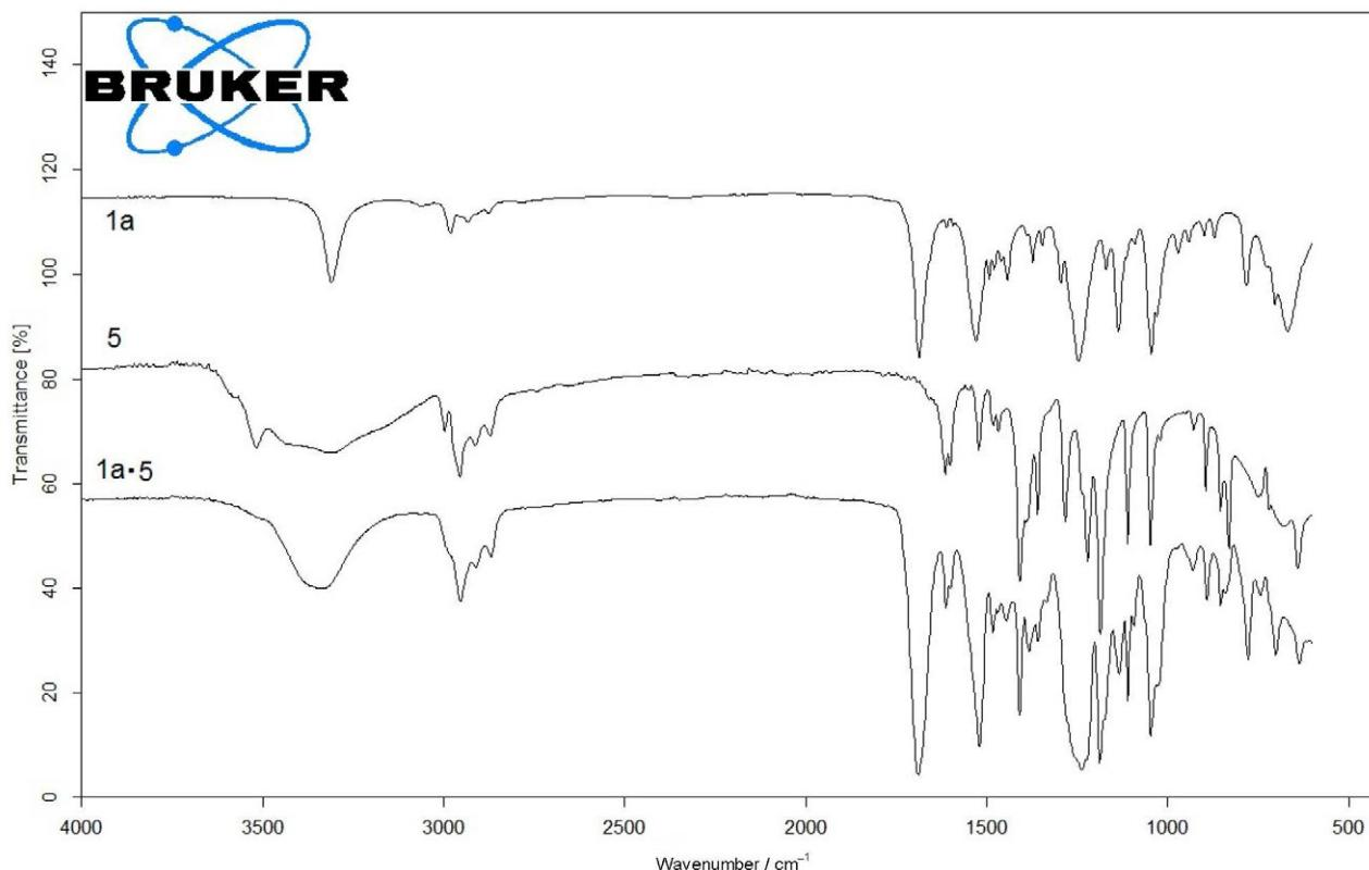
Figure S15. FT-IR spectra of **1a**, **5** and **1a·5** complex.
