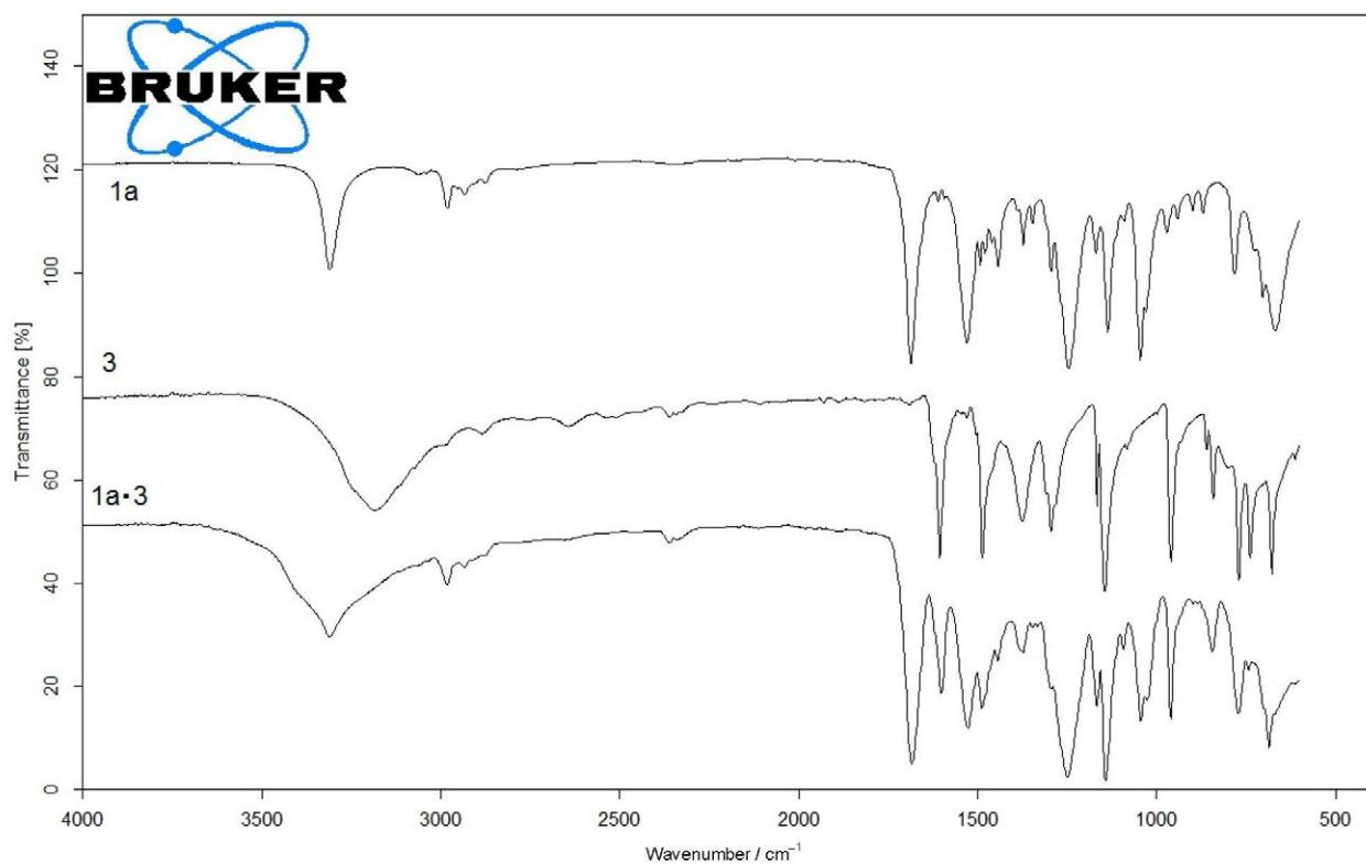
**Figure S13.** FT-IR spectra of **1a**, **3** and **1a·3** complex.
