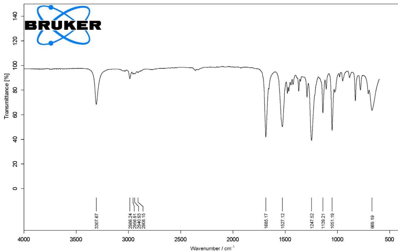
**Figure S8.** FT-IR spectra (neat, ATR) of **2a**.
