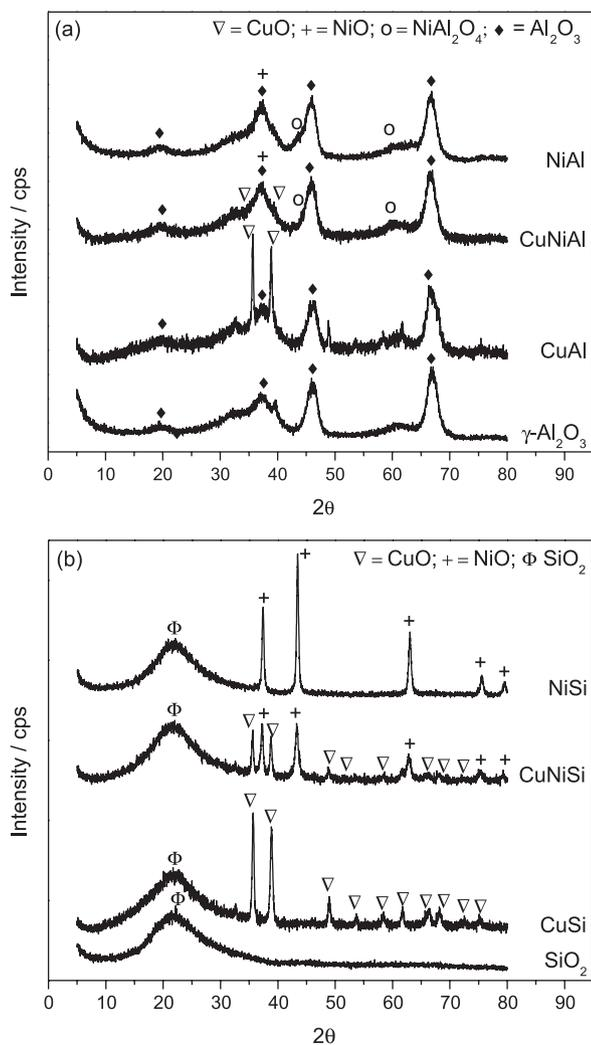
**Figure 2.** XRD patterns of catalysts supported (a) on  $\gamma$ -Al<sub>2</sub>O<sub>3</sub> and (b) on SiO<sub>2</sub>.
