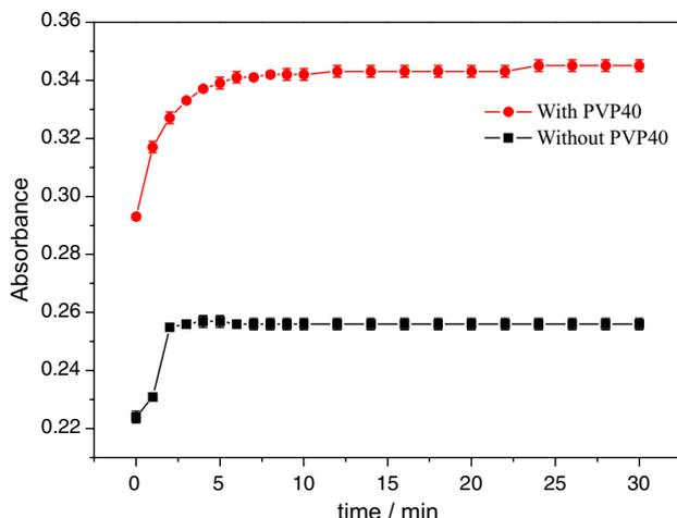
**Figure 4.** Effect of time on the development of absorbance by the Al-alizarin red S complex in the presence and absence of added PVP40. Bars represent standard deviation of three replicate measurements.
