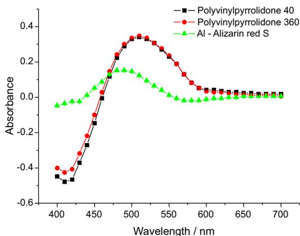
**Figure 1.** Absorption spectra of the Al-alizarin red S complex ( $100 \mu\text{g L}^{-1} \text{Al}^{3+}$ ) and the effect of added PVP40 and PVP360 surfactants at a final concentration of 0.8% m/v. Bars represent standard deviation of three replicate measurements.
