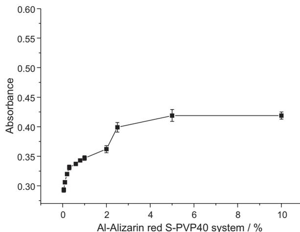
**Figure 2.** Effect of PVP40 concentration on absorbance from an aqueous standard solution containing  $100 \mu\text{g L}^{-1} \text{Al}^{3+}$ . Bars represent standard deviation of three replicate measurements.
