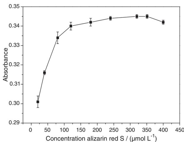
**Figure 3.** Effect of concentration of alizarin red S on absorbance from an aqueous standard solution containing  $100 \mu\text{g L}^{-1}$  of  $\text{Al}^{3+}$  and 1% m/v PVP40. Bars represent standard deviation of three replicate measurements.
