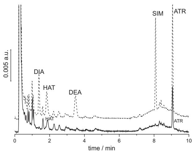
**Figure 4.** Chromatograms of a soil extract (continuous line) superposed to the chromatogram of an extract obtained from the  $1 \text{ mg kg}^{-1}$  spiked soil (dashed line) obtained in the core-shell column. Chromatographic conditions were described in caption of Figure 1d.
