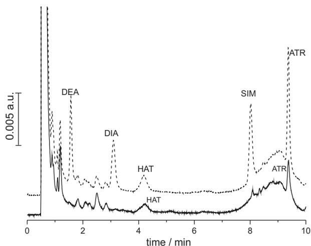
**Figure 3.** Chromatograms of a soil extract (continuous line) superposed to the chromatogram of an extract obtained from the  $1 \text{ mg kg}^{-1}$  spiked soil (dashed line) obtained in the monolithic column. Chromatographic conditions were described in caption of Figure 2b.
