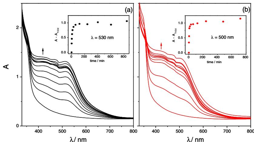
**Figure 7.** Absorption spectra of TiO<sub>2</sub> films being sensitized by *cis*-[Ru(Me<sub>4</sub>-phen)(dcbH<sub>2</sub>)(NCS)<sub>2</sub>] (a); or *cis*-[Ru(Me<sub>2</sub>-phen)(dcbH<sub>2</sub>)(NCS)<sub>2</sub>] (b). (Insets: absorption changes as a function of time).
