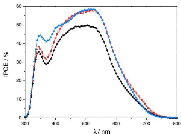
**Figure 8.** Photocurrent action spectra of *cis*-[Ru(Me<sub>4</sub>-phen)(dcbH<sub>2</sub>)(NCS)<sub>2</sub>] (●), *cis*-[Ru(Me<sub>2</sub>-phen)(dcbH<sub>2</sub>)(NCS)<sub>2</sub>] (□) and *cis*-[Ru(dcbH)<sub>2</sub>(NCS)<sub>2</sub>]<sup>2-</sup> (▲).
