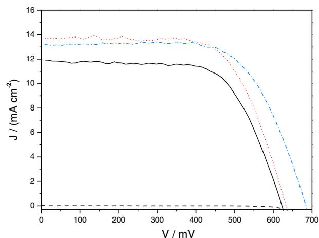
**Figure 9.** Current – voltage curves determined for *cis*-[Ru(Me<sub>4</sub>-phen)(dcbH<sub>2</sub>)(NCS)<sub>2</sub>] (—), *cis*-[Ru(Me<sub>2</sub>-phen)(dcbH<sub>2</sub>)(NCS)<sub>2</sub>] (⋯) and *cis*-[Ru(dcbH<sub>2</sub>)(NCS)<sub>2</sub>]<sup>2-</sup> (---) under AM 1.5 irradiation (P = 100 mW cm<sup>-2</sup>) and for *cis*-[Ru(dcbH<sub>2</sub>)(NCS)<sub>2</sub>]<sup>2-</sup> in the dark (---).
