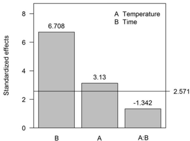
**Figure 1.** Pareto chart for the effects of temperature and time on the VOCs extraction.
