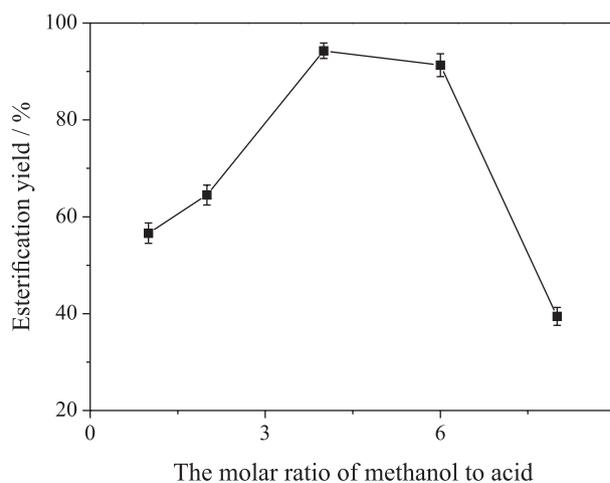
**Figure 2.** Effect of molar ratio on esterification catalyzed by CRL in DBSA microemulsion system (reaction conditions:  $w_0$  3.3, time 4 h, lipase 120  $\text{mg g}^{-1}$ ).
