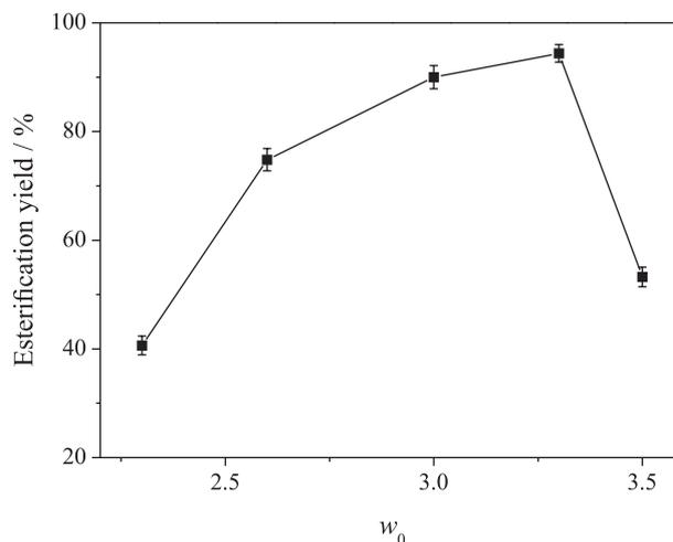
**Figure 1.** Effect of  $w_0$  on esterification catalyzed by CRL in DBSA microemulsion system (reaction conditions: molar ratio (alcohol/acid) 4, time 4 h, lipase 120  $\text{mg g}^{-1}$ ).
