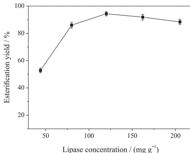
**Figure 4.** The effect of concentration of lipase on esterification in DBSA microemulsion system (reaction conditions: molar ratio (alcohol/acid) 4,  $w_0$  3.3, time 4 h).
