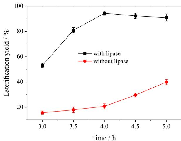
**Figure 3.** Effect of reaction time on esterification catalyzed by CRL and without CRL in DBSA microemulsion system (reaction conditions: molar ratio (alcohol/acid) 4,  $w_0$  3.3, lipase 120 mg g<sup>-1</sup>).
