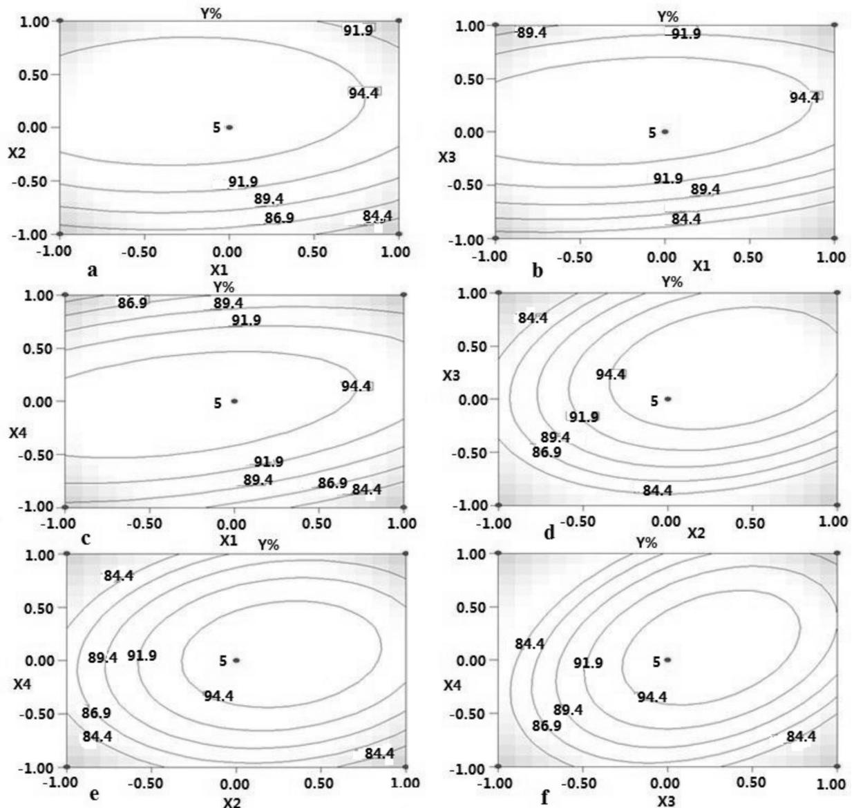
**Figure 6.** Response surface contour plots of interaction between the four independent factors on yield of biodiesel. (a) Effect of  $w_0$  and reaction time; (b) effect of  $w_0$  and methanol/acid molar ratio; (c) effect of  $w_0$  and lipase concentration; (d) effect of reaction time and methanol/acid molar ratio; (e) effect of reaction time and lipase concentration; (f) effect of methanol/acid molar ratio and lipase concentration.
