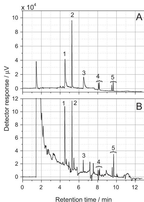
**Figure 2.** Chromatogram of a standard solution of pesticides in acetonitrile (A) and in the organic extract of tomato (B) at a concentration of 100 μg L<sup>-1</sup>, where: 1: chlorothalonil; 2: chlorpyrifos; 3: iprodione; 4: permethrin and 5: deltamethrin.
