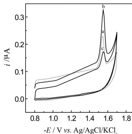
**Figure 3.** Cyclic voltammograms of  $1.0 \times 10^{-6} \text{ mol L}^{-1}$  LV.HCl in the BR universal buffer at pH 7.0 recorded following its preconcentration onto HMDE by adsorptive preconcentration under open circuit conditions (a) and then at  $E_{acc} = -0.8 \text{ V}$  for 20 s (1<sup>st</sup> cycle (b) and 2<sup>nd</sup> cycle (c)); scan rate =  $100 \text{ mV s}^{-1}$ .
