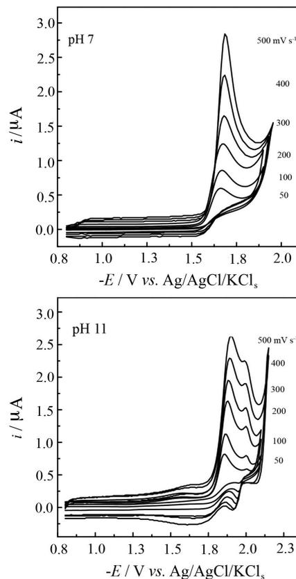
**Figure 1.** Voltammograms of  $1.0 \times 10^{-4}$  mol L $^{-1}$  LV.HCl in the BR universal buffer of various pH values at various scan rates.
