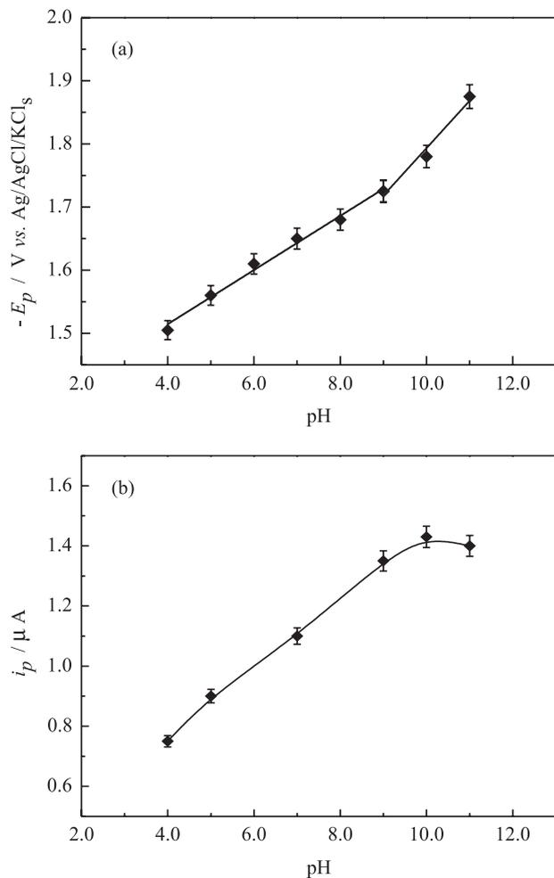
**Figure 2.** (a)  $E_p$  vs. pH and (b)  $i_p$  vs. pH plots for LV.HCl at various pH values (scan rate = 200 mV s<sup>-1</sup>).
