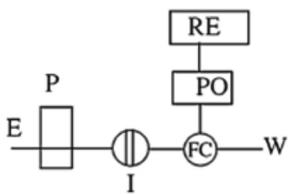
**Figure 1.** Scheme of the FIA apparatus for morpholine determination.
