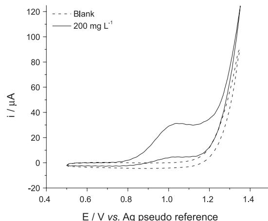
**Figure 2.** Cyclic voltammograms obtained in the absence and presence of (200 mg L<sup>-1</sup>) morpholine standard solution in 0.1 mol L<sup>-1</sup> KCl using SPCEs.
