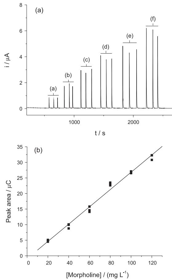
**Figure 4.** Amperometric (a) and analytical (b) curves recorded using several morpholine concentrations in  $0.1 \text{ mol L}^{-1}$  KCl solution at  $1.0 \text{ V}$  using FIA and screen-printed electrodes. Morpholine concentrations: (a)  $20 \text{ mg L}^{-1}$ ; (b)  $40 \text{ mg L}^{-1}$ ; (c)  $60 \text{ mg L}^{-1}$ ; (d)  $80 \text{ mg L}^{-1}$ ; (e)  $100 \text{ mg L}^{-1}$ ; (f)  $120 \text{ mg L}^{-1}$ .
