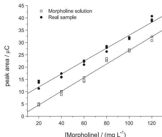
**Figure 7.** Matrix effect study for the amperometric method using FIA.
