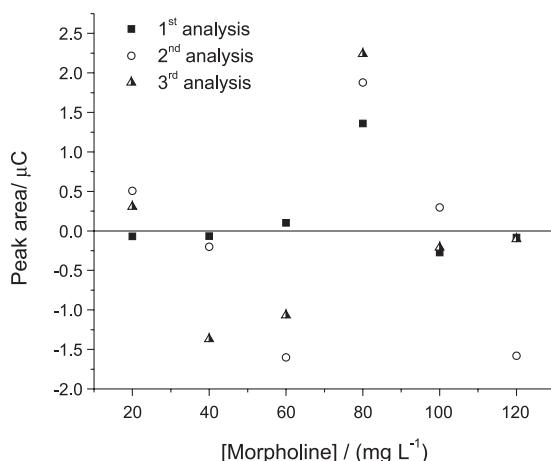
**Figure 5.** Residue graph from the analytical curve obtained by the amperometric method using FIA and screen-printed electrodes.
