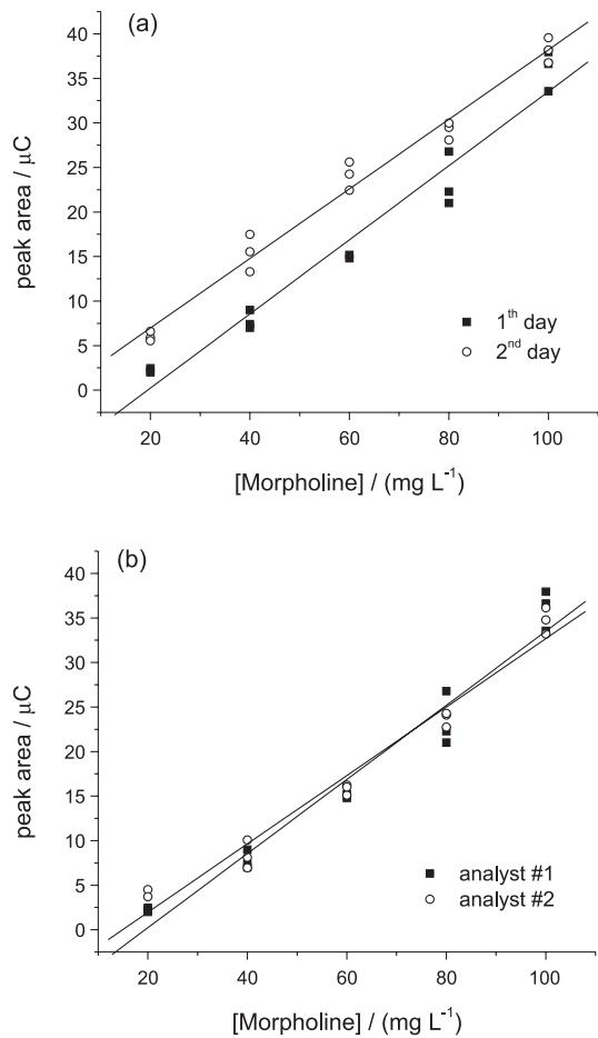
**Figure 6.** Precision study for the amperometric method: (a) analytical curves obtained on different days and (b) analytical curves obtained by different operators.
