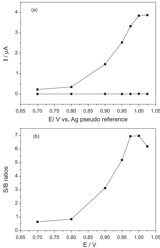
**Figure 3.** (a) Hydrodynamic voltammogram in the absence and presence of a  $70 \text{ mg L}^{-1}$  morpholine solution with the averages of the peak currents from four injections (the analyte solution was injected four times at each potential, and then the average peak current was obtained by calculation), using  $0.1 \text{ mol L}^{-1}$  KCl solution as a carrier stream. (b) Hydrodynamic of the signal-to-blank ratio. The flow rate was  $1.5 \text{ mL min}^{-1}$ .
