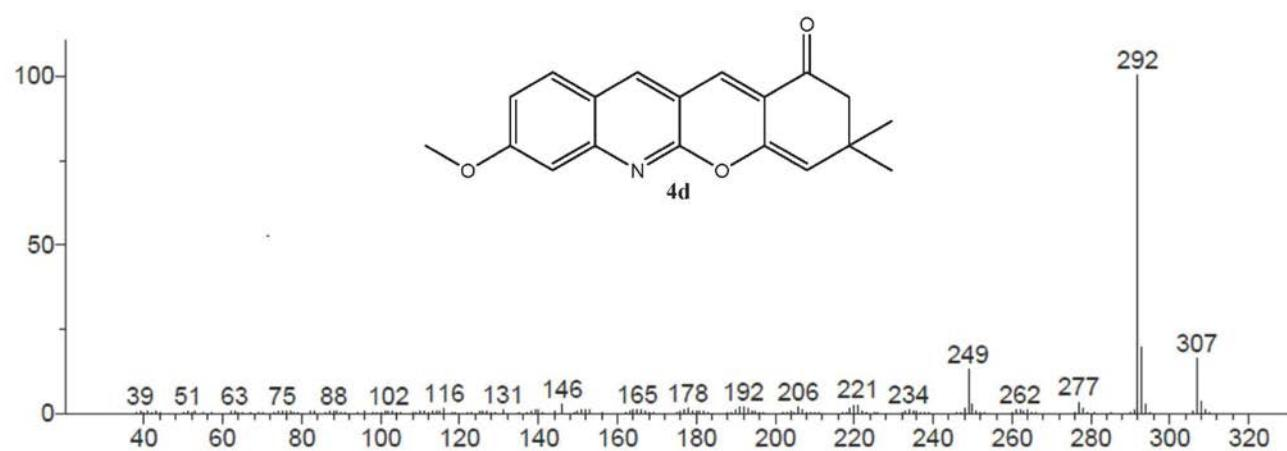
Figure S29. EI-MS spectrum of **4d**.
