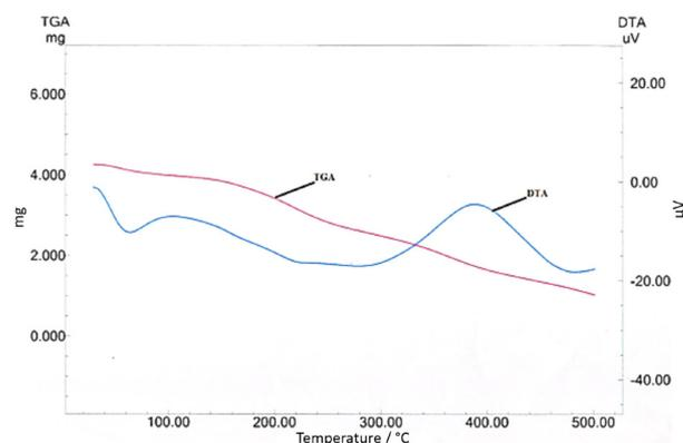
Figure 6. TG/DTA graph of cellulose sulfuric acid.
