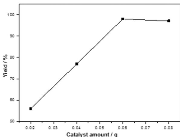
Figure 7. Effect of catalyst loading on the model reaction.
