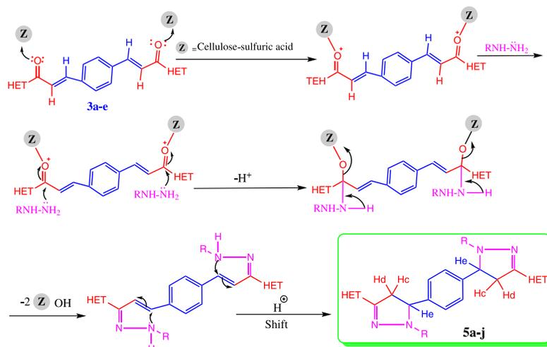
**Scheme 3.** Plausible mechanism for the synthesis of bis-pyrazolines (**5a-j**).
