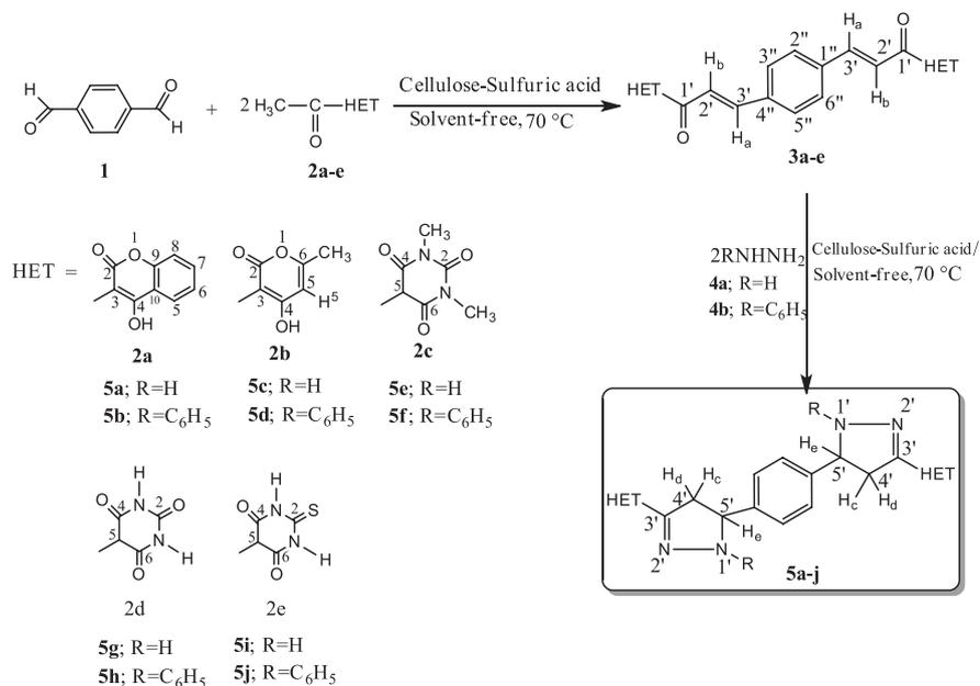
**Scheme 1.** Synthetic route of bis-chalcones (3a-e) and bis-pyrazolines (5a-j).
