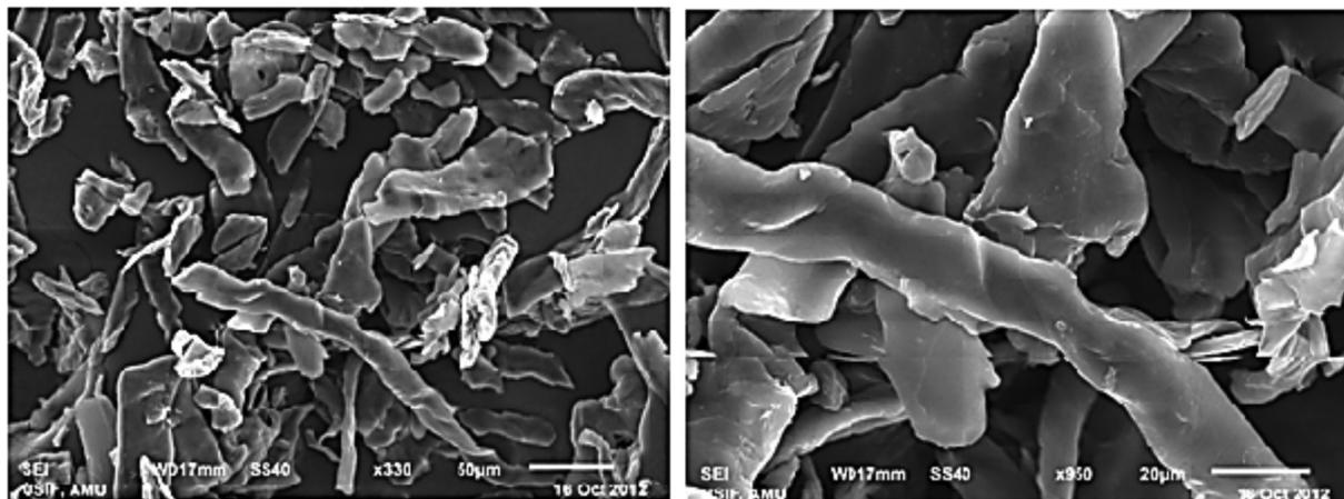
Figure 4. SEM images of the catalyst (CSA) at different magnifications.
