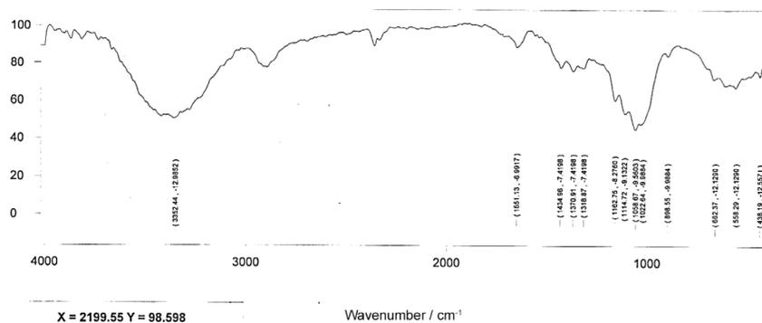
Figure 2. FT-IR spectra of cellulose sulfuric acid.
