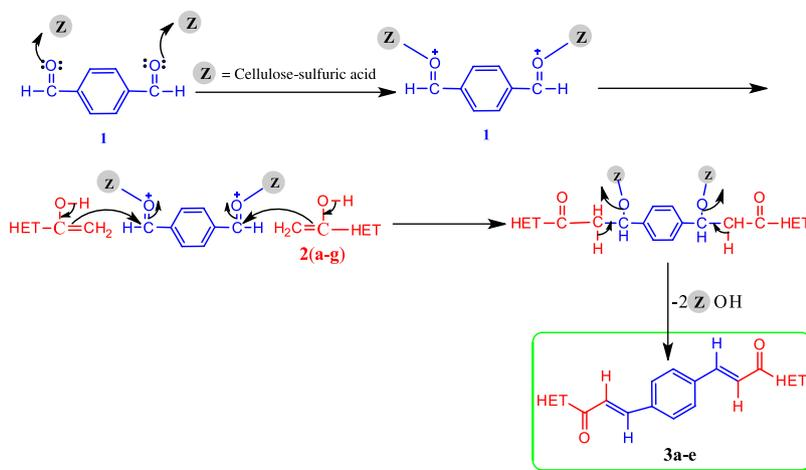
**Scheme 2.** Plausible mechanism for the synthesis of bis-chalcones (3a-e).
