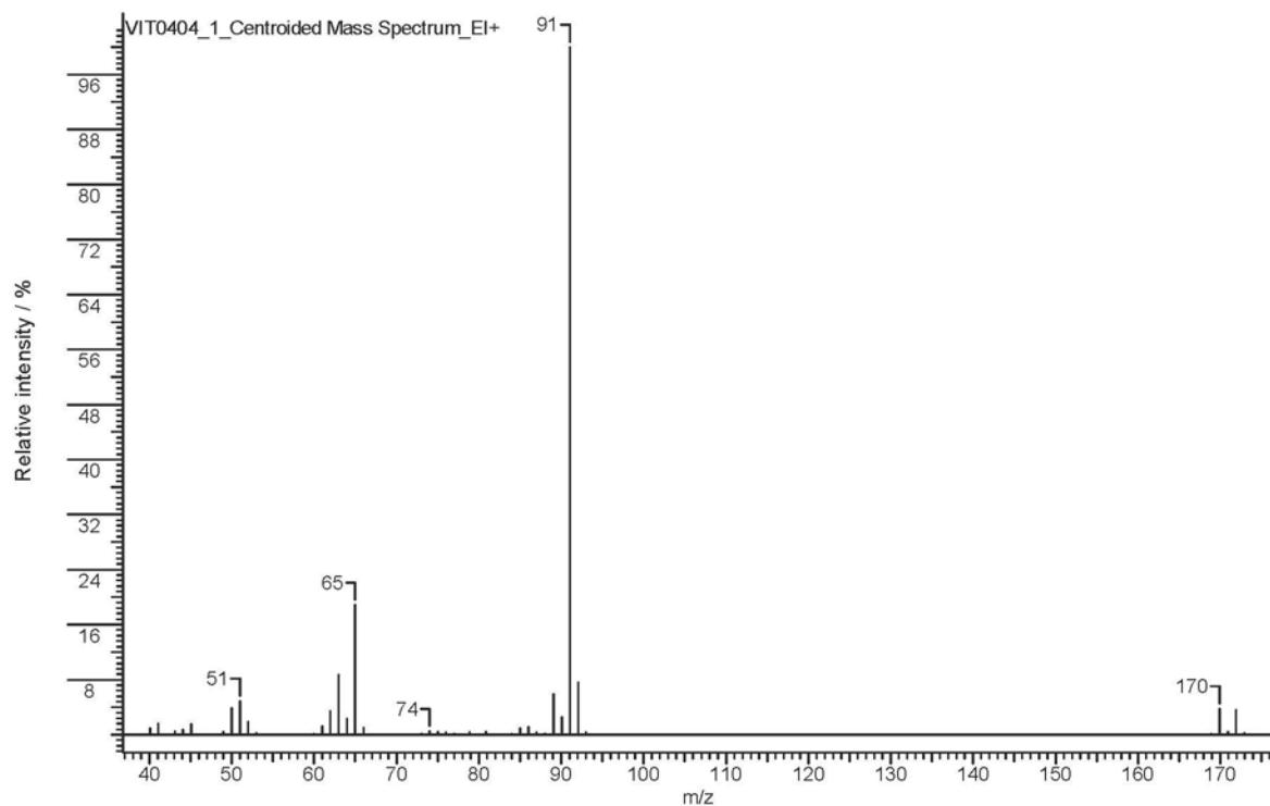
**Figure S16.** Mass spectrum (70 eV) of benzyl bromide.
