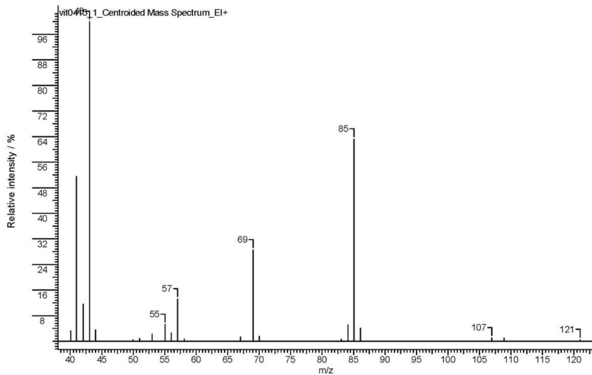
**Figure S32.** Mass spectrum (70 eV) of 2-bromo-4-methylpentane.
