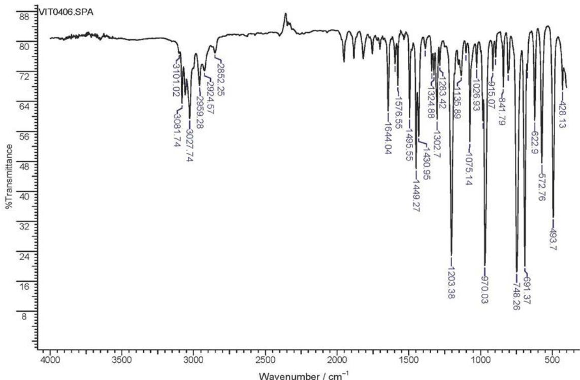
Figure S19. IR spectrum ( $\text{KBr}$ ) of cinnamyl bromide.
