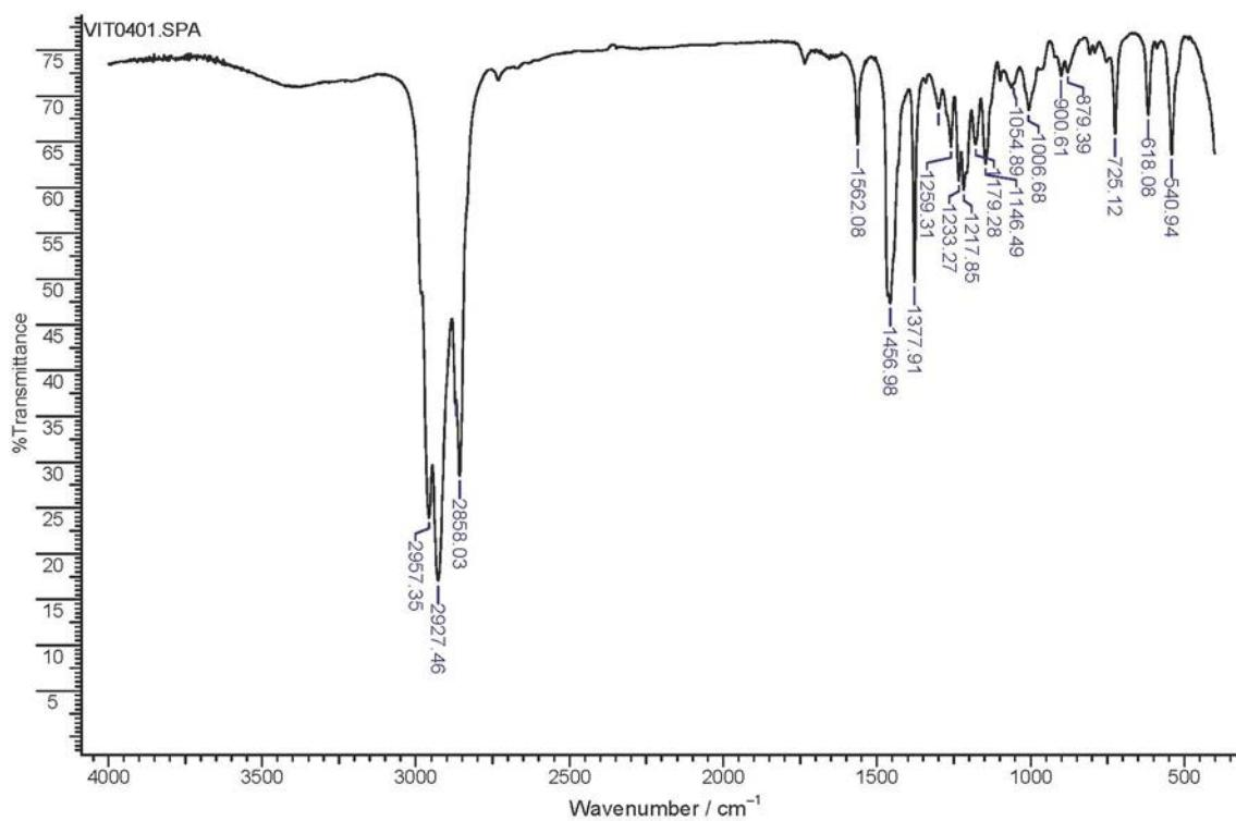
Figure S3. IR spectrum (KBr) of 2-bromooctane.
