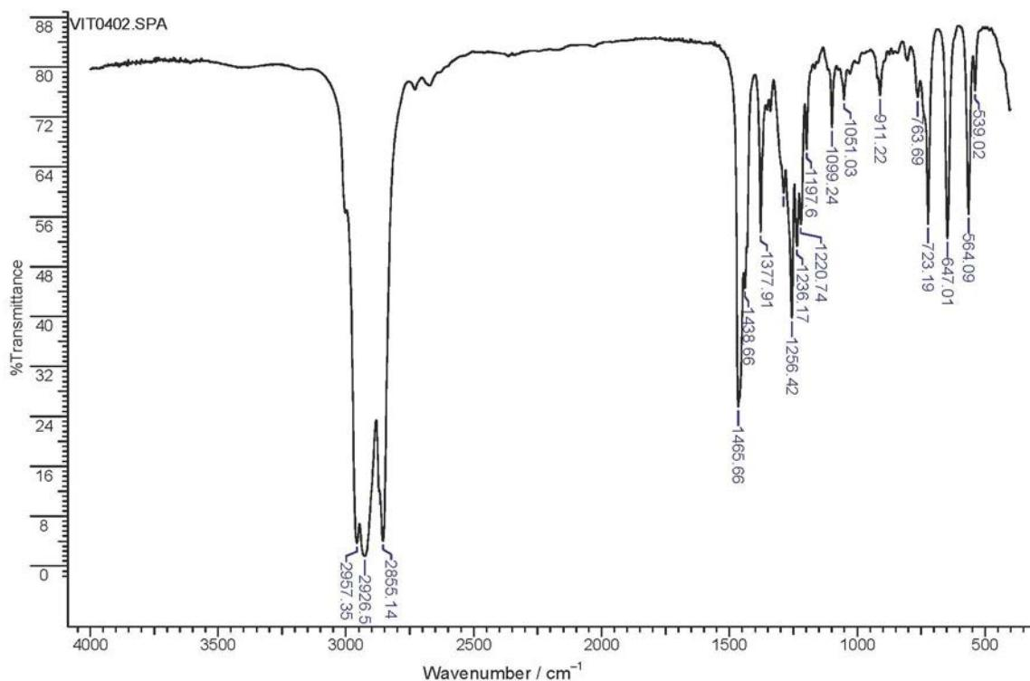
**Figure S7.** IR spectrum ( $\text{KBr}$ ) of 1-bromooctane.
