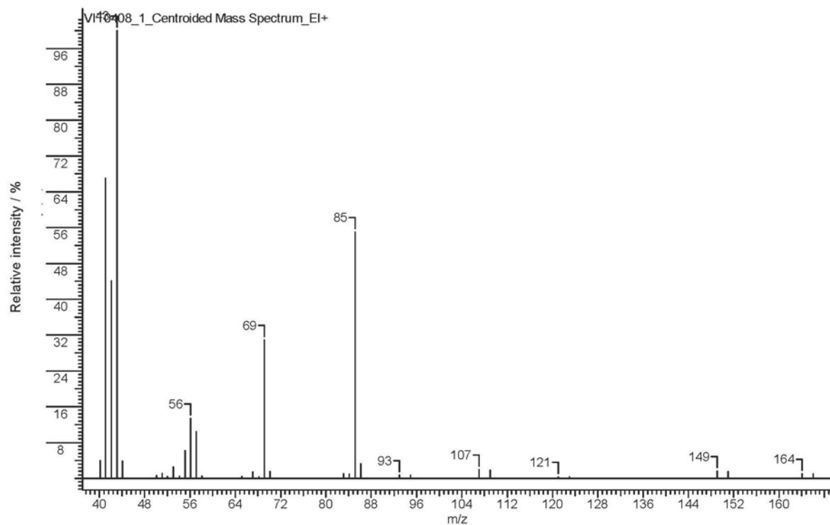
**Figure S28.** Mass spectrum (70 eV) of 1-bromo-4-methylpentane.
