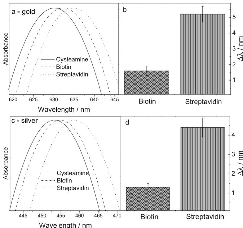
**Figure 6.** Application of gold nanoparticle multilayer film (on top) and silver nanoparticle multilayer film (bottom) to detect surface binding in the assembly process of cysteamine monolayer-biotin linker-streptavidin protein system. (b) and (d) SPR shift measured relative to cysteamine after the adsorption of biotin and streptavidin on the nanoparticles.
