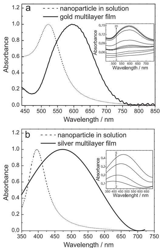
**Figure 2.** Absorption spectra from (a) gold nanoparticles in solution, gold multilayer film (20 layers), (b) silver nanoparticles in solution and silver multilayer film (5 layers). Insets: Absorbance as a function of the number of layers from (a) gold and (b) silver nanoparticles multilayer films.
