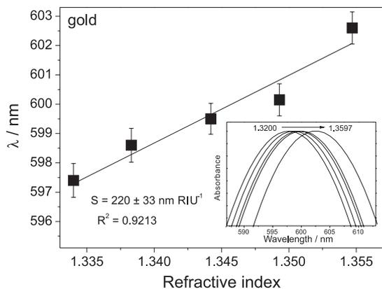
**Figure 4.** Surface plasmon resonance position of gold nanoparticle multilayer film (20 layers) as a function of the refractive index. Inset: normalized absorption spectra of gold plasmonic substrate in different refractive index.
