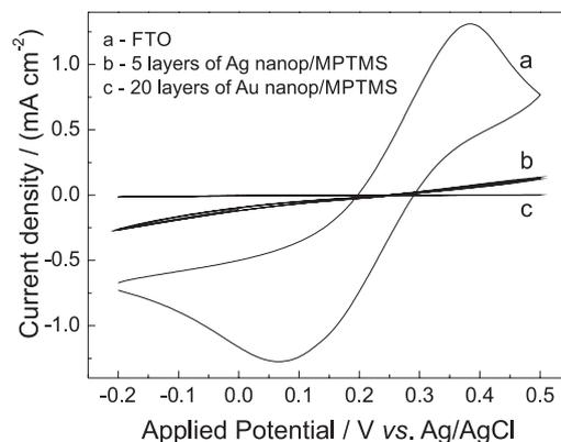
**Figure 3.** Voltammograms of 1 mmol L<sup>-1</sup> of  $K_3[Fe(CN)_6]$  and 0.1 mol L<sup>-1</sup> of KCl solution on (a) bare FTO electrode, (b) 5 layers of silver nanoparticles covered FTO electrode and (c) 20 layers of gold nanoparticles covered electrode.
