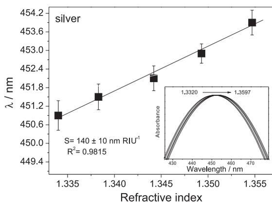
**Figure 5.** Surface plasmon resonance mode of silver nanoparticle multilayer film (5 layers) as a function of the refractive index. Inset: normalized absorption spectra of silver plasmonic substrate in different refractive index.
