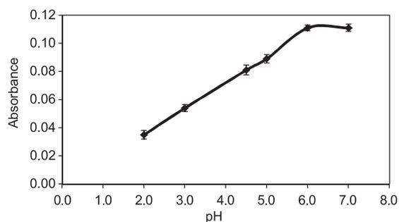
**Figure 2.** Effect of pH sample on Se(IV) extraction. Aqueous phase volume, 10 mL; [Se(IV)], 100.0  $\mu\text{g L}^{-1}$ ; formic acid 20%, 0.25 mL; DAB,  $1.6 \times 10^{-3} \text{ mol L}^{-1}$ ; extracting solvent, 100.0  $\mu\text{L}$ ; dispersive solvent, 150.0  $\mu\text{L}$ ; n = 3.
