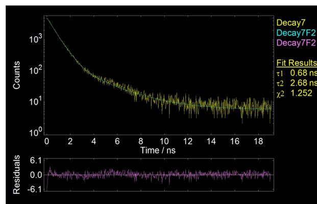
**Figure 6.** Luminescent lifetime curve of **6** monitored at corresponding excitation/emission maxima, which can be fitted with double-exponential decay, fitting results:  $\tau_1 = 0.68$  ns,  $\tau_2 = 2.68$  ns ( $\chi^2 = 1.252$ ).
