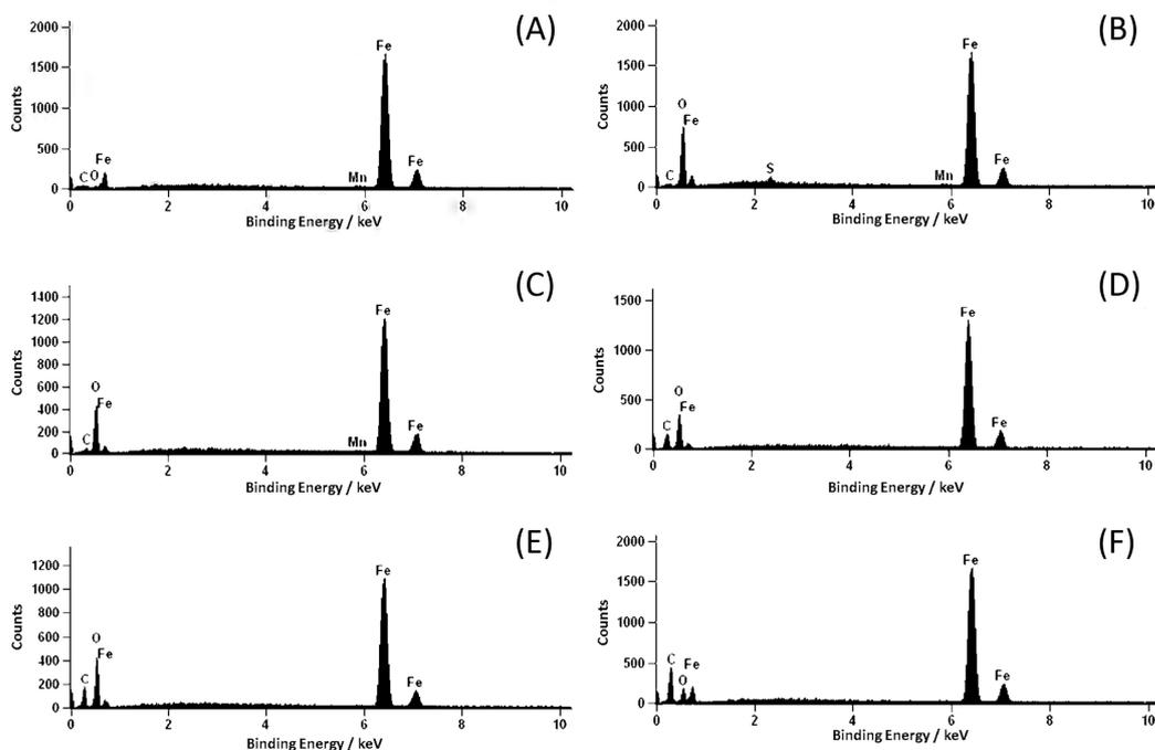
**Figure 8.** EDS spectra for the mild steel surface of (A) the reference coupon, and after 24 h of immersion in (B)  $0.1 \text{ mol L}^{-1} \text{H}_2\text{SO}_4$  and solutions containing (C) 1.0, (D) 3.0, (E) 5.0 and (F)  $10.0 \text{ mmol L}^{-1}$  of caffeine.
