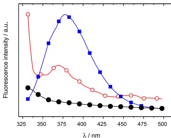
**Figure 9.** Fluorescence emission spectra for (●) the mild steel surface, (○) the mild steel surface after 24 h of immersion in 0.1 mol L<sup>-1</sup> H<sub>2</sub>SO<sub>4</sub> in the presence of 10 mmol L<sup>-1</sup> caffeine and (■) 10 mmol L<sup>-1</sup> caffeine in 0.1 mol L<sup>-1</sup> H<sub>2</sub>SO<sub>4</sub> aqueous solution.
