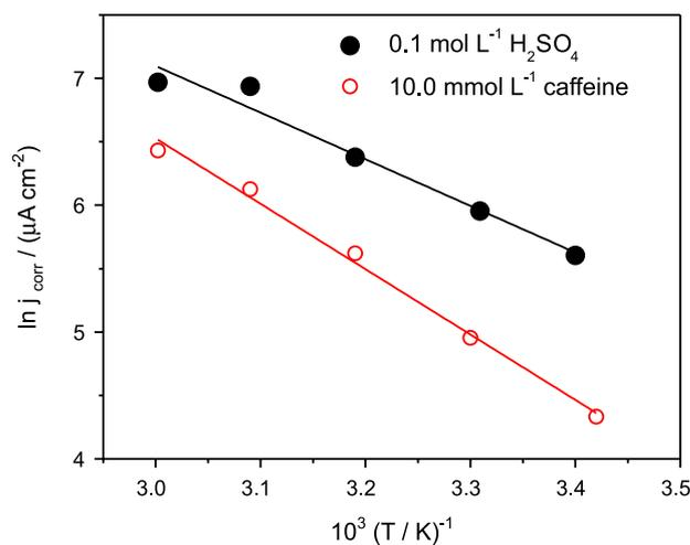
**Figure 4.** Arrhenius plot for mild steel in 0.1 mol L<sup>-1</sup> H<sub>2</sub>SO<sub>4</sub> and solutions containing 10.0 mmol L<sup>-1</sup> of caffeine.
