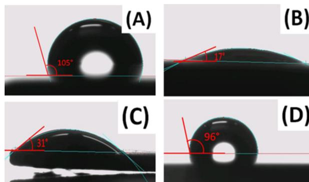
**Figure 6.** Water droplet contact angles on mild steel surfaces: (A) reference, and after 24 h in  $0.1 \text{ mol L}^{-1} \text{ H}_2\text{SO}_4$  in (B) the absence and presence of (C)  $10 \text{ mmol L}^{-1}$  and (D)  $50 \text{ mmol L}^{-1}$  of caffeine.
