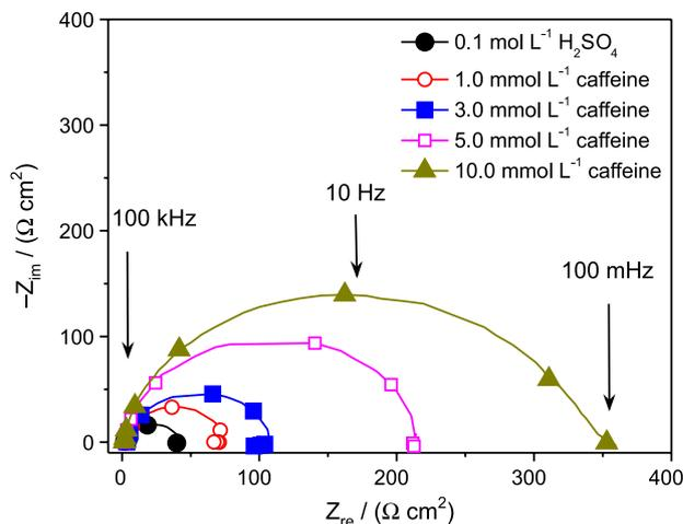
**Figure 3.** Nyquist plots for mild steel in  $0.1 \text{ mol L}^{-1} \text{ H}_2\text{SO}_4$  and solutions containing  $1.0$  to  $10.0 \text{ mmol L}^{-1}$  of caffeine.
