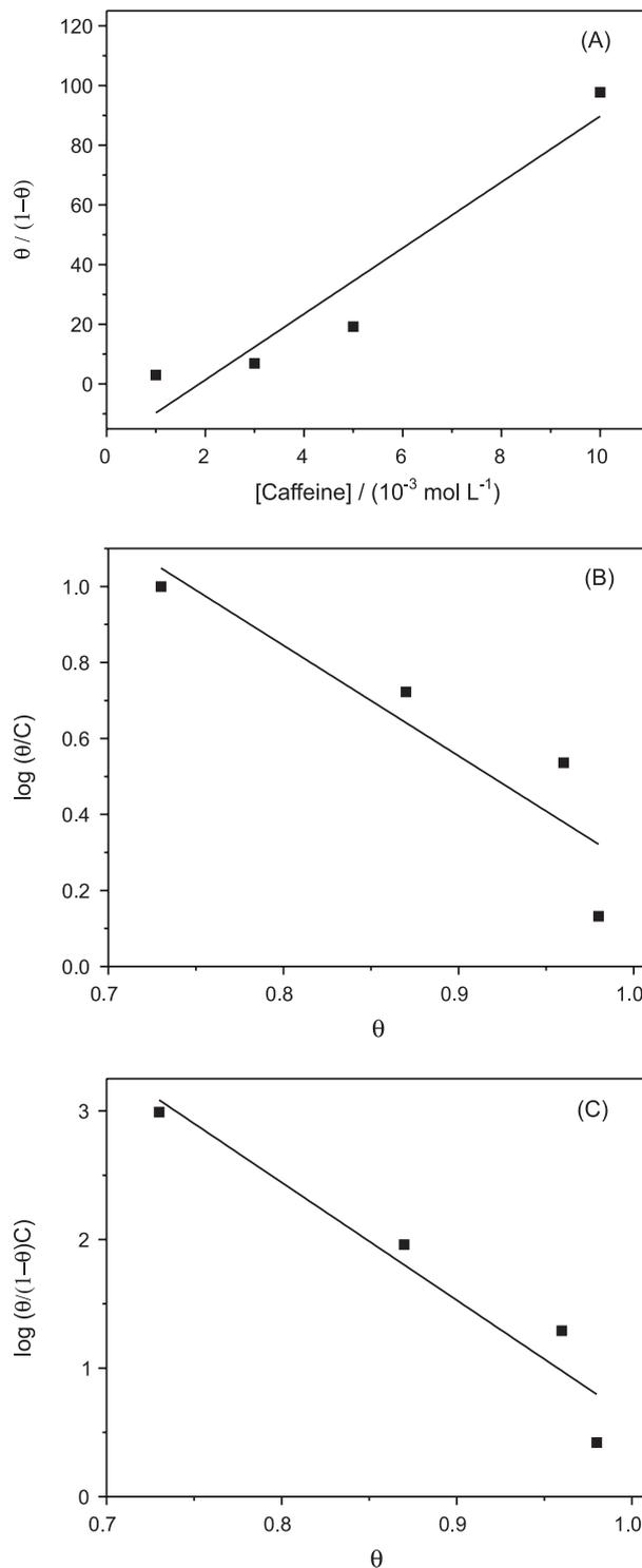
**Figure 5.** (A) Langmuir, (B) Temkin and (C) Frumkin isotherms for the adsorption of caffeine onto the mild steel surface in  $0.1 \text{ mol L}^{-1} \text{ H}_2\text{SO}_4$  solutions.
