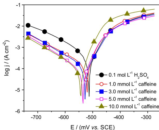
**Figure 2.** Potentiodynamic polarization curves for mild steel in 0.1 mol L<sup>-1</sup> H<sub>2</sub>SO<sub>4</sub> and solutions containing 1.0 to 10.0 mmol L<sup>-1</sup> of caffeine.
