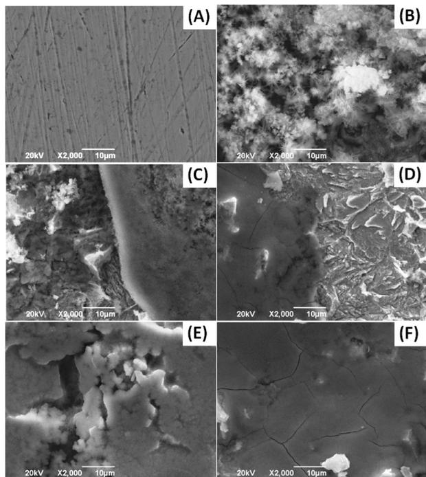
**Figure 7.** SEM images of mild steel surface for (A) reference coupon and after 24 h of immersion in (B)  $0.1 \text{ mol L}^{-1} \text{H}_2\text{SO}_4$  and solutions containing (C) 1.0, (D) 3.0, (E) 5.0 and (F)  $10.0 \text{ mmol L}^{-1}$  of caffeine.
