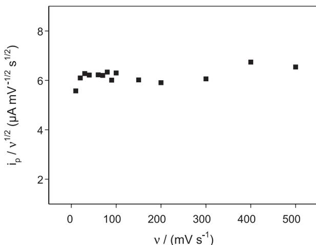
**Figure 3.** Variation of the current function ( $i_p/v^{1/2}$ ) in relation to the potential scan rate for a solution of 1.00 mmol L<sup>-1</sup> TBH in 0.10 mol L<sup>-1</sup> KOH using GCE.
