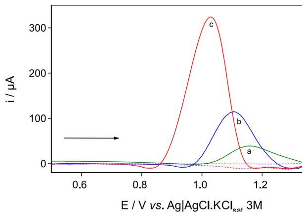
**Figure 4.** Comparison between the (a) LSV, (b) SWV, and (c) DPV experiments in optimized conditions for 1.00 mmol L<sup>-1</sup> TBH at GCE in 0.10 mol L<sup>-1</sup> KOH.
