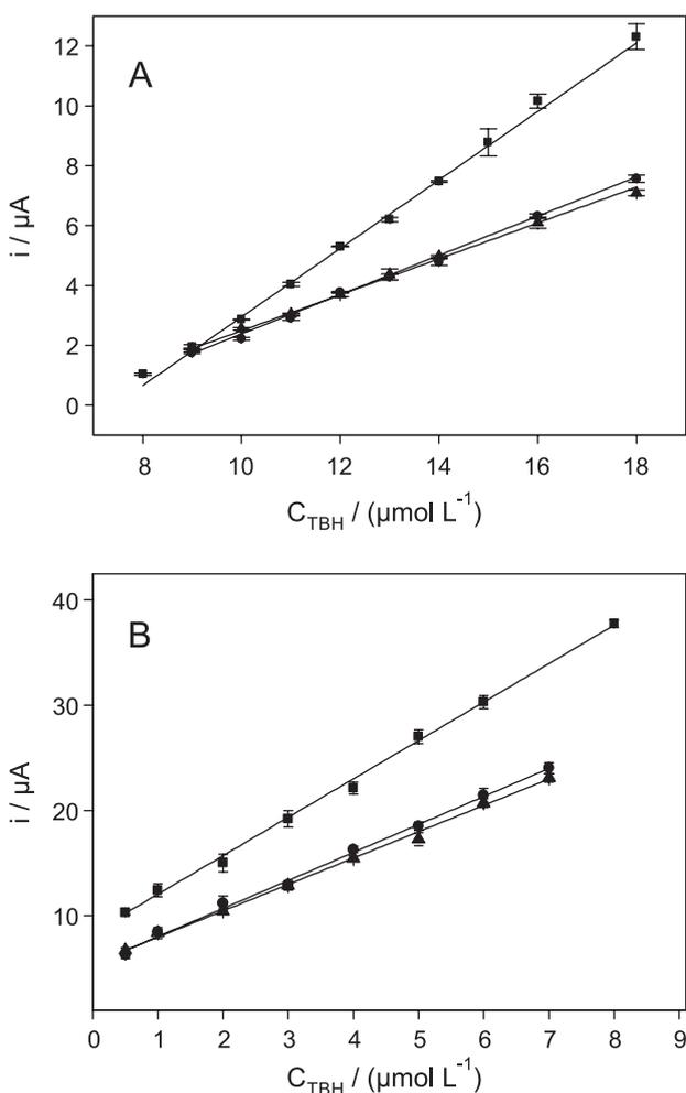
**Figure 6.** Analytical curves obtained by (A) SWV in the absence of matrix (■), presence of brown sugar matrix (●), and presence of crystal sugar (▲). (B) DPV in the absence of matrix (■), presence of brown sugar matrix (●), and presence of crystal sugar matrix (▲) using glassy carbon electrode and 0.10 mol L<sup>-1</sup> KOH as supporting electrolyte.
