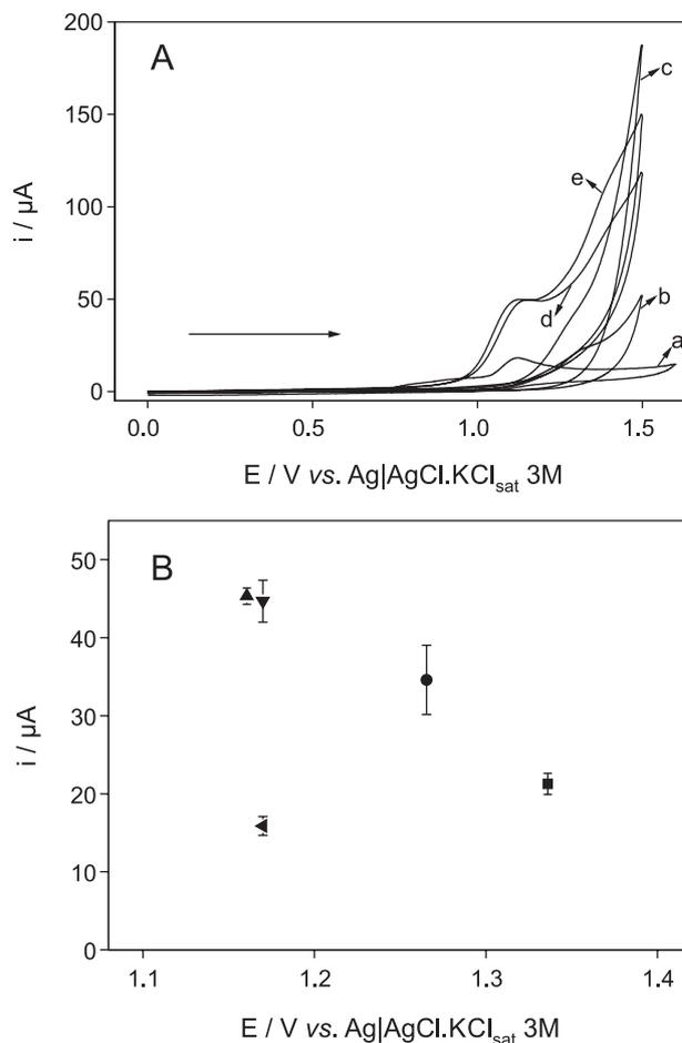
**Figure 2.** Cyclic voltammograms using (A)  $\text{BF}_4\text{TBA/DMF}$  (a), carbonate buffer (b), ammonia buffer (c),  $\text{NaOH}$  (d), and  $\text{KOH}$  (e) as the supporting electrolyte solution in the analysis of 1.00  $\text{mmol L}^{-1}$  TBH and (B) relationship between the peak current and peak potential using  $\text{BF}_4\text{TBA/DMF}$  (●), ammonia buffer (■), carbonate buffer (●),  $\text{NaOH}$  (▼), and  $\text{KOH}$  (▲). Conditions:  $v = 50 \text{ mV s}^{-1}$ .
