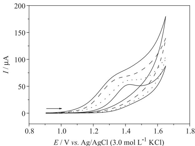
**Figure 5.** Cyclic voltammograms ( $50 \text{ mV s}^{-1}$ ) of  $1.0 \text{ mmol L}^{-1}$  PTU solutions in BR buffers of different pH values: 2.0 (solid thick line), 3.0 (dotted line), 4.0 (dashed line), and 5.0 (solid line) using a cathodically pretreated BDD electrode.
