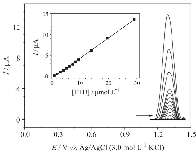
**Figure 7.** Differential pulse voltammograms obtained using the cathodically pretreated BDD electrode for (1) 1.0, (2) 2.0, (3) 3.2, (4) 4.3, (5) 5.3, (6) 6.3, (7) 7.5, (8) 8.5, (9) 9.5, (10) 14.0, (11) 20.0, and (12) 29.1  $\mu\text{mol L}^{-1}$  PTU solutions in the BR buffer (pH 2.0). Insert: corresponding analytical curve.
