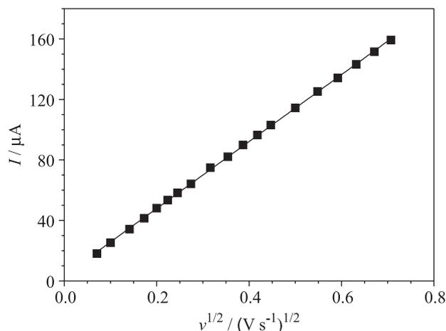
**Figure 6.** Linear dependence of the peak current ( $I_{ap}$ ) with the square root of the scan rate ( $v^{1/2}$ ) for cyclic voltammograms of a  $1.0 \text{ mmol L}^{-1}$  PTU solution in the BR buffer (pH 2.0) using a cathodically BDD electrode at different scan rates ( $0.005\text{-}0.500 \text{ V s}^{-1}$ ).
