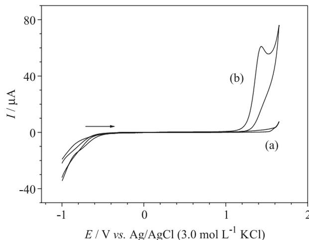
**Figure 2.** Cyclic voltammograms ( $50 \text{ mV s}^{-1}$ ) obtained using a cathodically pretreated BDD electrode for a: (a) BR buffer solution (pH 2.0); (b)  $1.0 \text{ mmol L}^{-1}$  PTU solution in the BR buffer (pH 2.0).
