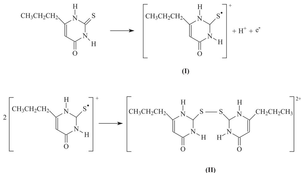
**Figure 4.** Proposed oxidation mechanism for propylthiouracil and its dimerization to a disulfide compound.
