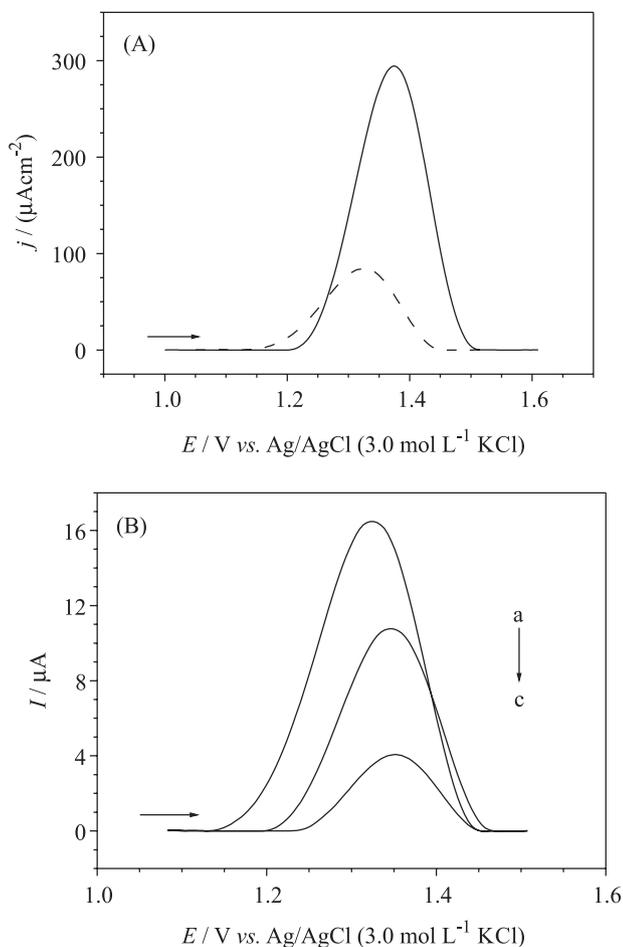
**Figure 8.** Differential pulse voltammograms for a 500  $\mu\text{mol L}^{-1}$  PTU solution in the BR buffer (pH 2.0) obtained on: (A) GC (dashed line) and BDD (solid line) electrodes; (B) a GC electrode for the (a) first, (b) second, and (c) third scans.
