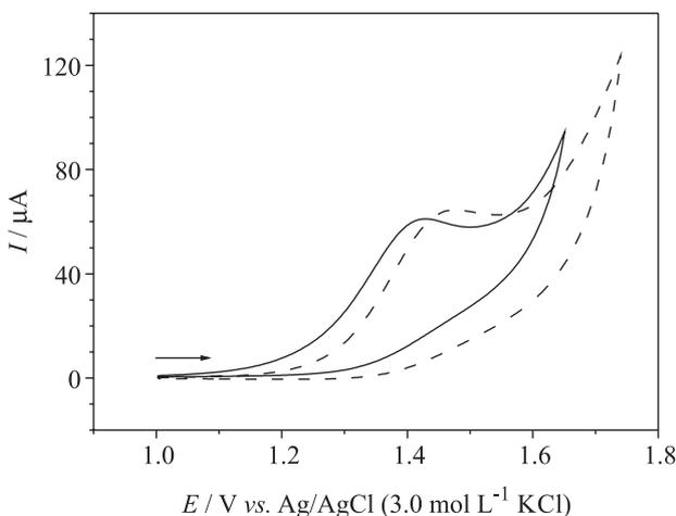
**Figure 3.** Cyclic voltammograms ( $50 \text{ mV s}^{-1}$ ) obtained for a  $1.0 \text{ mmol L}^{-1}$  PTU solution in the BR buffer (pH 2.0) using a BDD electrode after it underwent an anodic (dashed line) or cathodic (solid line) pretreatment (see text).
