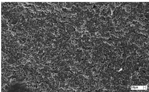
**Figure 2.** SEM image of the working electrode surface of a EIGPU, under a 500x magnification.
