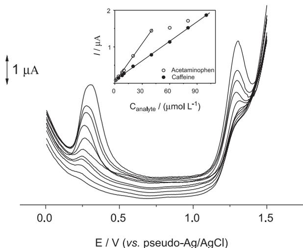
**Figure 6.** Differential pulse voltammetric curves obtained at the EIGPU for acetaminophen and caffeine at equal concentrations between 1.00 and 200  $\mu\text{mol L}^{-1}$ , scan rate 25  $\text{mV s}^{-1}$  and pulse amplitude 75 mV. In set the analytical curve.
