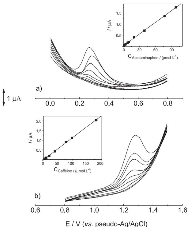
**Figure 4.** Differential pulse voltammetric curves obtained for a) acetaminophen and b) caffeine, in 0.100 mol  $\text{L}^{-1}$  phosphate buffer pH 6.0, at concentrations between 1.00 and 200  $\mu\text{mol L}^{-1}$ , scan rate 25  $\text{mV s}^{-1}$  and pulse amplitude 75 mV. In the inset, the analytical curve.
