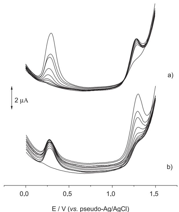
**Figure 5.** Differential pulse voltammograms obtained at the EIGPU for a) acetaminophen at concentrations between 1.00 and 200  $\mu\text{mol L}^{-1}$  in the presence of  $6.0 \times 10^{-5}$  mol  $\text{L}^{-1}$  caffeine; b) caffeine at concentrations between 1.00 and 200  $\mu\text{mol L}^{-1}$  in the presence of  $6.0 \times 10^{-5}$  mol  $\text{L}^{-1}$  acetaminophen. Scan rate 25  $\text{mV s}^{-1}$  and pulse amplitude 75 mV.
