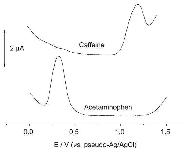
**Figure 3.** Differential pulse voltammetric curves obtained for  $1.0 \times 10^{-4} \text{ mol L}^{-1}$  acetaminophen and caffeine, in 0.100  $\text{mol L}^{-1}$  phosphate buffer pH 6.0, scan rate 25  $\text{mV s}^{-1}$  and pulse amplitude 75 mV.
