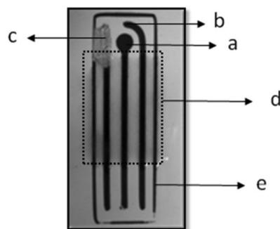
**Figure 1.** Design of the EIGPU with the components: working electrode (a), auxiliary electrode (b), silver glue (c), insulating (d) and electrical contact (e).
