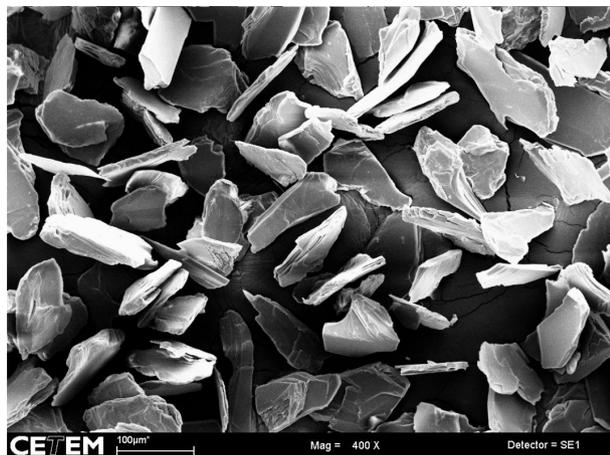
Figure 3. SEM micrograph of the phlogopite sample.
