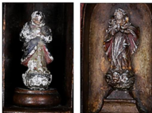
**Figure 1.** Corroded polychrome lead sculptures from the Oratory Museum, Ouro Preto (Minas Gerais, Brazil). The white areas correspond to corrosion products.
