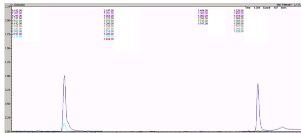
Figure S3. Chromatograms of target ions in real sample (week 4). Signal in ca. 3.25 min is carbendazim.
