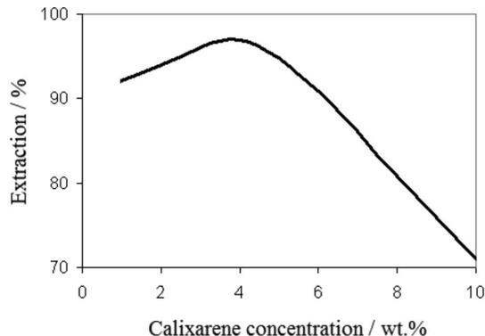
**Figure 5.** Effect of calixarene concentration on the extraction efficiency of dioxin in the ELM process.
