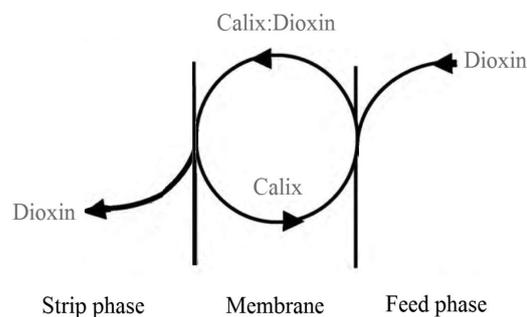
Figure 3. Facilitated transport mechanism of dioxin in ELM.
