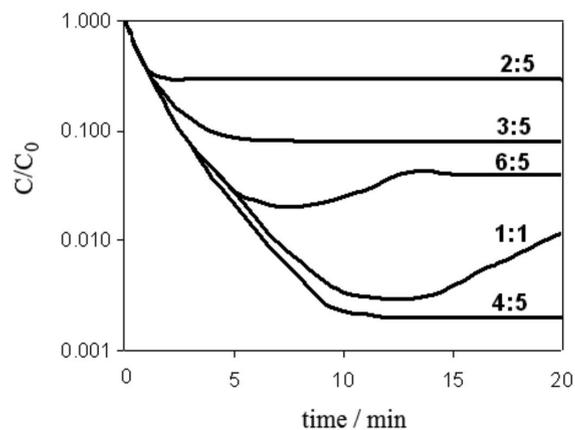
**Figure 6.** Effect of phase ratio on the extraction efficiency of dioxin in the ELM process.
