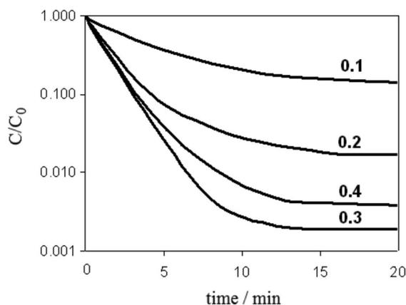
**Figure 7.** Effect of treat ratio on the extraction efficiency of dioxin in the ELM process.
