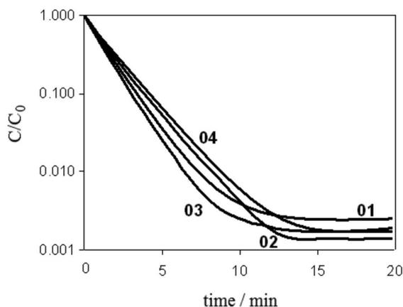
**Figure 4.** Effect of calixarene type on the extraction efficiency of dioxin in the ELM process.
