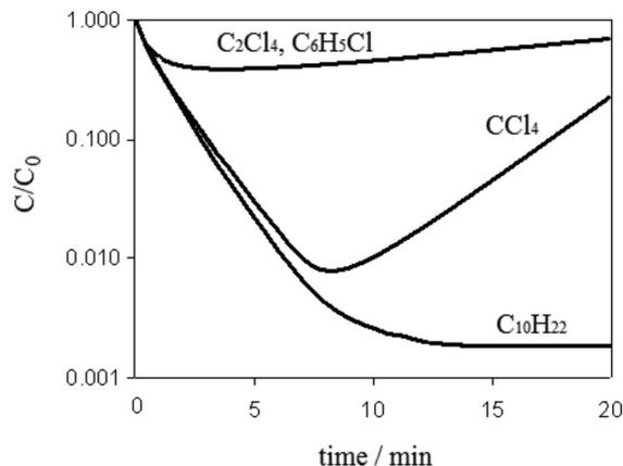
**Figure 8.** Effect of diluent (membrane) type on the extraction efficiency of dioxin in the ELM process.
