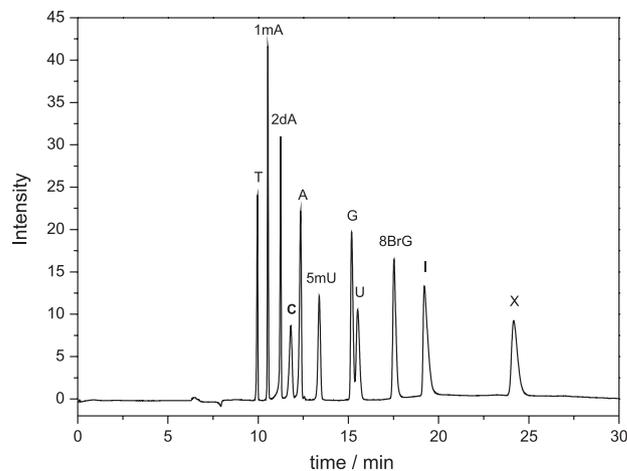
**Figure 3.** Electropherogram obtained under optimized analysis conditions, as follows: BGE composed by 20 mmol L<sup>-1</sup> borate at pH 9.20, 260 mmol L<sup>-1</sup> SDS and 17% methanol; 25 kV; 20 °C; L<sub>r</sub>: 60 cm, L<sub>eff</sub>: 52 cm, i.d.: 50 μm; 0.500 mmol L<sup>-1</sup> solution of nucleoside standards.
