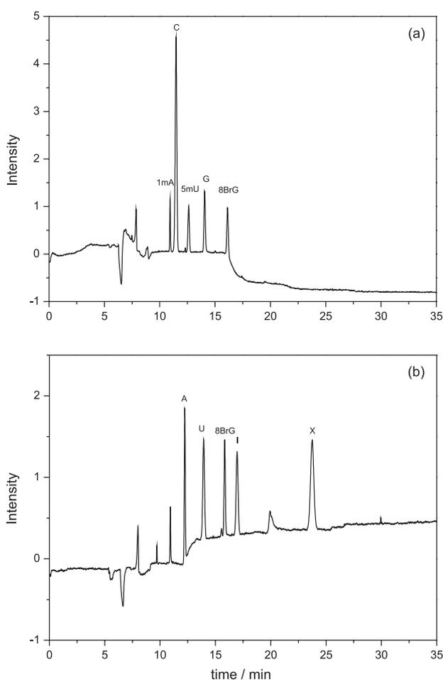
**Figure 4.** Electropherograms of the analyzed sample with analytes concentration referent to the middle point of the analytical curves: (a) 1mA, C, 5mU, G and 8BrG (internal standard); and (b) A, U, I, X and 8BrG. The conditions of analysis are the same presented in Figure 3, except for nucleosides concentration.
