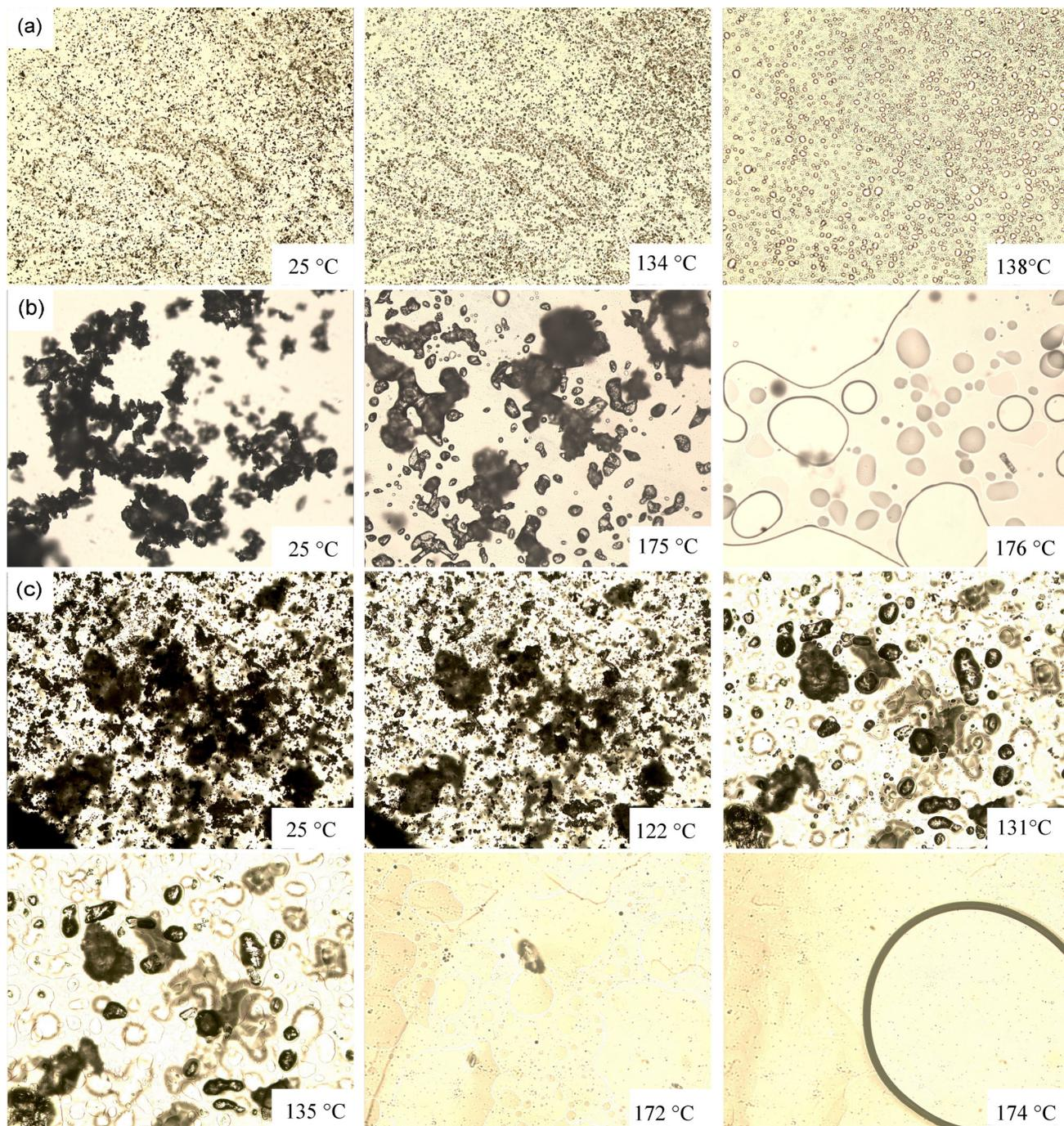
**Figure 4.** TOA images at 100× magnification of (a) efavirenz, (b) lamivudine and (c) mixture. Three images in different temperatures were shown for each pure drug and six for the mixture.
