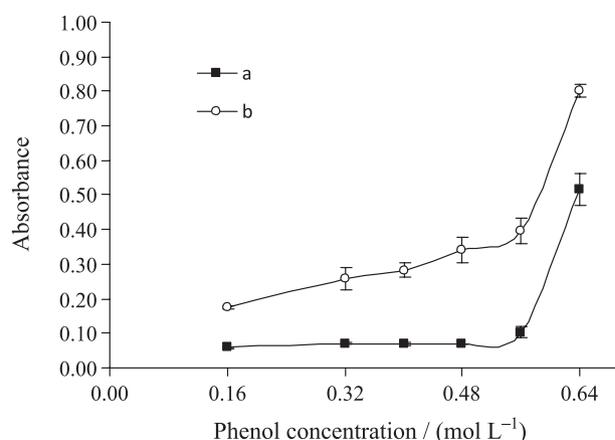
**Figure 3.** Effect of the phenol concentration. Blank solution (a);  $160 \mu\text{mol L}^{-1}$  of allantoin standard solution (b). Results are average of 5 consecutive measurements.
