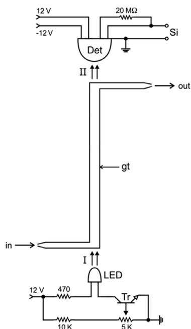
**Figure 1.** Diagram of the photometer. Tr = transistor (BC547); LED = light emitting diode,  $\lambda_{\max} = 660 \text{ nm}$ ; gt = flow cell body, borosilicate glass tube, inner diameter of 1.2 mm; I = radiation beam emitted by the LED; II = radiation beam after cross the flow cell window; Det = photodetector (OPT301); Si = generated sinal (mV); in and out = input and output of solution, respectively.
