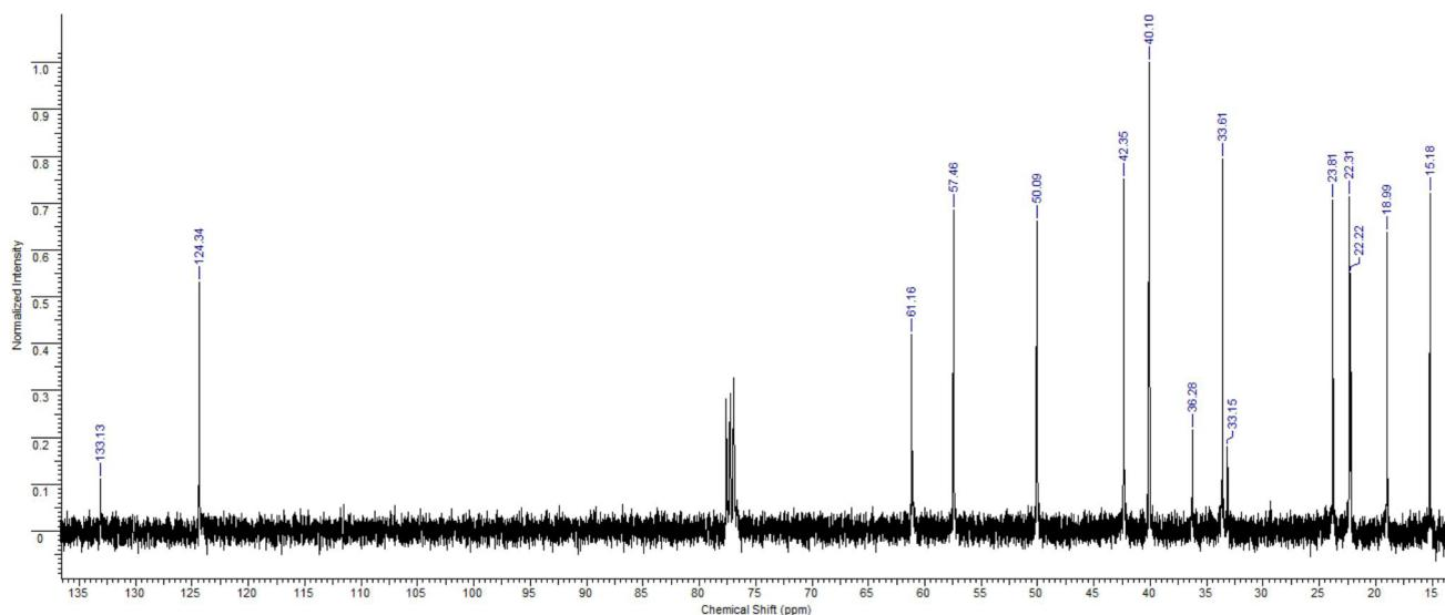
**Figure S4.**  $^{13}\text{C}$  NMR ( $\text{CDCl}_3$ , 100 MHz) spectrum of drimenol.
