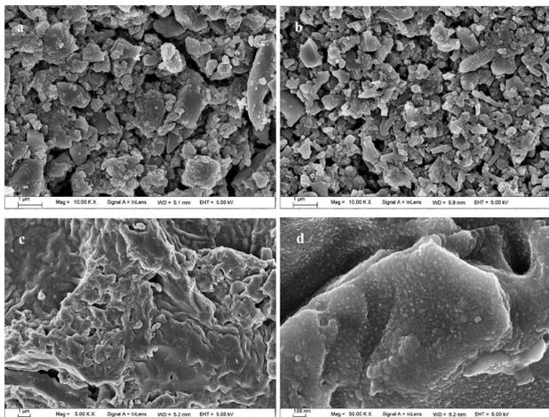
**Figure 6.** SEM images of Ni/AC particle electrode: a: untreated, b: after oxidation, c and d: after plating.
