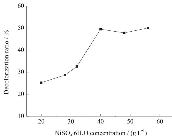
**Figure 2.** Effect of  $\text{NiSO}_4 \cdot 6\text{H}_2\text{O}$  concentration on the decolorization ratio of Ni/AC particle electrode. Experimental conditions:  $27 \text{ g L}^{-1} \text{ NaH}_2\text{PO}_2 \cdot \text{H}_2\text{O}$ ,  $50 \text{ }^\circ\text{C}$ , 20 min plating time, 10.0 g particle electrode dose,  $12 \text{ g L}^{-1} \text{ Na}_2\text{SO}_4$  and 6 V cell voltage.
