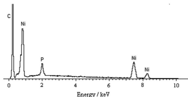
**Figure 8.** EDS spectrum of plated Ni/AC particle electrode.
