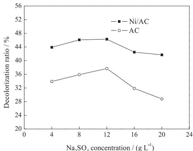
**Figure 10.** Effect of Na<sub>2</sub>SO<sub>4</sub> concentration on the decolorization ratio. Experimental conditions: 40 g L<sup>-1</sup> NiSO<sub>4</sub>·6H<sub>2</sub>O, 27 g L<sup>-1</sup> NaH<sub>2</sub>PO<sub>2</sub>·H<sub>2</sub>O, 50 °C, 20 min plating time, 10.0 g particle electrode dose and 6 V cell voltage.
