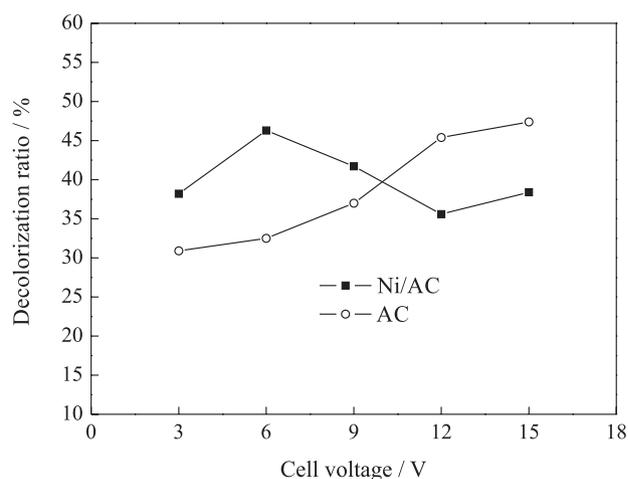
**Figure 11.** Effect of cell voltage on the decolorization ratio. Experimental conditions: 40 g L<sup>-1</sup> NiSO<sub>4</sub>·6H<sub>2</sub>O, 27 g L<sup>-1</sup> NaH<sub>2</sub>PO<sub>2</sub>·H<sub>2</sub>O, 50 °C, 20 min plating time, 10.0 g particle electrode dose and 12 g L<sup>-1</sup> Na<sub>2</sub>SO<sub>4</sub>.
