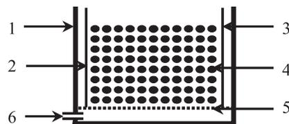
**Figure 1.** Schematic diagram of a cell with a three-dimensional electrode. 1: support; 2: anode; 3: cathode; 4: particle electrode; 5: micropore plate; 6: compressed air.
