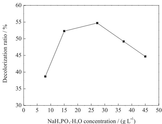
**Figure 3.** Effect of NaH<sub>2</sub>PO<sub>2</sub>·H<sub>2</sub>O concentration on the decolorization ratio of Ni/AC particle electrode. Experimental conditions: 40 g L<sup>-1</sup> NiSO<sub>4</sub>·6H<sub>2</sub>O, 50 °C, 20 min plating time, 10.0 g particle electrode dose, 12 g L<sup>-1</sup> Na<sub>2</sub>SO<sub>4</sub> and 6 V cell voltage.
