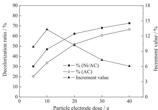
**Figure 9.** Effect of particle electrode dose on the decolorization ratio. Experimental conditions: 40 g L<sup>-1</sup> NiSO<sub>4</sub>·6H<sub>2</sub>O, 27 g L<sup>-1</sup> NaH<sub>2</sub>PO<sub>2</sub>·H<sub>2</sub>O, 50 °C, 20 min plating time, 12 g L<sup>-1</sup> Na<sub>2</sub>SO<sub>4</sub> and 6 V cell voltage.
