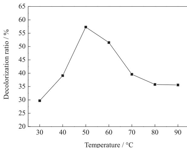
**Figure 4.** Effect of plating temperature on the decolorization ratio of Ni/AC particle electrode. Experimental conditions: 40 g L<sup>-1</sup> NiSO<sub>4</sub>·6H<sub>2</sub>O, 27 g L<sup>-1</sup> NaH<sub>2</sub>PO<sub>2</sub>·H<sub>2</sub>O, 20 min plating time, 10.0 g particle electrode dose, 12 g L<sup>-1</sup> Na<sub>2</sub>SO<sub>4</sub> and 6 V cell voltage.
