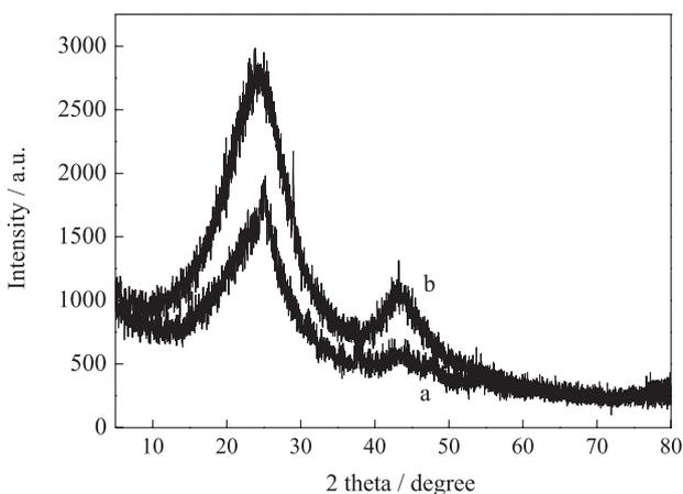
**Figure 7.** X-ray diffraction pattern of Ni/AC particle electrode: a: before plating, and b: after plating.
