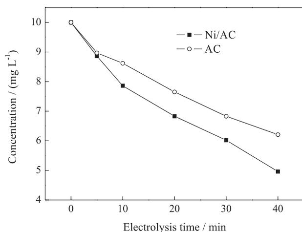
**Figure 12.** Effect of electrolysis time on the concentration. Experimental conditions: 40 g L<sup>-1</sup> NiSO<sub>4</sub>·6H<sub>2</sub>O, 27 g L<sup>-1</sup> NaH<sub>2</sub>PO<sub>2</sub>·H<sub>2</sub>O, 50 °C, 20 min plating time, 10.0 g particle electrode dose, 12 g L<sup>-1</sup> Na<sub>2</sub>SO<sub>4</sub> and 6 V cell voltage.
