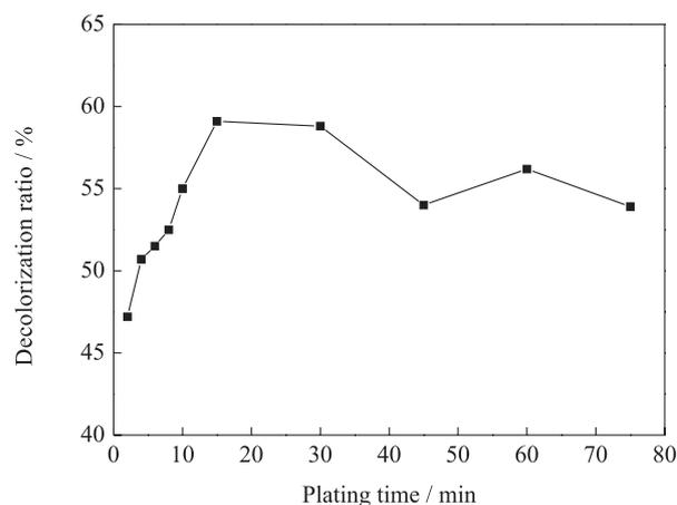
**Figure 5.** Effect of plating time on the decolorization ratio of Ni/AC particle electrode. Experimental conditions: 40 g L<sup>-1</sup> NiSO<sub>4</sub>·6H<sub>2</sub>O, 27 g L<sup>-1</sup> NaH<sub>2</sub>PO<sub>2</sub>·H<sub>2</sub>O, 50 °C, 10.0 g particle electrode dose, 12 g L<sup>-1</sup> Na<sub>2</sub>SO<sub>4</sub> and 6 V cell voltage.
