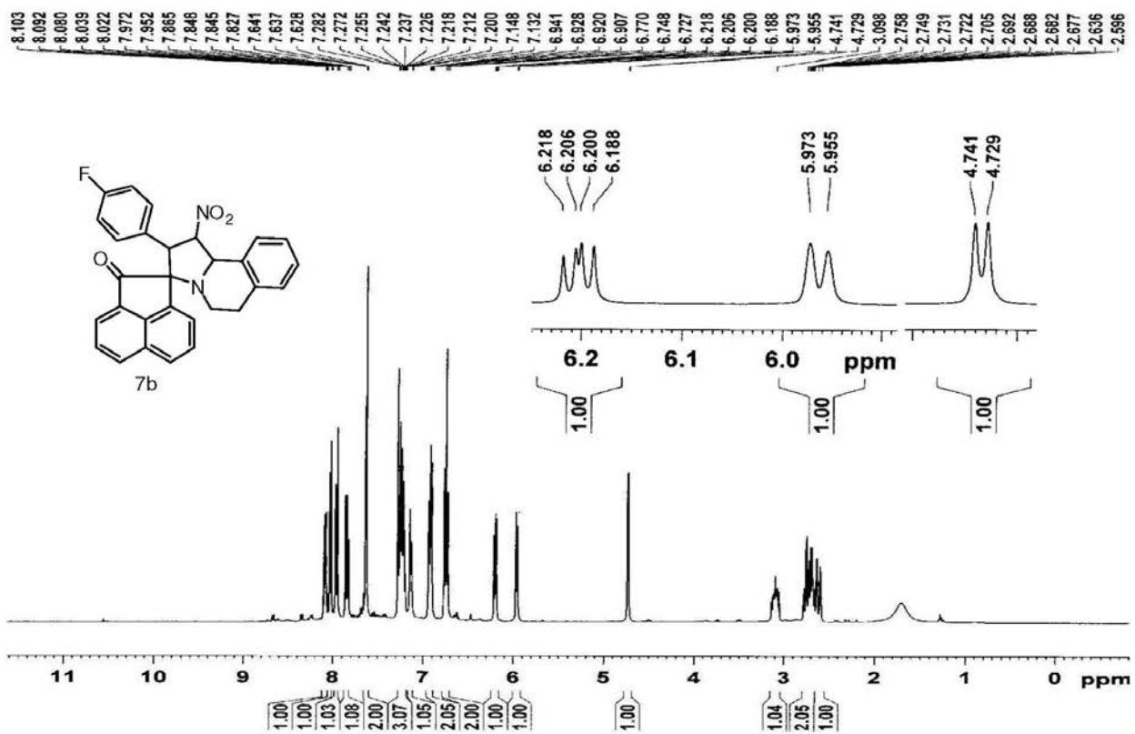
Figure S46. <sup>1</sup>H NMR (400 MHz,  $\text{CDCl}_3$ ) of (7b).
