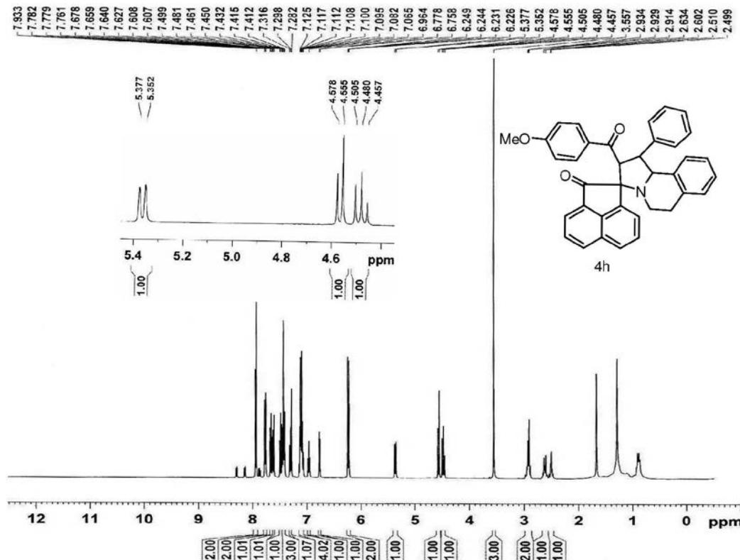
**Figure S24.** <sup>1</sup>H NMR (400 MHz, CDCl<sub>3</sub>) of (**4h**).
