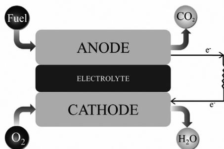
**Figure 1.** Representative scheme of the hydrocarbon fuel cell operation mechanism.
