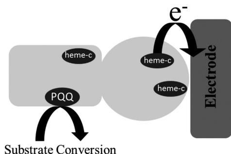
**Figure 6.** Illustration of the electron transfer mechanism in a PQQ-dependent enzyme.<sup>120</sup>
