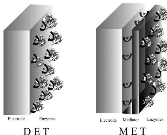
**Figure 4.** Types of electron transfer processes between enzymes and electrode surfaces in enzymatic biofuel cells.
