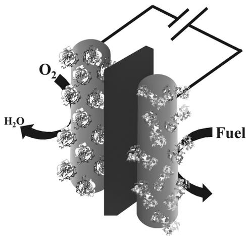
**Figure 2.** Schematic representation of an enzymatic biofuel cell.
