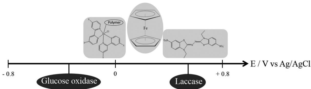
**Figure 5.** Redox potential range of some of the most often employed metal-based mediators and of the oxidoreductase enzymes glucose oxidase and laccase.
