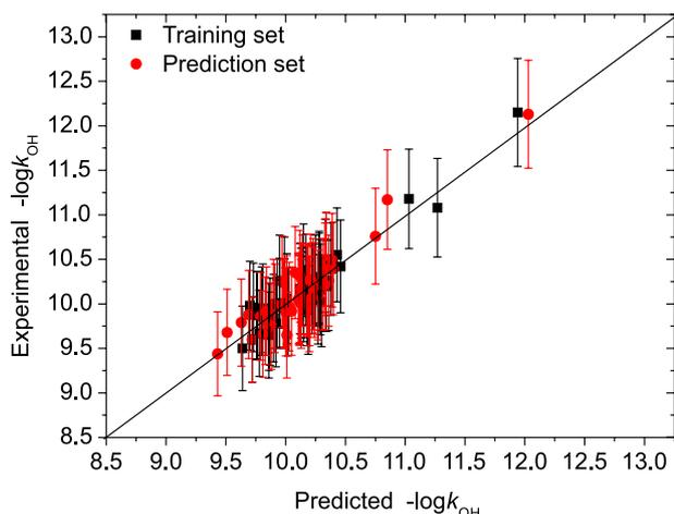
**Figure 4.** Predicted vs. experimental  $-\log k_{\text{OH}}$  values from the MLR model for  $-\log k_{\text{OH}}$ . Error bars represent the typical 5% error in the measurement of the rate constants.
