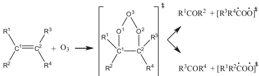
**Scheme 1.** Degradation reaction process of alkenes with  $O_3$ .
