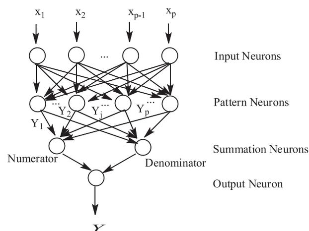
Figure 1. Structure model of a GRNN model.
