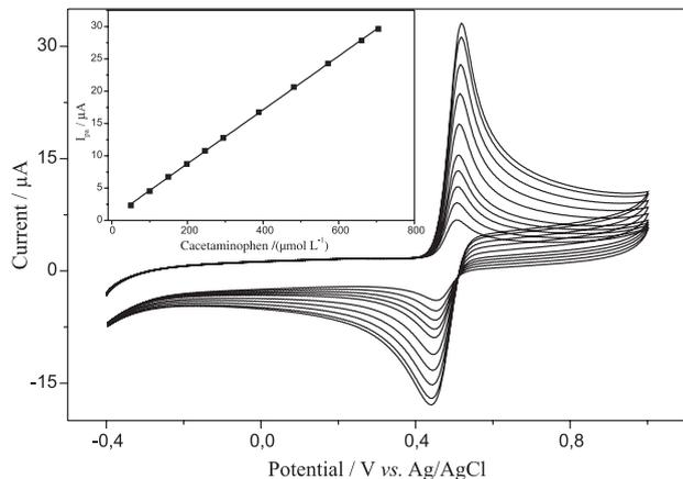
**Figure 6.** Cyclic voltammograms of acetaminophen as a function of concentration in the range of 50-700 μmol L<sup>-1</sup> in 0.1 mol L<sup>-1</sup> acetate buffer solution (pH 4.75) at the ESPE. Inset: Anodic peak currents vs. acetaminophen concentration.
