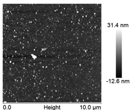
**Figure 3.** AFM image of a  $\{Mn-TPyP[Ru(dppb)]_4(\mu Cl_3)_2\}_{2n}^{(4n2+)+}$  film deposited on ITO electrode surface.
