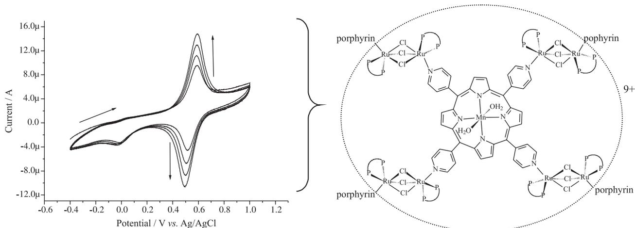
**Figure 2.** (A) Repetitive voltammograms (4 cycles) of  $\{Mn-TPyP(H_2O)_2[RuCl_3(dppb)]_4\}PF_6$  and (B) electropolymerized supramolecular tetraruthenated porphyrins,  $0.1 \text{ mmol L}^{-1} \{Mn-TPyP[Ru(dppb)]_4(\mu Cl_3)_2\}_{2n}^{(4n2+)+}$ ,  $0.1 \text{ mol L}^{-1}$  TBAH,  $CH_2Cl_2$ , glassy carbon as working electrode, scan rate =  $100 \text{ mV s}^{-1}$ .
