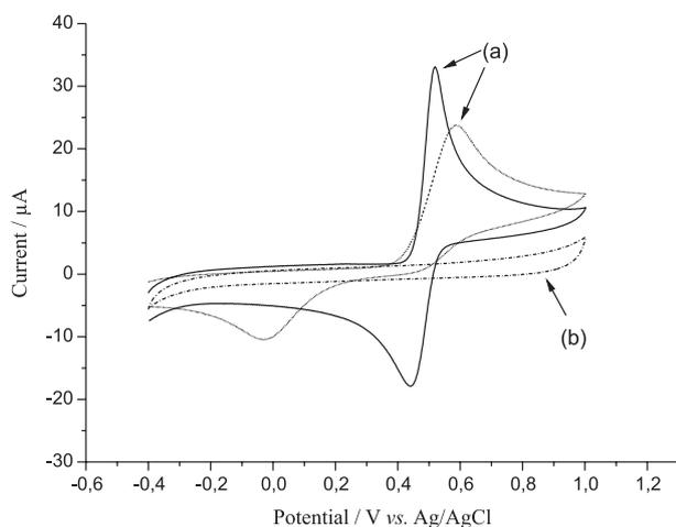
**Figure 4.** (a) Cyclic voltammograms of  $0.25 \text{ mmol L}^{-1}$  acetaminophen in  $0.1 \text{ mol L}^{-1}$  acetate buffer solution (pH 4.75) at the ESPE (solid line); GC electrode (dot line). (b) Cyclic voltammogram at the ESPE in  $0.1 \text{ mol L}^{-1}$  acetate buffer solution (pH 4.75).
