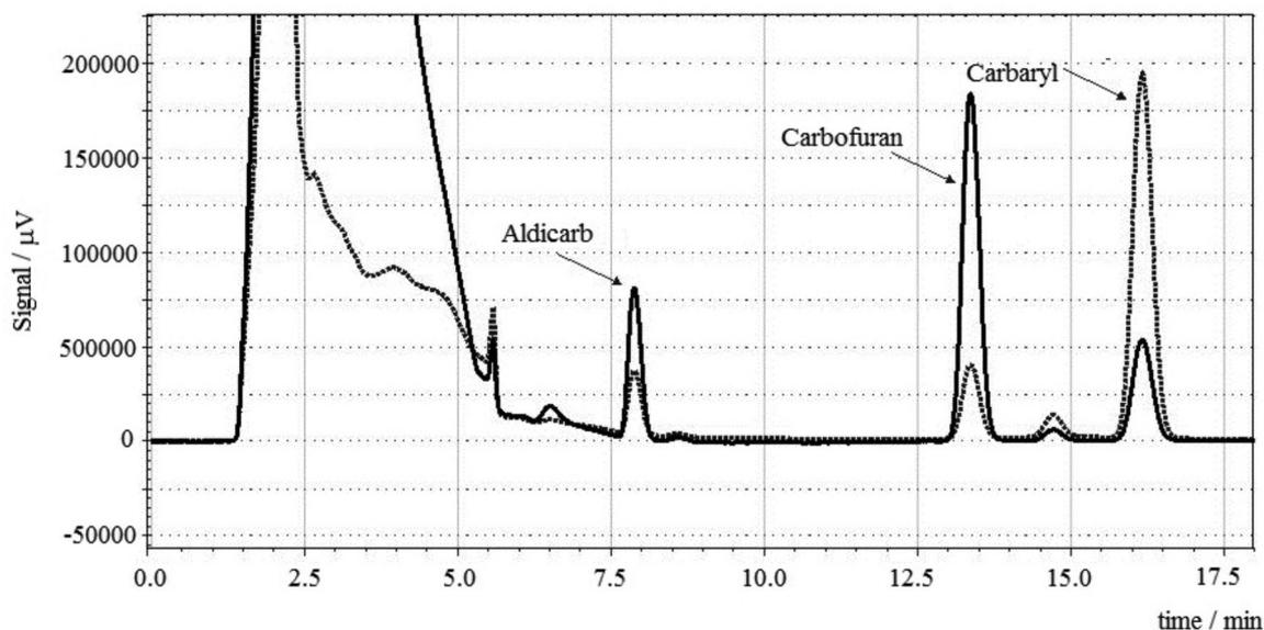
**Figure 6.** Chromatograms of one extract obtained from grape juice samples to which the commercial carbamates were added and analyzed at 195 (—) and 213 nm (-----).
