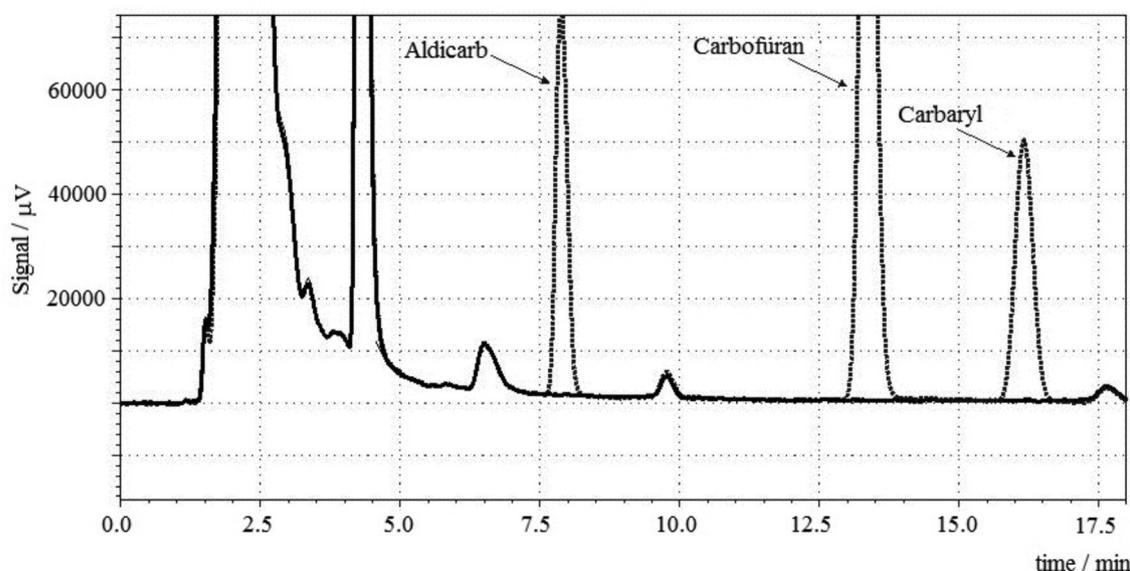
**Figure 5.** Chromatograms of an extract obtained from the chocolate milk beverage free of active principles (—) and of a chocolate milk beverage extract fortified with 2500.0  $\mu\text{g L}^{-1}$  of the carbamates (-----).
