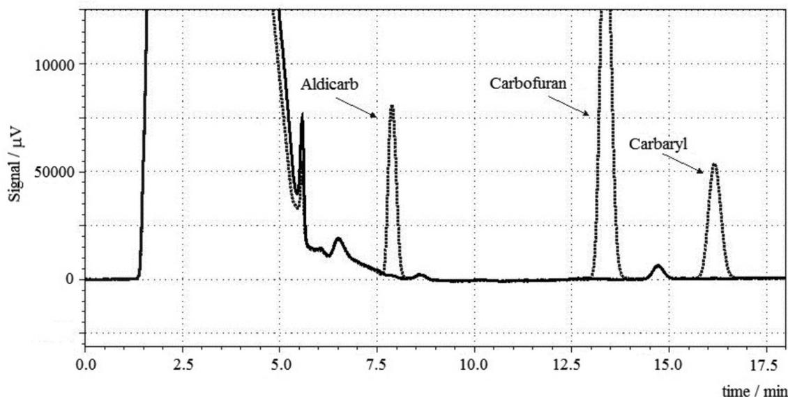
**Figure 4.** Chromatograms of an extract obtained from grape juice free of active principles (—) and of a grape juice extract fortified with 2500.0  $\mu\text{g L}^{-1}$  of the carbamates (----).
