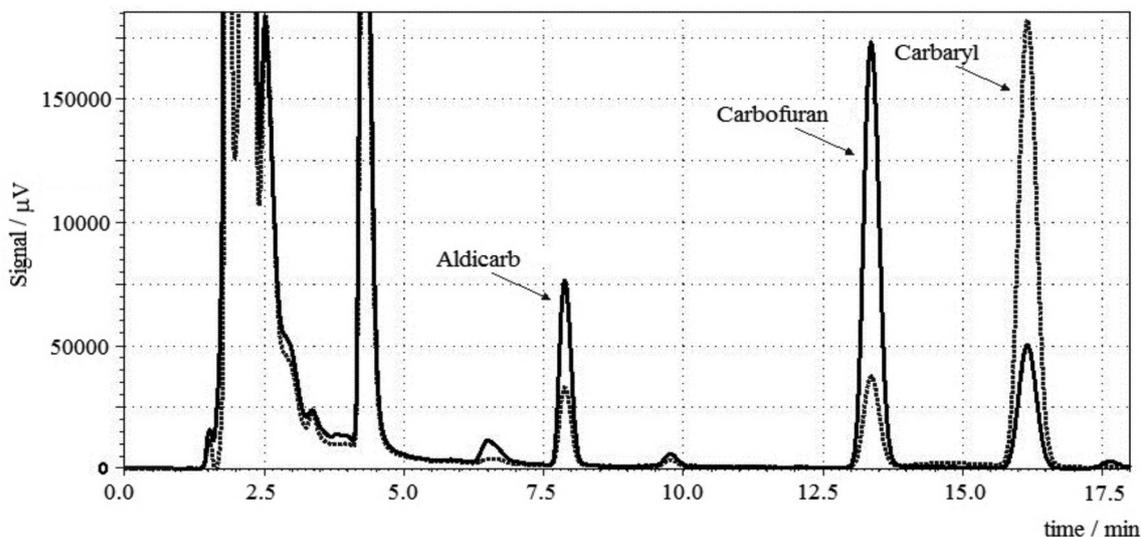
**Figure 7.** Chromatograms of one extract obtained from the chocolate milk beverage samples to which the commercial carbamates were added and analyzed at 195 (—) and 213 nm (-----).
