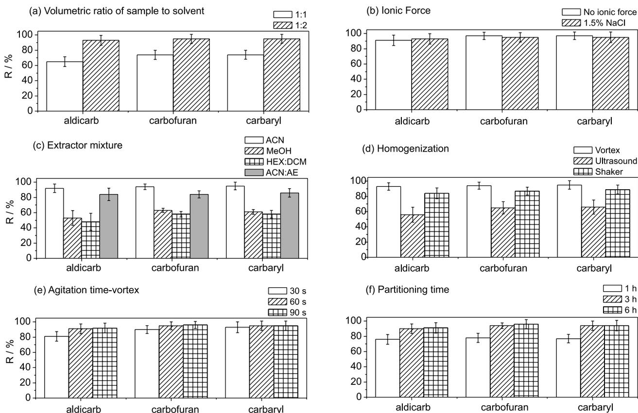
**Figure 3.** Extraction percentages obtained in optimization of the LLE-LTP technique for pesticides in chocolate milk: (a) volumetric ratio of sample to solvent, (b) ionic force, (c) extractor mixture, (d) homogenization, (e) agitation time and (f) partitioning time.
