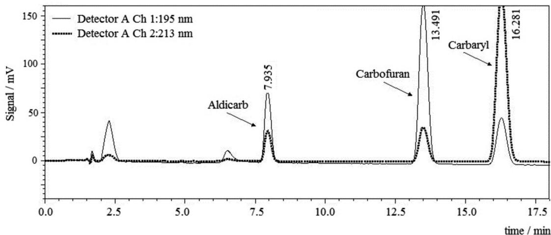
**Figure 1.** Chromatograms of a standard solution of 5.0  $\text{mg L}^{-1}$  of aldicarb ( $t_R = 7.935$  min), carbofuran ( $t_R = 13.491$  min) and carbaryl ( $t_R = 16.281$  min) in acetonitrile.
