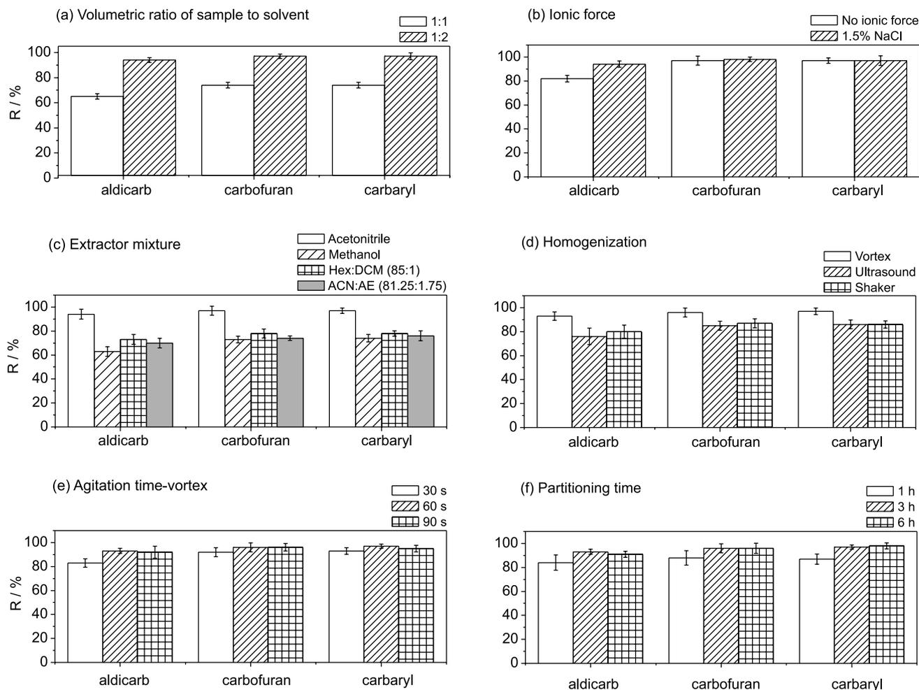
**Figure 2.** Extraction percentages obtained in optimization of the LLE-LTP technique for pesticides in grape juice: (a) volumetric ratio of sample to solvent, (b) ionic force, (c) extractor mixture, (d) homogenization, (e) agitation time and (f) partitioning time.
