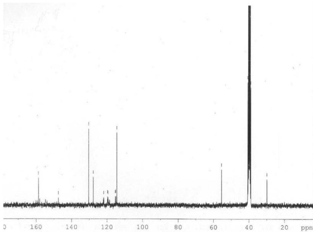
**Figure S52.** <sup>13</sup>C NMR (75 MHz, DMSO-*d*<sub>6</sub>) spectrum of **6h**.
