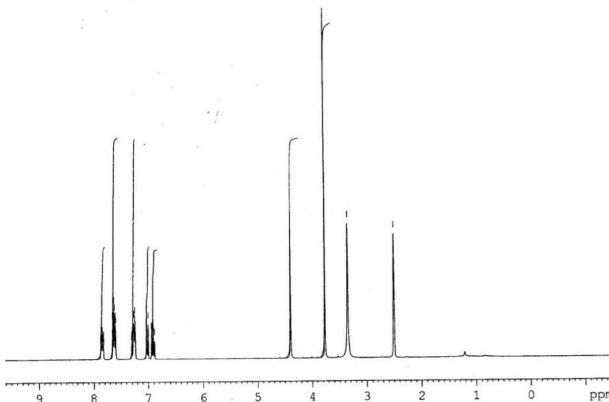
Figure S43.  $^1\text{H}$  NMR (300 MHz,  $\text{DMSO}-d_6$ ) spectrum of **6d**.
