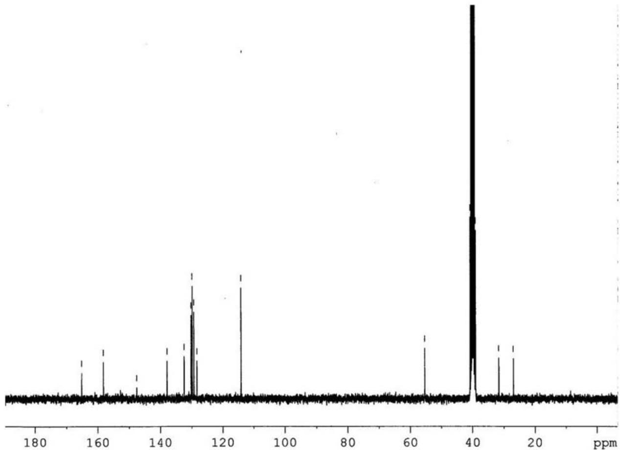
**Figure S32.**  $^{13}\text{C}$  NMR (75 MHz,  $\text{DMSO}-d_6$ ) spectrum of **6a**.
