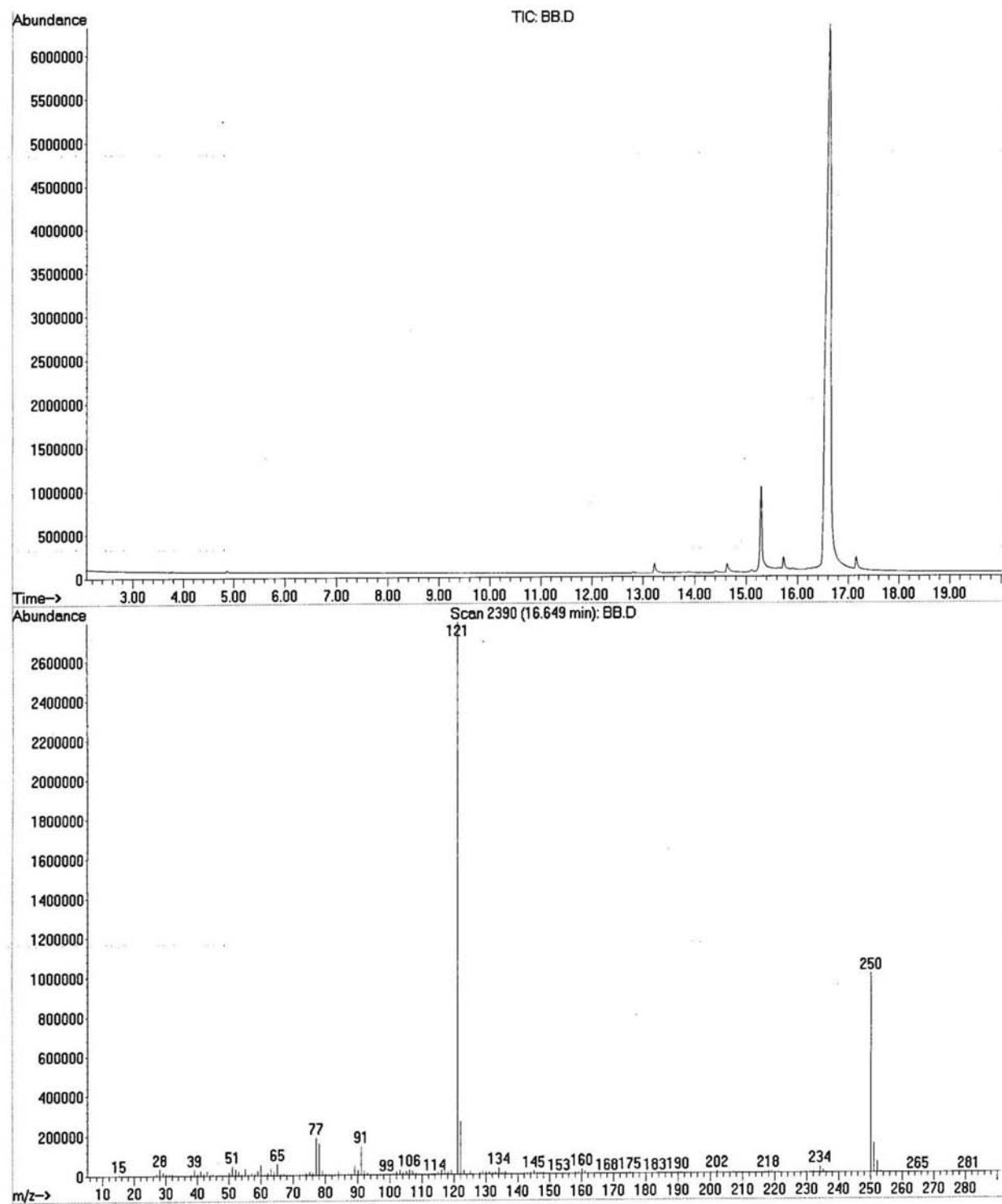
Figure S15. GC MS spectrum of 5a.
