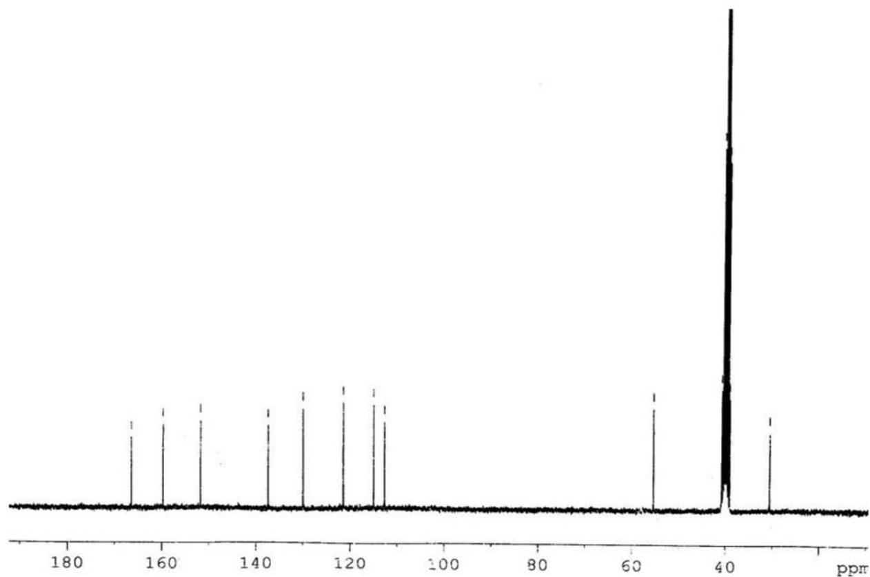
**Figure S22.**  $^{13}\text{C}$  NMR (75 MHz,  $\text{DMSO}-d_6$ ) spectrum of **5c**.
