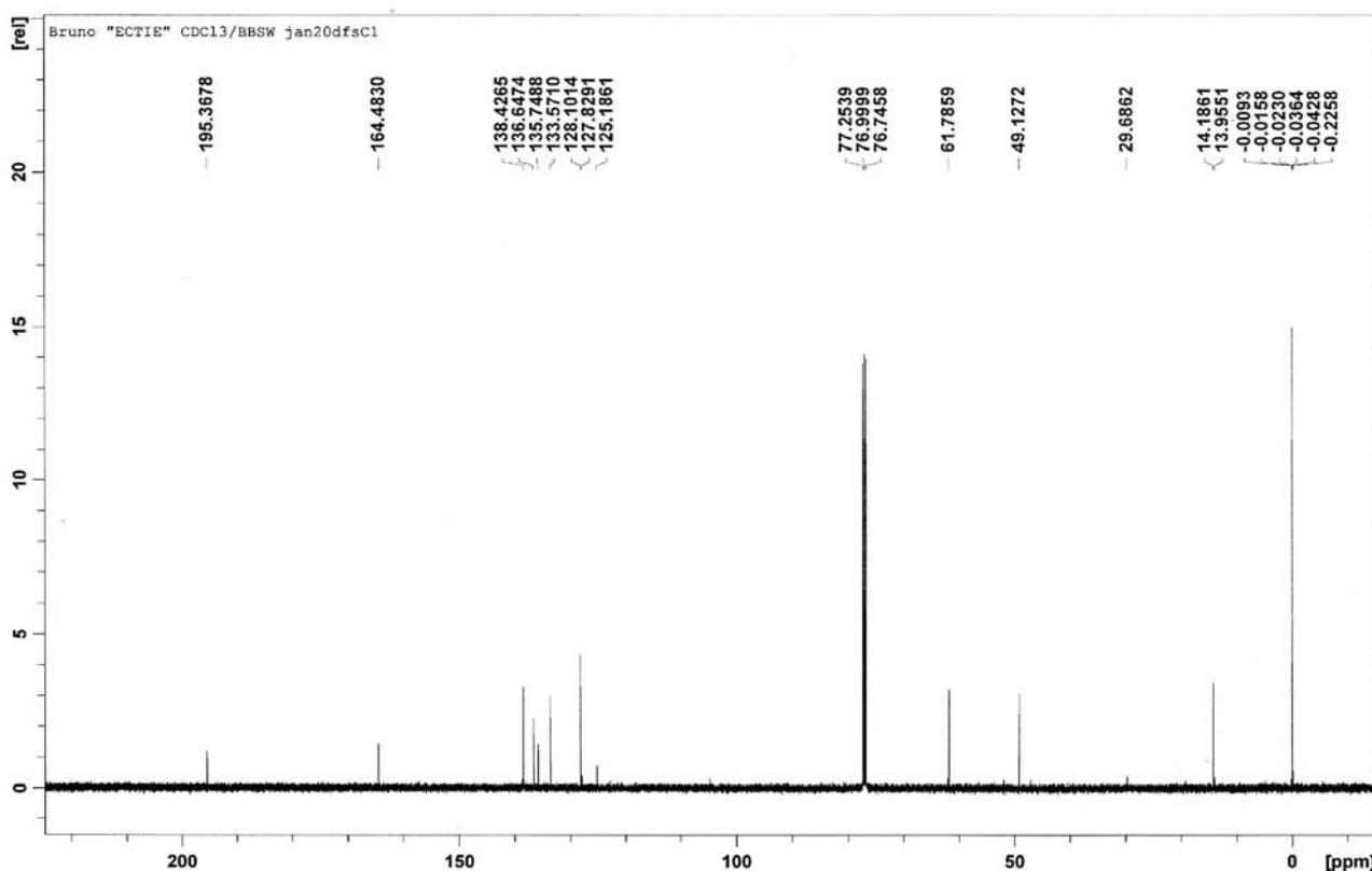
**Figure S52.**  $^{13}\text{C}$  NMR spectrum ( $\text{CDCl}_3$ , 125 MHz) of ethyl (*E*)-2-chloroacetyl-3-(2'-thiofuranyl)propenoate (*E*-3f).
