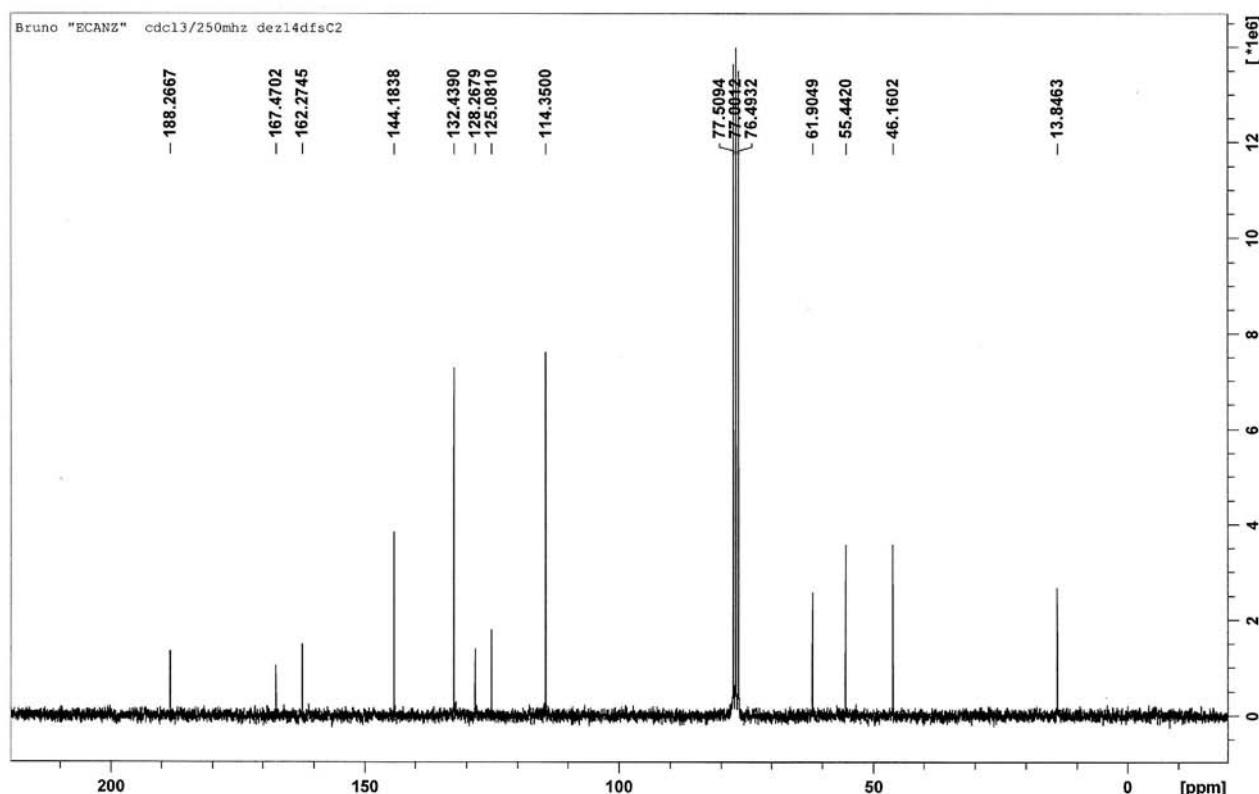
**Figure S27.** <sup>13</sup>C NMR spectrum (CDCl<sub>3</sub>, 62.5 MHz) of ethyl (Z)-2-chloroacetyl-3-(4'-methoxyphenyl)propenoate (Z-3c).
