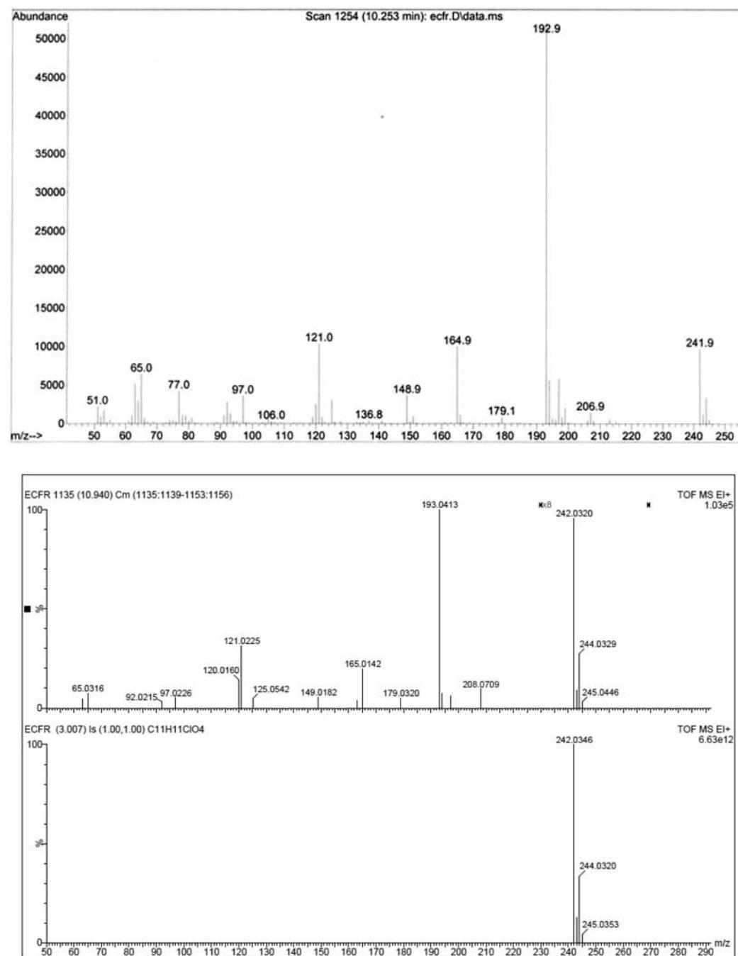
**Figure S50.** MS and HRMS (EI) spectra of ethyl (Z)-2-chloroacetyl-3-(2'-furanyl)propenoate (*Z*-3e).
