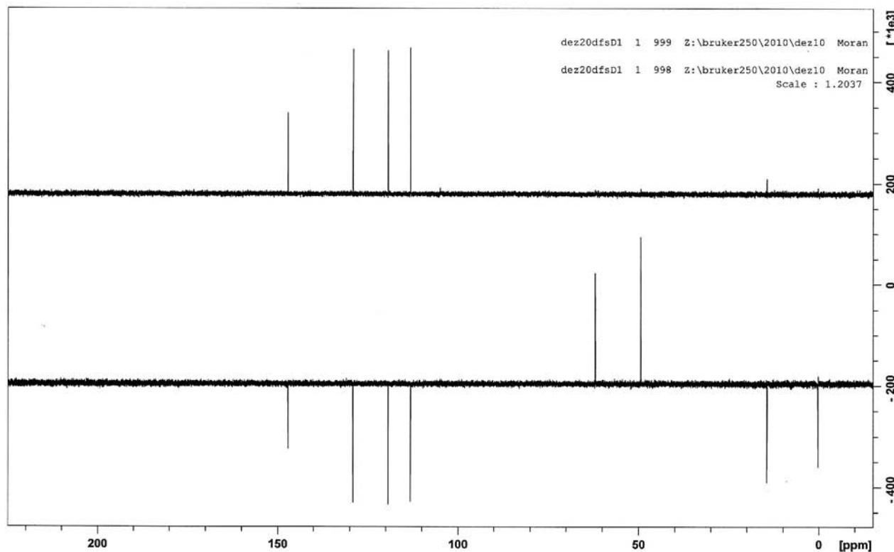
**Figure S43.** DEPT-90 and DEPT-135 spectra ( $\text{CDCl}_3$ , 125 MHz) of ethyl (*E*)-2-chloroacetyl-3-(2'-furanyl)propenoate (*E*-3e).
