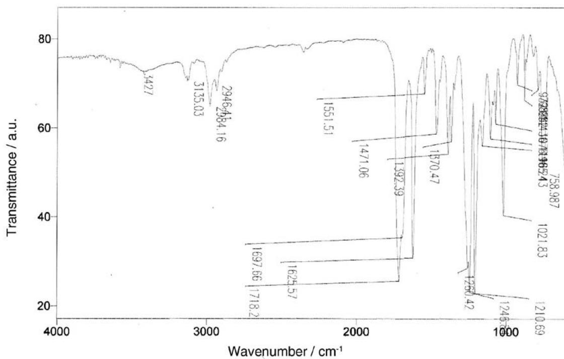
**Figure S44.** IR spectrum (film) of ethyl (E)-2-chloroacetyl-3-(2'-furanyl)propenoate (*E*-3e).
