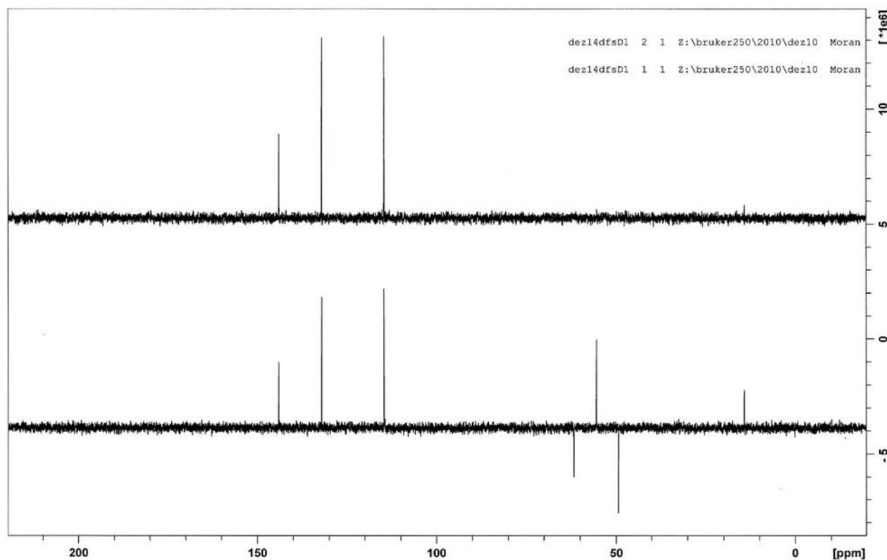
**Figure S23.** DEPT-90 and DEPT-135 spectra ( $\text{CDCl}_3$ , 62.5 MHz) of ethyl (*E*)-2-chloroacetyl-3-(4'-methoxyphenyl)propenoate (*E*-**3c**).
