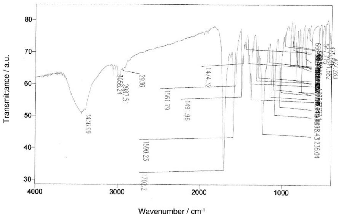
**Figure S19.** IR spectrum (KBr) of ethyl (Z)-2-chloroacetyl-3-(4'-chlorophenyl)propenoate (**Z-3b**).
