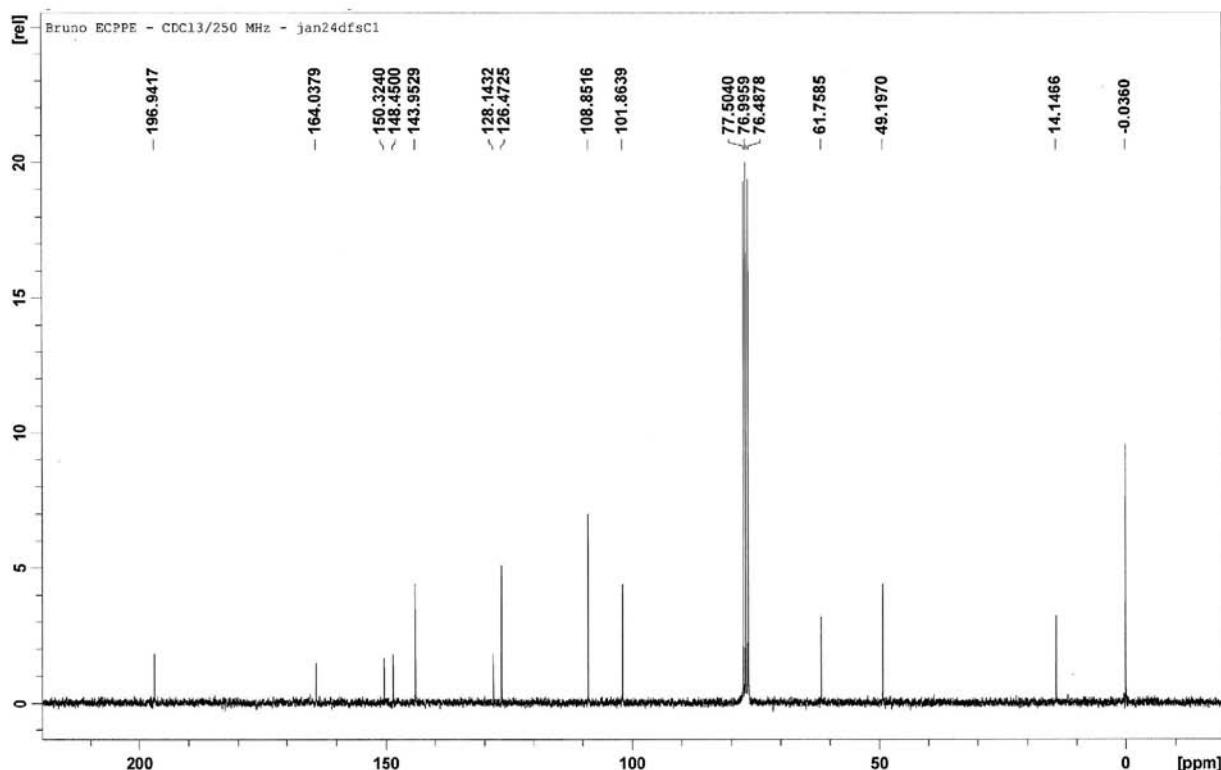
**Figure S32.**  $^{13}\text{C}$  NMR spectrum ( $\text{CDCl}_3$ , 62.5 MHz) of ethyl (*E*)-2-chloroacetyl-3-(3',4'-methylenedioxyphenyl)propenoate (*E*-3d).
