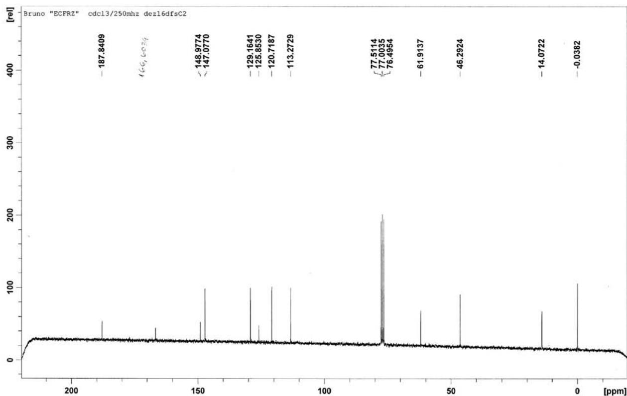
**Figure S47.**  $^{13}\text{C}$  NMR spectrum ( $\text{CDCl}_3$ , 62.5 MHz) of ethyl (Z)-2-chloroacetyl-3-(2'-furanyl)propenoate (Z-3e).
