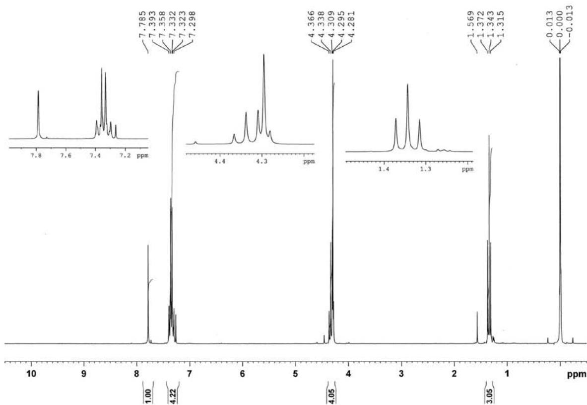
**Figure S11.**  $^1\text{H}$  NMR spectrum ( $\text{CDCl}_3$ , 250 MHz) of ethyl (*E*)-2-chloroacetyl-3-(4'-chlorophenyl)propenoate (*E*-3b).
