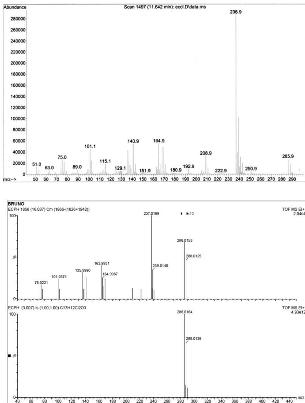
**Figure S15.** MS and HRMS (EI) spectra of ethyl (E)-2-chloroacetyl-3-(4'-chlorophenyl)propenoate (*E*-3b).
