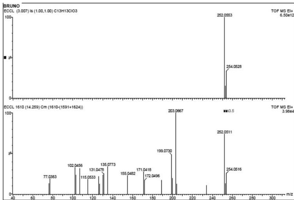
**Figure S5.** MS and HRMS (EI) spectra of ethyl (*E*)-2-chloroacetyl-3-phenylpropenoate (*E*-3a).
