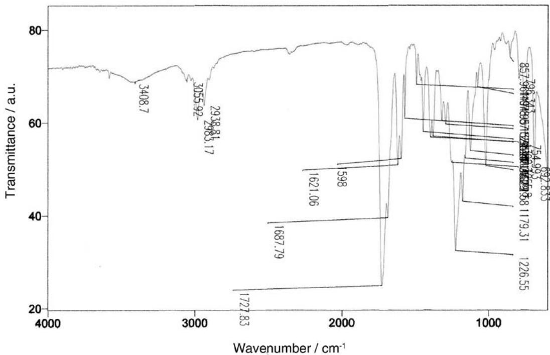
**Figure S9.** IR spectrum (film) of ethyl (Z)-2-chloroacetyl-3-phenylpropenoate (Z-3a).
