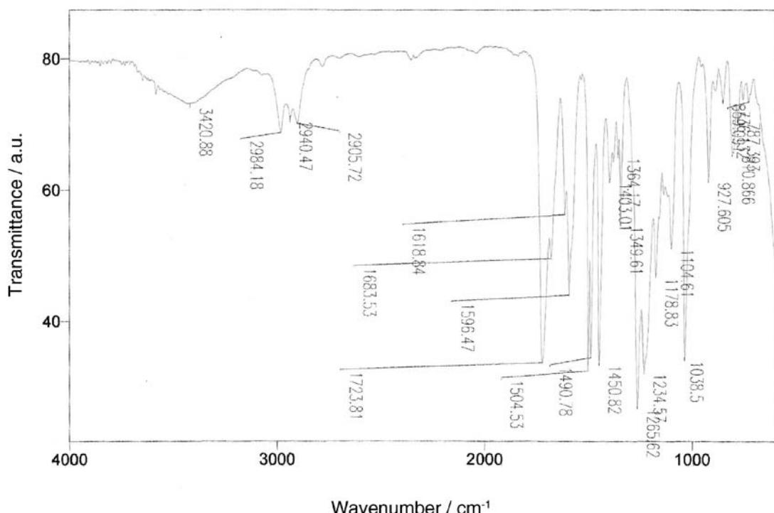
**Figure S39.** IR spectrum (film) of ethyl (Z)-2-chloroacetyl-3-(3',4'-methylenedioxyphenyl)propenoate (Z-3d).
