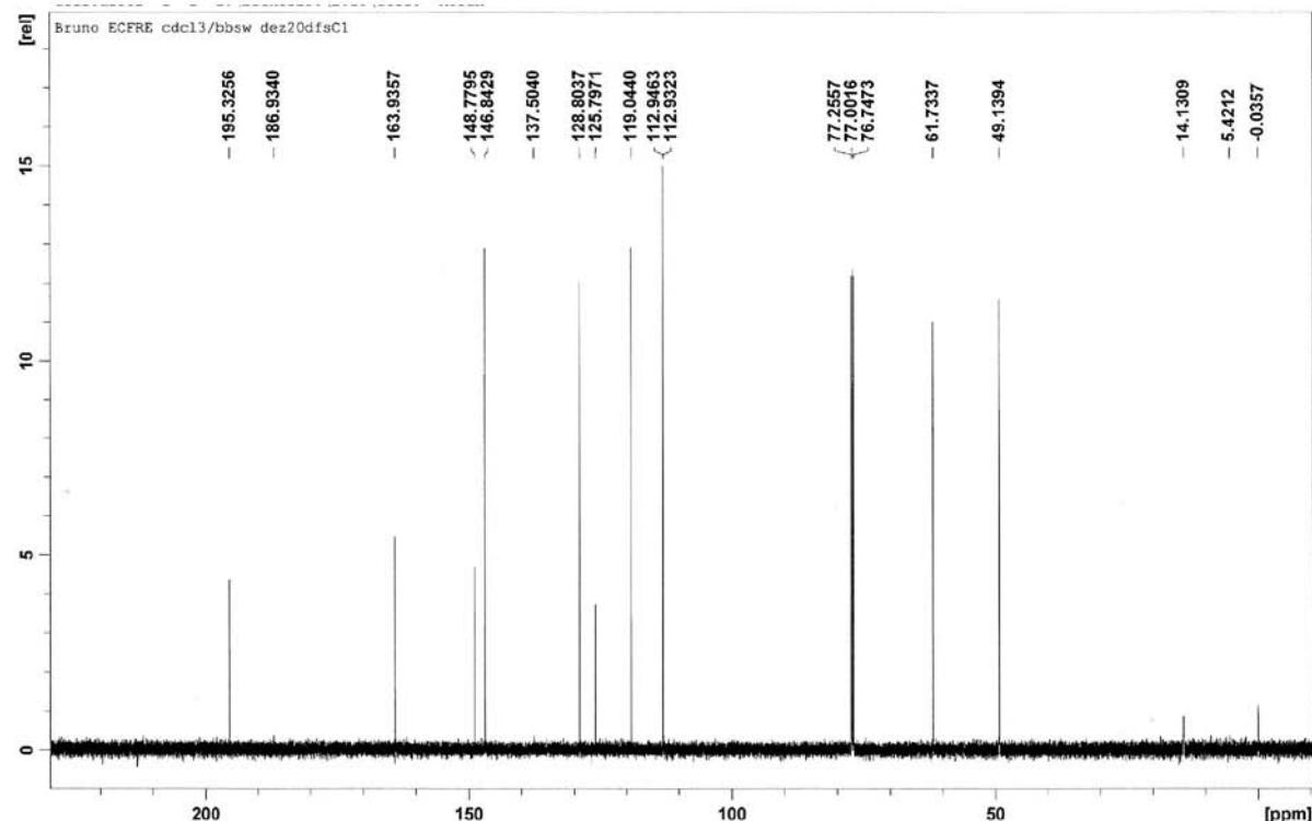
**Figure S42.**  $^{13}\text{C}$  NMR spectrum ( $\text{CDCl}_3$ , 125 MHz) of ethyl (*E*)-2-chloroacetyl-3-(2'-furanyl)propenoate (*E*-3e).
