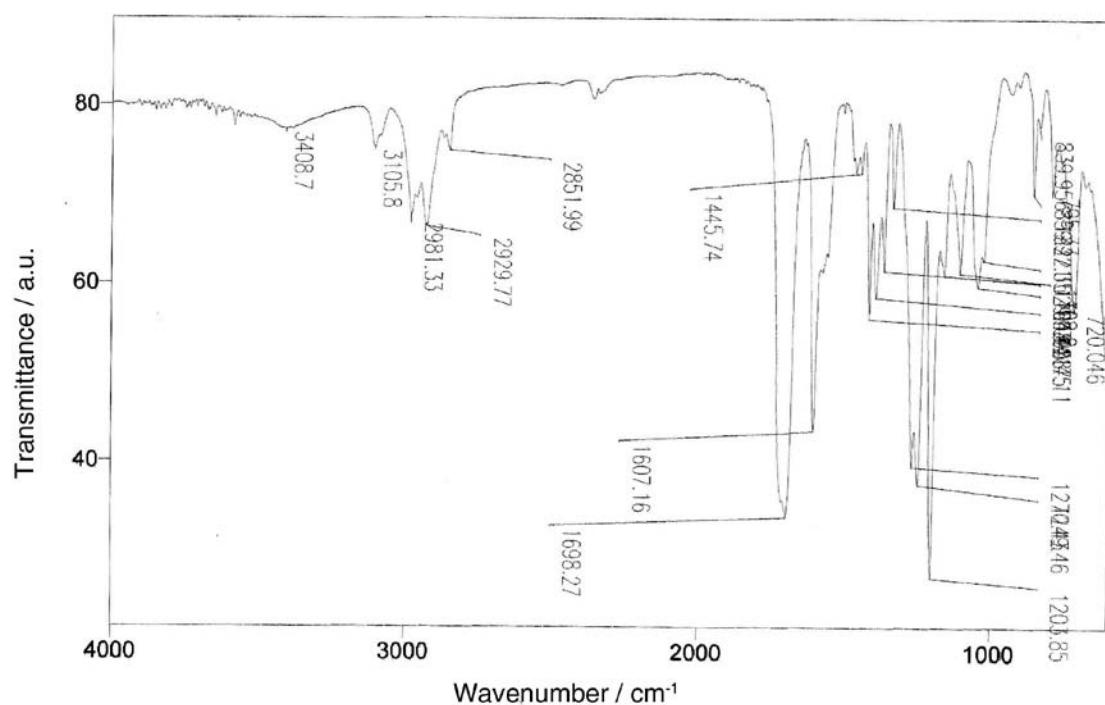
**Figure S54.** IR spectrum (film) of ethyl (E)-2-chloroacetyl-3-(2'-thiofuranyl)propenoate (*E*-3f).
