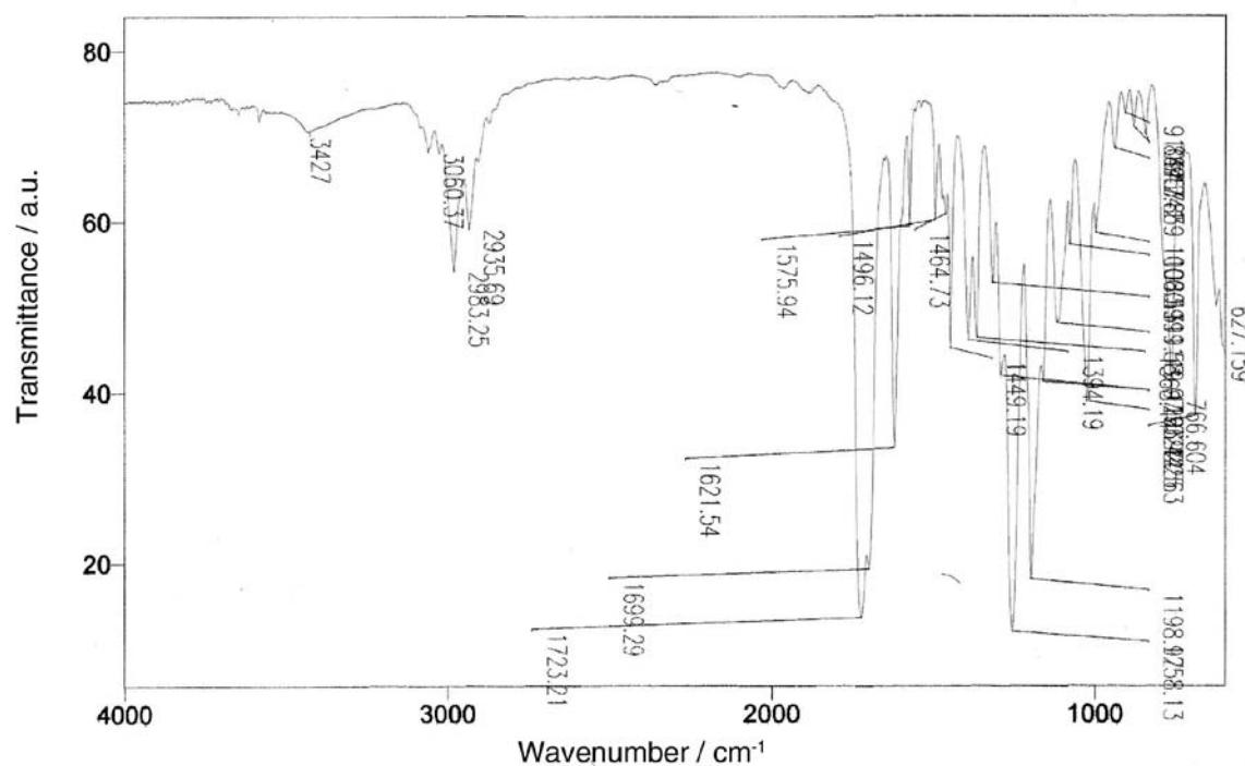
**Figure S4.** IR spectrum (film) of ethyl (*E*)-2-chloroacetyl-3-phenylpropenoate (*E*-3a).
