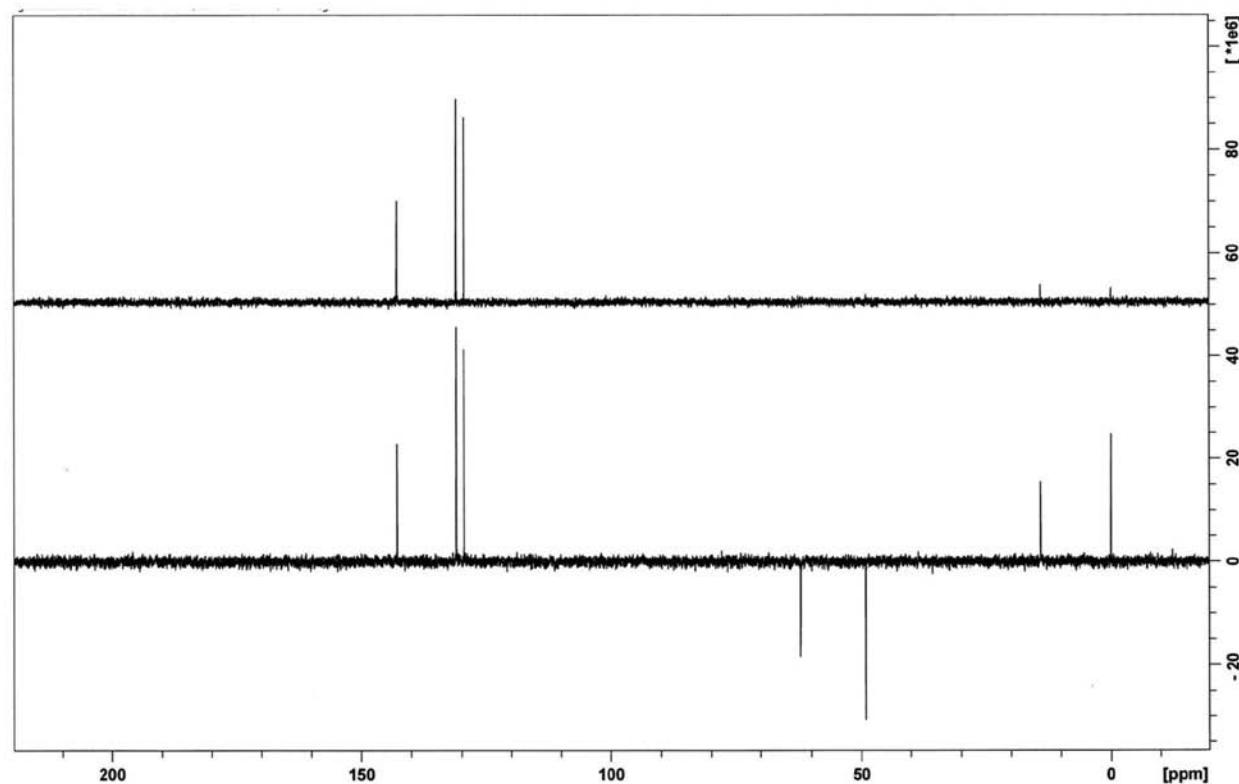
**Figure S13.** DEPT-90 and DEPT-135 spectra (CDCl<sub>3</sub>, 62.5 MHz) of ethyl (E)-2-chloroacetyl-3-(4'-chlorophenyl)propenoate (**E-3b**).
