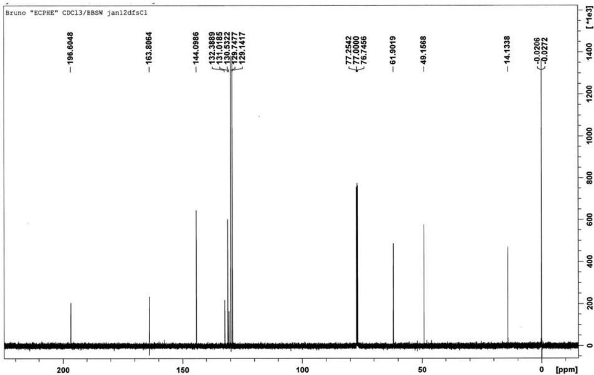
**Figure S2.**  $^{13}\text{C}$  NMR spectrum (CDCl<sub>3</sub>, 125 MHz) of ethyl (E)-2-chloroacetyl-3-phenylpropenoate (*E*-3a).
