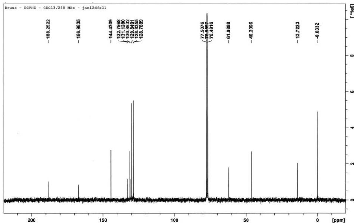
**Figure S7.**  $^{13}\text{C}$  NMR spectrum ( $\text{CDCl}_3$ , 62.5 MHz) of ethyl (Z)-2-chloroacetyl-3-phenylpropenoate (**Z-3a**).
