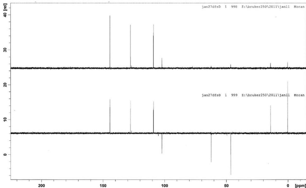
**Figure S38.** DEPT-90 and DEPT-135 spectra ( $\text{CDCl}_3$ , 125 MHz) of ethyl (Z)-2-chloroacetyl-3-(3',4'-methylenedioxyphenyl)propenoate (Z-3d).
