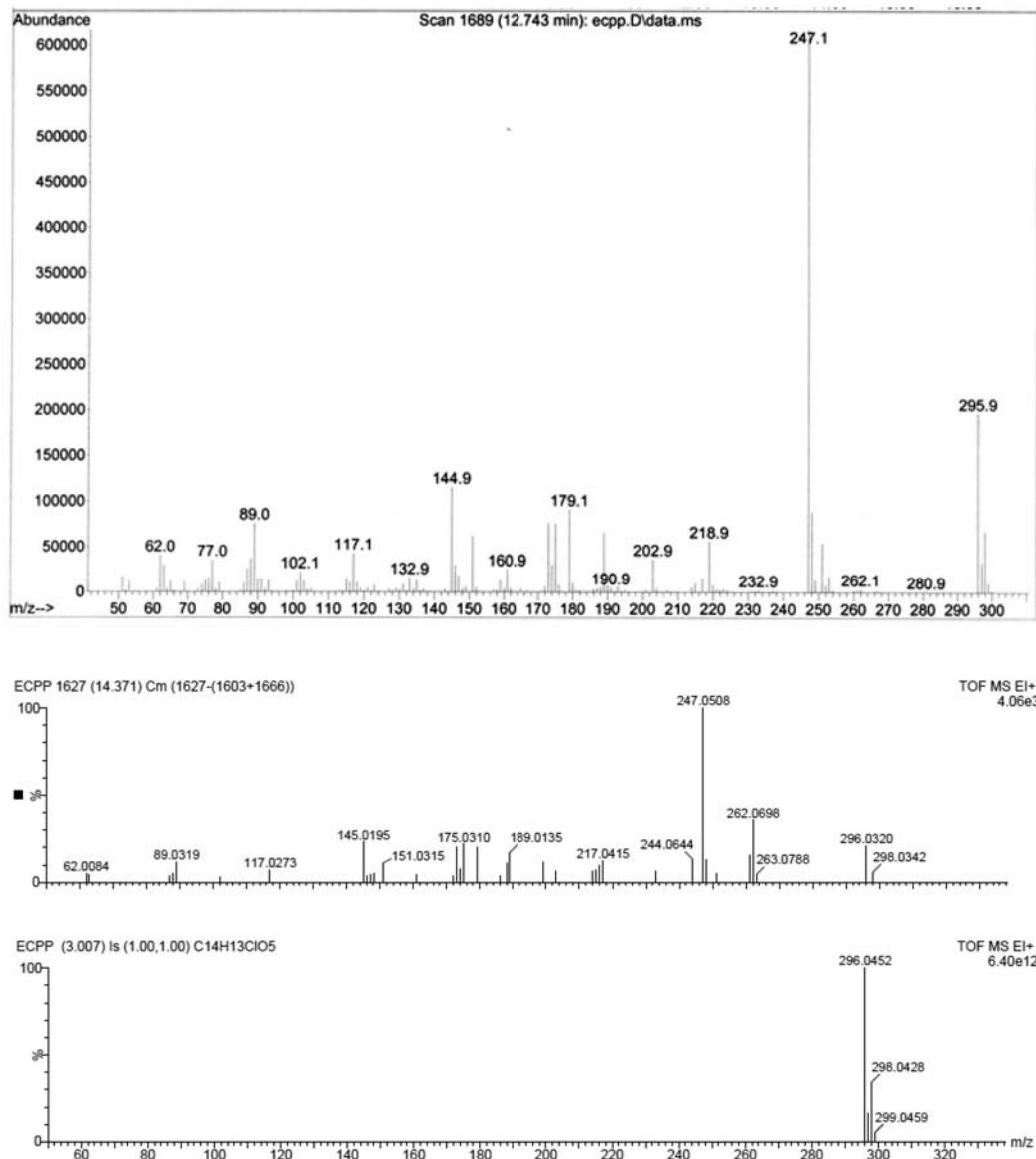
**Figure S35.** MS and HRMS (EI) spectra of ethyl (*E*)-2-chloroacetyl-3-(3',4'-methylenedioxyphenyl)propenoate (*E*-3d).
