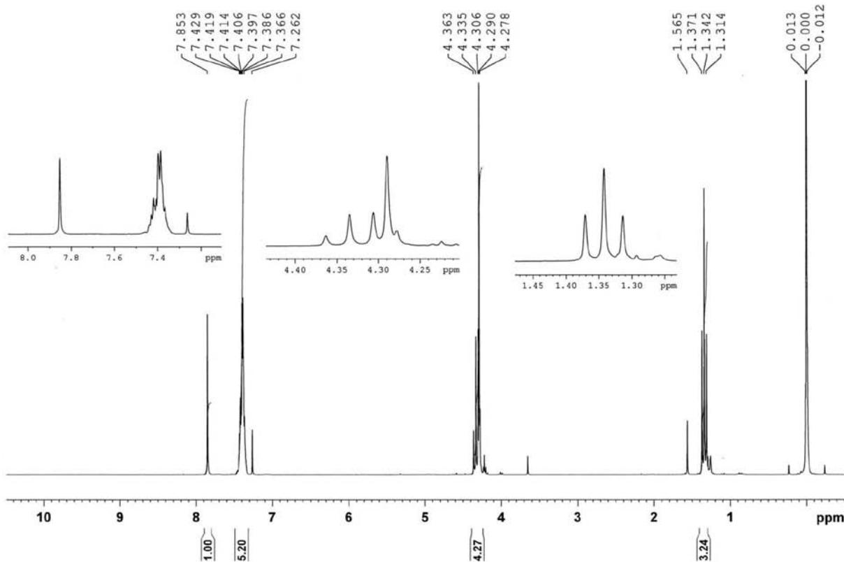
**Figure S1.**  $^1\text{H}$  NMR spectrum (CDCl<sub>3</sub>, 250 MHz) of ethyl (E)-2-chloroacetyl-3-phenylpropenoate (*E*-3a).
