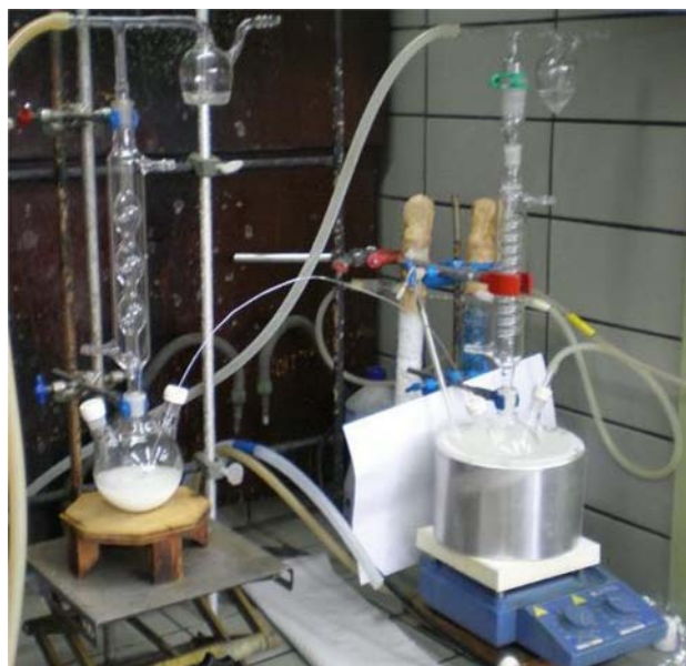
Figure S18. Addition of the cyclopentanecarboxylic acid dianion solution (left) to oxygen-saturated THF (right) in the preparation of 1-carboxy-1-hydroperoxycyclopentane ( 9 ).
