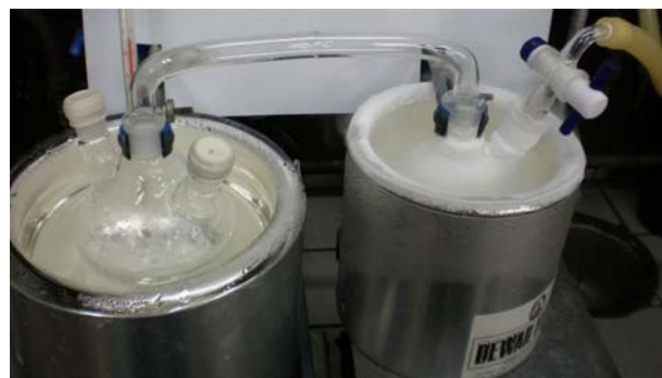
Figure 22. Bulb-to-bulb distillation of spiro -cyclopentyl-1,2-dioxetanone ( 6 ) in \text{CH}_2\text{Cl}_2 , from the reaction flask at -30\text{ }^\circ\text{C} (left) to the collection flask at -198\text{ }^\circ\text{C} (right).
