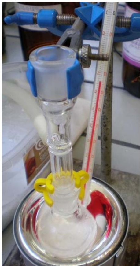
Figure S20. Crystallization of 1-carboxy-1-hydroperoxycyclopentane ( 9 ) from pentane at -25^{\circ}\text{C} .
