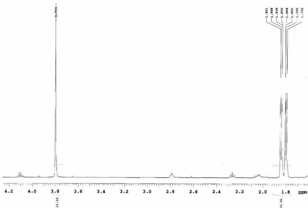
**Figure S4.** <sup>1</sup>H NMR spectrum (CDCl<sub>3</sub>, 500 MHz,  $\delta_{\text{H}}$  4.2–1.6) of the compound **1**.
