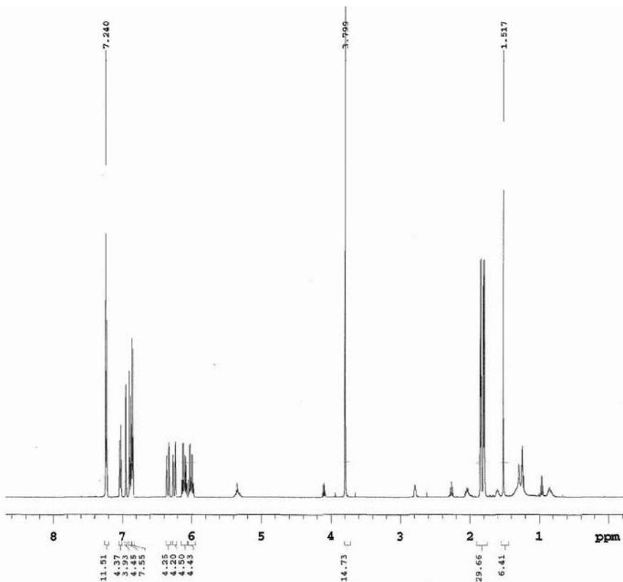
**Figure S2.**  $^1\text{H}$  NMR spectrum ( $\text{CDCl}_3$ , 500 MHz) of the compound 1.
