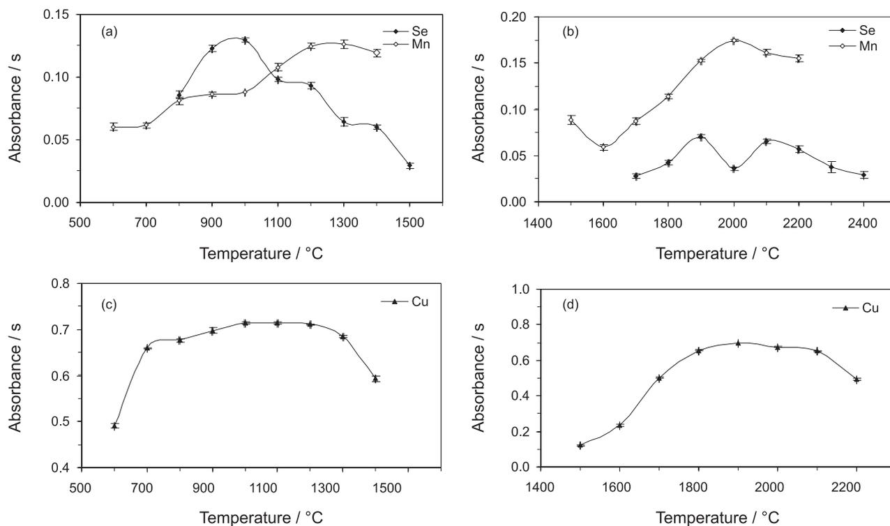
**Figure 1.** Optimization of experimental conditions for the GF AAS determination of Se, Mn and Cu in bovine semen samples: (a) pyrolysis curves for Se and Mn, (b) atomization curves for Se and Mn, (c) pyrolysis curve for Cu and (d) atomization curve for Cu. Injection of 20  $\mu\text{L}$  of bovine semen diluted 1:10 in 0.5% v/v  $\text{HNO}_3$  and 10  $\mu\text{L}$  of chemical modifier (20  $\mu\text{g}$  palladium and 5  $\mu\text{g}$  magnesium nitrate).
