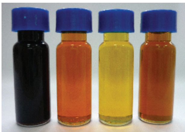
Figure 6. Photos of heavy oil (HO) and its hydrogenation products on sulfided catalysts.
