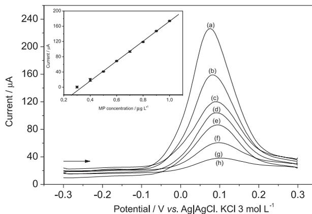
**Figure 8.** SWV optimized responses for different MP concentrations: (a)  $263.3$  (b)  $237.0$  (c)  $210.7$  (d)  $184.3$  (e)  $158.0$  (f)  $131.7$  (g)  $105.3$  (h)  $79.0 \mu\text{mol L}^{-1}$  in supporting electrolyte  $0.20 \text{ mol L}^{-1}$  acetate buffer pH 5.2 and volume of graphite suspension as a modifier of  $10 \mu\text{L}$ . Inset: calibration curve for MP.
