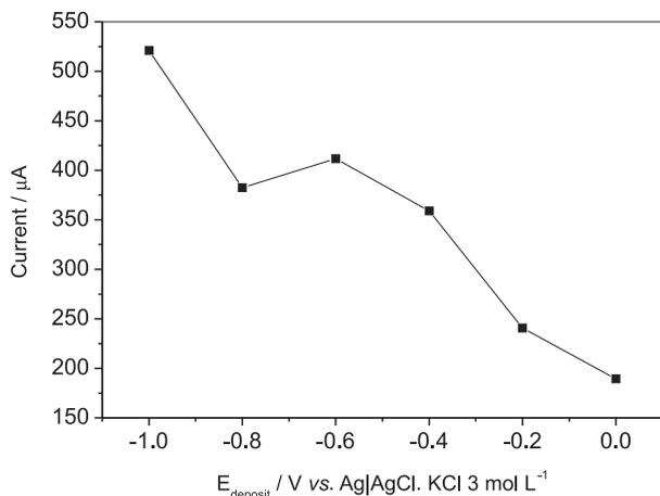
**Figure 7.** Relationship between accumulation potential ( $E_{\text{deposit}}$ ) for the  $3.0 \text{ mmol L}^{-1}$  MP oxidation peak current in supporting electrolyte  $0.20 \text{ mol L}^{-1}$  acetate buffer pH 5.2. SWV conditions: as described in Figure 6.
