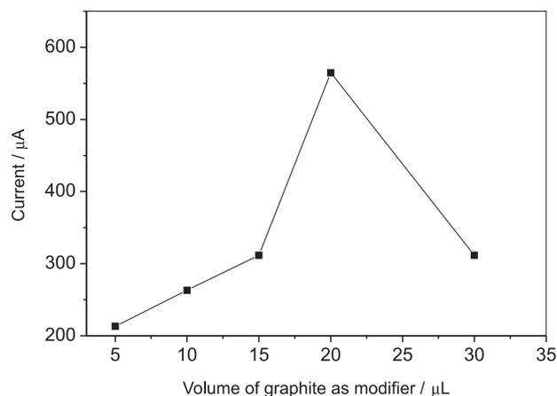
**Figure 6.** Influence effect of the amount of graphite dispersed in deionized water with the optimized SWV parameters on the 3.0 mmol L<sup>-1</sup> MP in supporting electrolyte 0.20 mol L<sup>-1</sup> acetate buffer pH 5.2. SWV conditions: scanning potential range -0.30 to + 0.30 V; frequency 50 Hz; potential increment (step potential) 1 mV; amplitude of the square-wave 100 mV.
