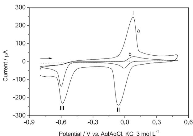
**Figure 2.** Cyclic voltammograms of  $5.0 \text{ mmol L}^{-1}$  MP on graphite-modified bppg (a) and bare bppg (b). Blank CV is shown as dot line. CV parameters: scan rate  $100 \text{ mV s}^{-1}$ ; supporting electrolyte  $0.20 \text{ mol L}^{-1}$  acetate buffer pH 5.2 and volume of graphite suspension as a modifier of  $10.0 \mu\text{L}$ .
