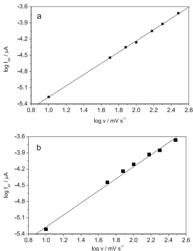
**Figure 5.** Dependence of the logarithm of peak current on logarithm of scan rate for oxidation (a: peak I) and reduction (b: peak II) of 3.0 mmol L<sup>-1</sup> MP.
