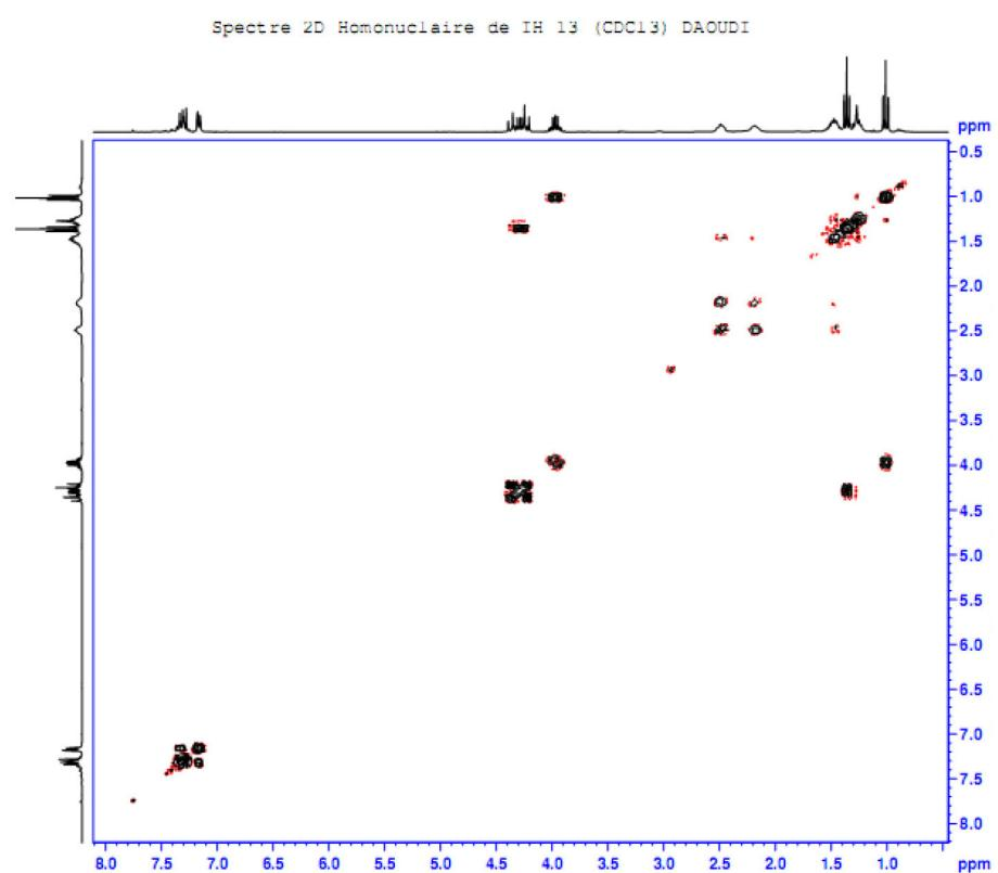
Figure S5. COSY of compound **6** in CDCl<sub>3</sub>.
