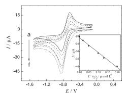
**Figure 5.** Cyclic voltammograms for **2**-CPE in 0.1 mol L<sup>-1</sup> B-R buffer solution, pH 6.1, containing (a-f) 0, 0.02, 0.05, 0.10, 0.13 and 0.20  $\mu$ mol L<sup>-1</sup> H<sub>2</sub>O<sub>2</sub>. Scan rate: 0.05 V s<sup>-1</sup>. Inset: cathodic peak current  $\nu$ s. H<sub>2</sub>O<sub>2</sub> concentration.
