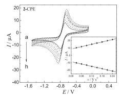
**Figure 4.** Cyclic voltammograms registered for **2-**CPE in 0.1 mol  $L^{-1}$  B-R buffer solution, pH 6.1. Curves (a-h) correspond to the scan rates 0.03, 0.06, 0.09, 0.12, 0.15, 0.18, 0.21 and 0.24 V s<sup>-1</sup>. Inset: peak current vs, the scan rate.
