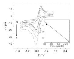
**Figure 6.** Cyclic voltammograms for **2**-CPE in 0.1 mol L<sup>-1</sup> B-R buffer solution, pH 6.1, containing (a-e) 0, 0.02, 0.05, 0.10 and 0.20 µmol L<sup>-1</sup> TCA. Scan rate: 0.05 V s<sup>-1</sup>. Inset: cathodic peak current *vs.* TCA concentration
